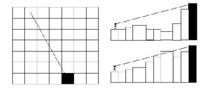
Figure 62. A visual schematic for line-of-sight calculation used in viewshed analysis. Each square column represents a cell in the digital elevation model, either visible or not visible from the observer point. From Wheatley (1995:12).
