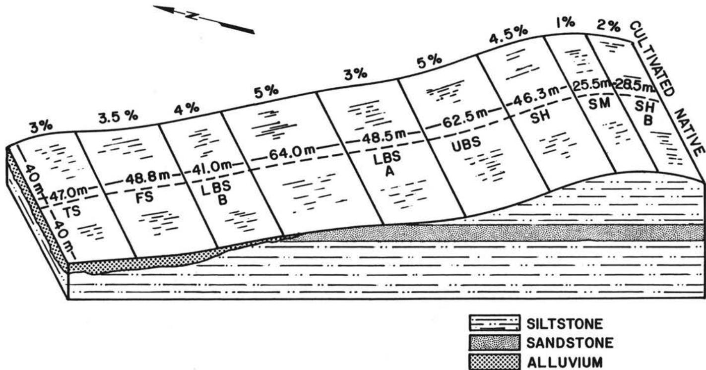
Figure 2.3 - Diagrammatic representation of the siltstone catena. Native and cultivated segments at this site include: Back Shoulder - SH B, Summit - SM, Shoulder - SH, Upper Backslope - UBS, Lower Backslope (A) - LBS A, Lower Backslope (B) - LBS B, Footslope - FS, Toeslope - TS. Slope lengths and gradients are indicated for each segment.
