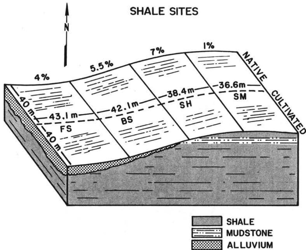
Figure 2.5 - Diagrammatic representation of the shale catena. Native and cultivated segments at this site include: Summit - SM, Shoulder - SH, Backslope - BS, Footslope - FS. Slope lengths and gradients are indicated for each segment.
