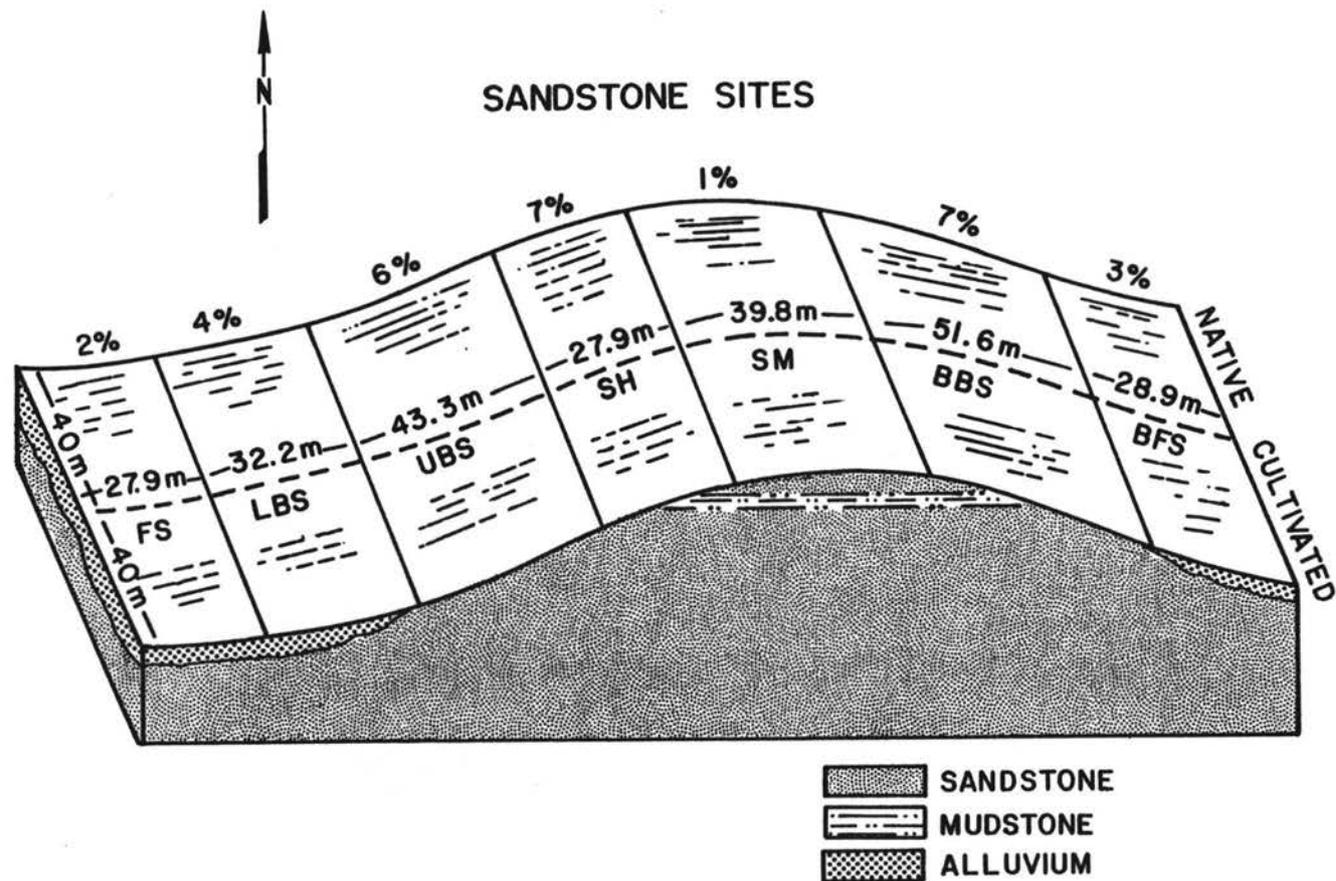
Figure 2.4 - Diagrammatic representation of the sandstone catena. Native and cultivated segments at this site include: Summit - SM, Shoulder - SH, Upper Backslope - UBS, Lower Backslope - LBS, Footslope - FS, Back Backslope - BBS, Back Footslope - BFS. Slope lengths and gradients are indicated for each segment.
