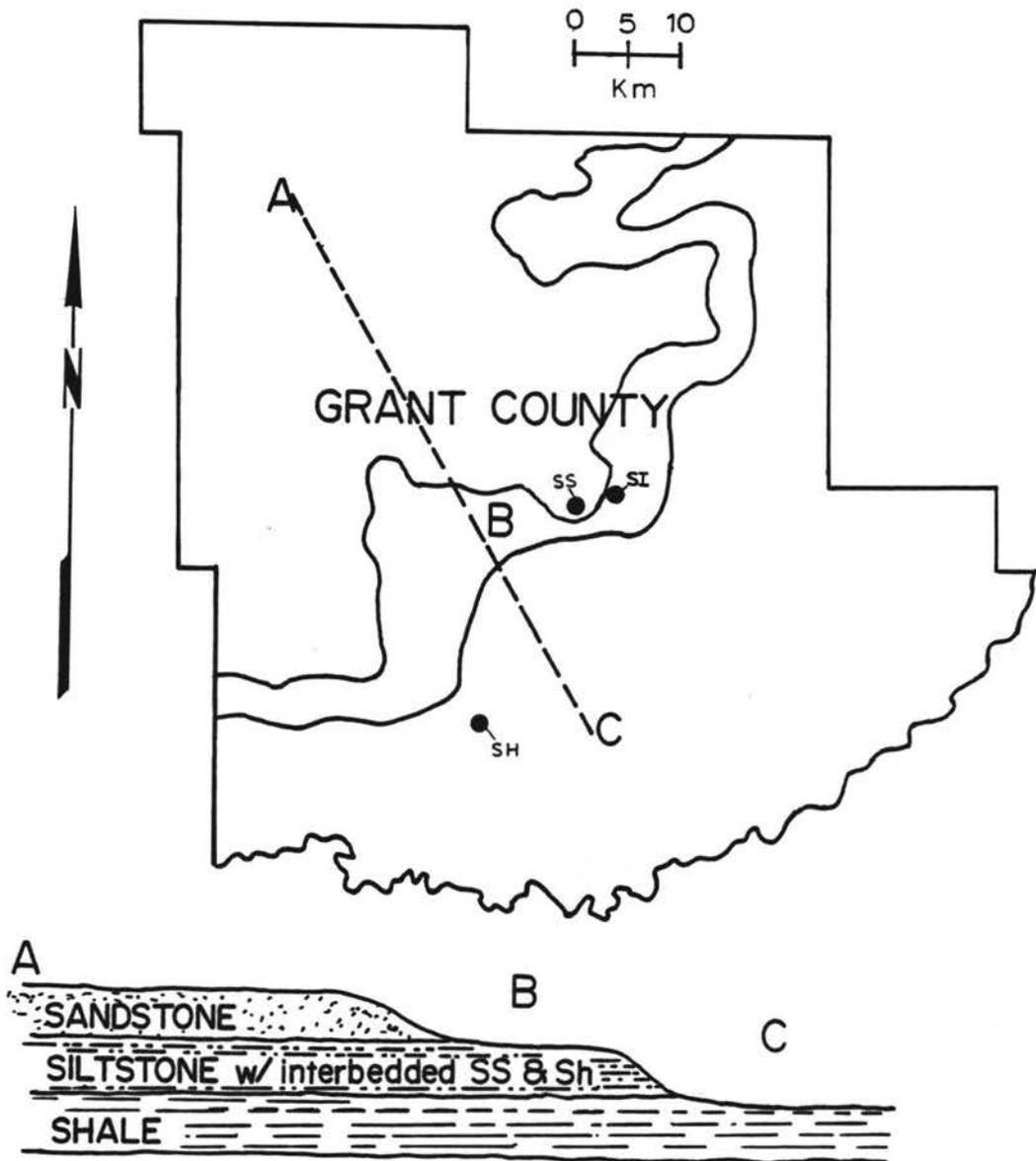
Figure 2.2 - Bedrock geology of Grant County, North Dakota. The locations of the three study sites are indicated on the diagram. (Sandstone - SS, Siltstone - SI, and Shale - SH)
