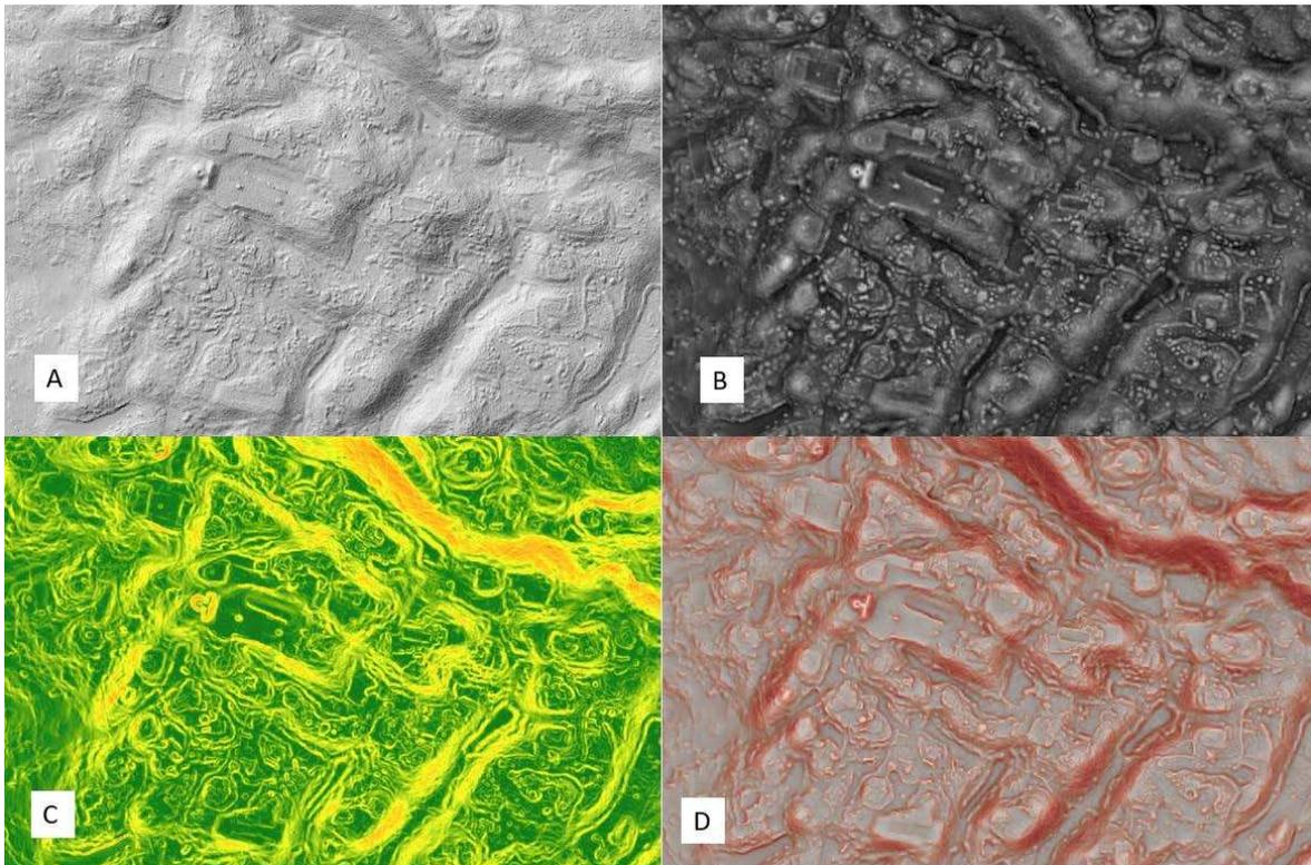
Figure 5. 5: LiDAR visualization techniques. a) standard hillshade, b) I factor, c) slope, d) pseudo RRIM
