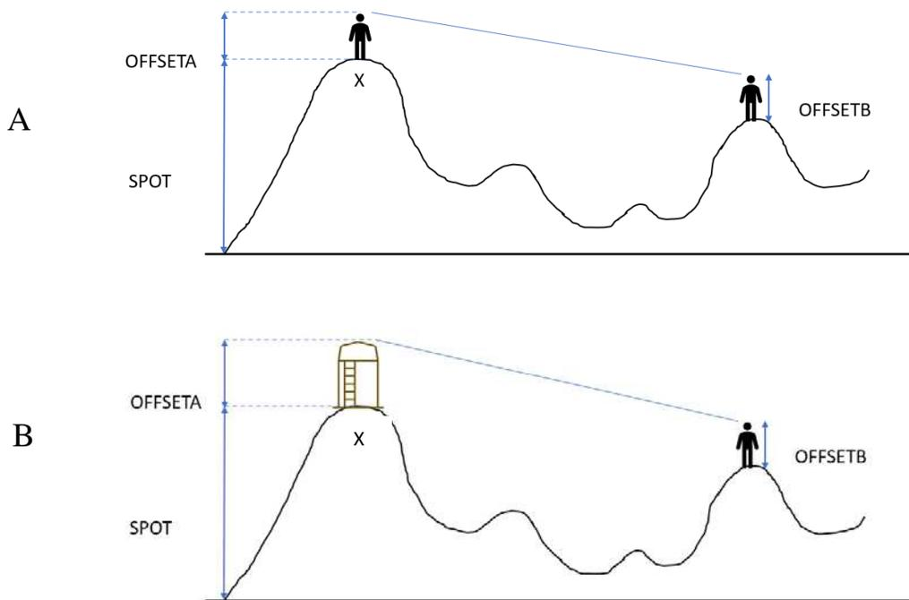
Figure 5. 2: Main observer parameters for visibility analysis in ArcGIS Pro. (a) assessing visibility of an observer at location X. (b) assessing visibility of a tower.
