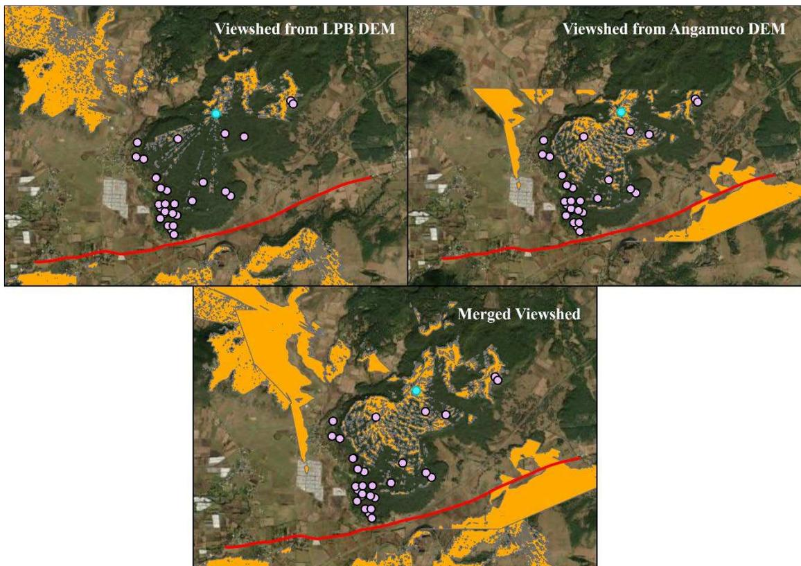
Figure 5. 27: Viewsheds for point AJ75-Py-1. (Top left) viewshed generated using the 2.5 m DEM for the LPB. (Top right) viewshed generated using the 0.5 m DEM for Angamuco. (Bottom) both viewsheds merged together into a single polygon feature class.
