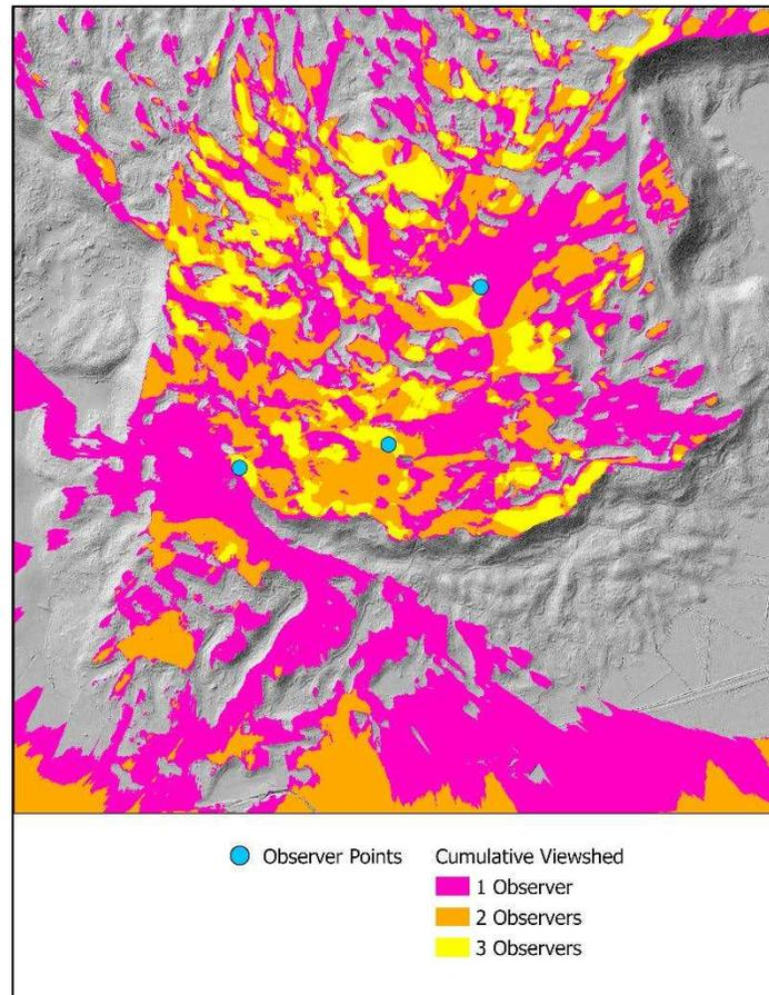
Figure 5. 3: Example cumulative viewshed surface displayed over a shaded relief. Each cell is coded with a value that represents the number of observer points that can see it/number of observer points it can see. Transparent areas do not have a line of sight to any observer points.
