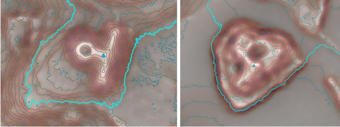
Figure 5. 18: Examples of 0.4 m contours generated for two pyramids (left) main yácata AN73-Py-1 and (right) yácata AC75-Py-1. The highlighted contours are the one's chosen as the base surface height.
