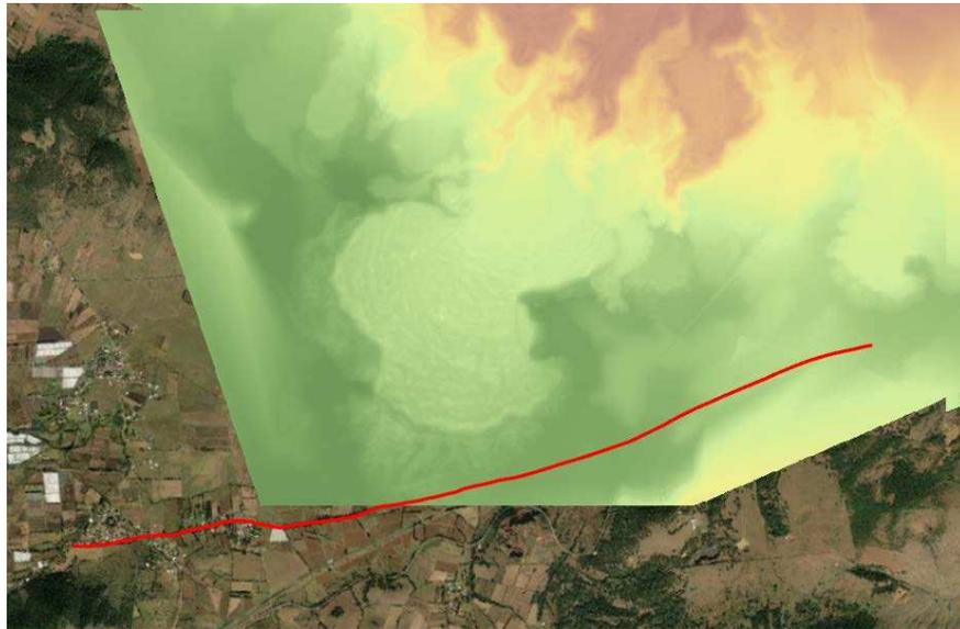
Figure 5. 26: Digitized portion of main southern road is shown as a red line. This is overlain on the Angamuco 0.5 m DEM. Note that the DEM extent does not cover the full length of the road segment.
