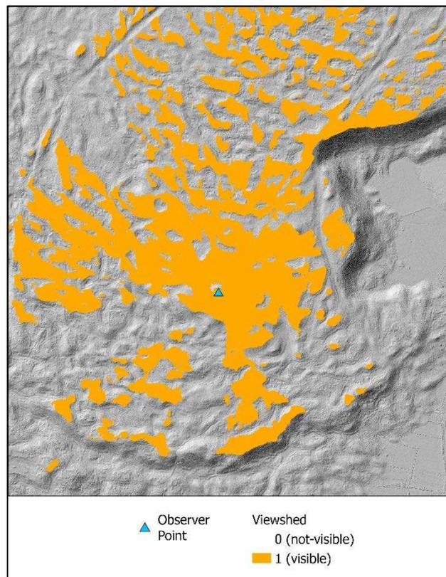
Figure 5. 1: Example of a simple viewshed with one observer point. All cells in orange have a value of 1, meaning they are visible to the observer/they can see the observer point. All cells with a value of 0 (turned transparent in this example) are not visible and cannot see the observer point. Viewshed is displayed over a shaded relief.
