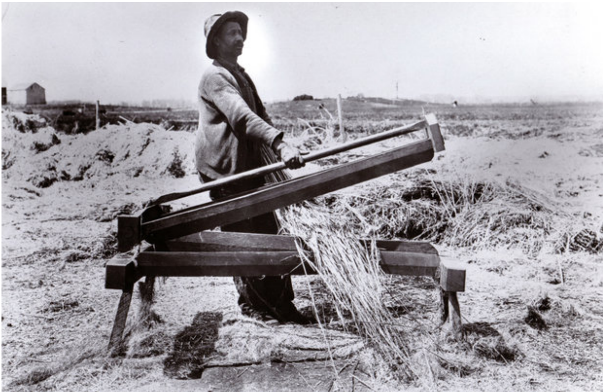
Figure 2.4. A hemp brake in operation in Kentucky circa 1920. A single person could operate a brake. Breaking typically took place from January to March each year (Hurt 1992:110). (Courtesy of the Kentucky Historical Society.)
