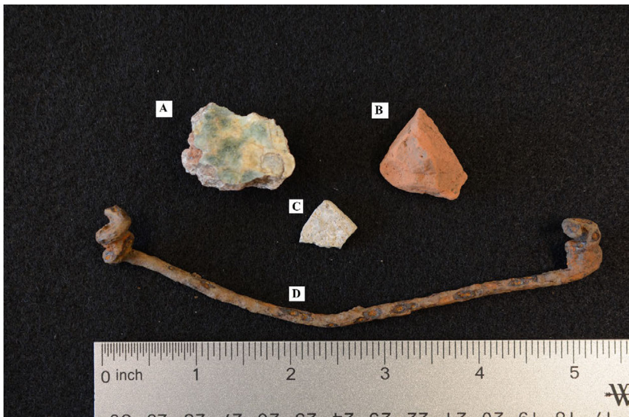
Figure 3.24. Construction material. (Upper) Numbers and percentages of construction-related material and (Lower) examples of (A) lime mortar with vitrification on one surface, (B) molded brick, (C) plaster; and (D) a segment of woven wire fencing (lower).
