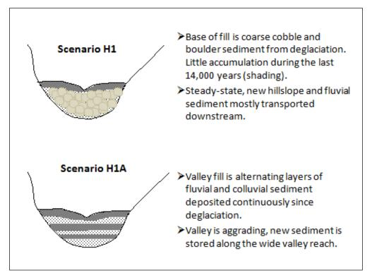
Figure 3.1. Scenario H1 represents a potential process of valley fill where a thin layer of fluvial and colluvial sediment is overlying a thick sequence of glacially derived coarse sediment. H1A would be identified by continuing aggradation in the 14,000 years since glacial retreat with several layers of alternating fine and coarse deposits.
