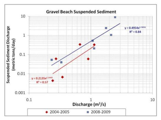
Figure 4.13. GB suspended sediment rating curve comparison of 2004-2005 with 2008-2009. Suspended sediment concentrations are higher in 2008-2009.
