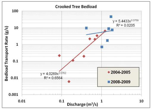
Figure 4.17. CT bedload sediment rating curve comparison of 2004-2005 with 2008-2009. There is no change in bedload transport.
