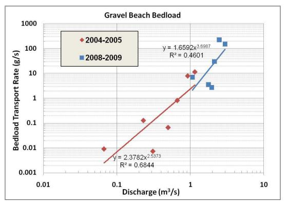
Figure 4.18. GB bedload sediment rating curve comparison of 2004-2005 with 2008-2009. There is no change in bedload transport.
