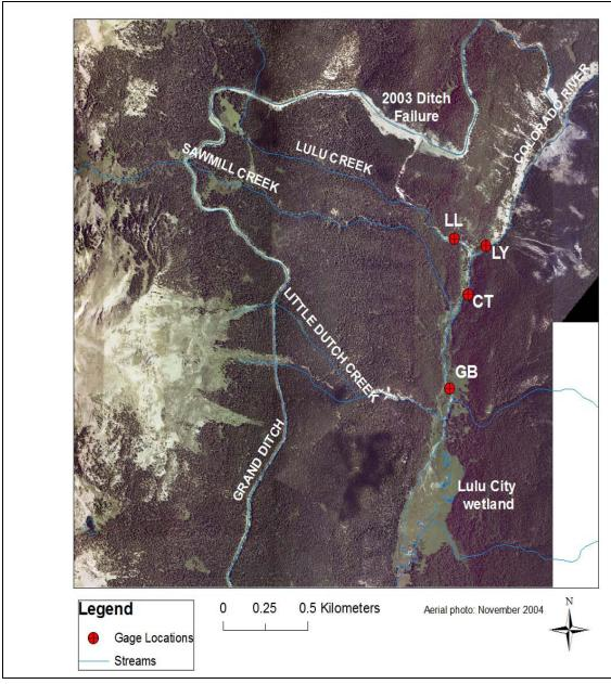
Figure 4.1. Four gages are located in the study area: LY is Colorado River at Little Yellowstone, CT is Colorado River at Crooked Tree, GB is Colorado River at Gravel Beach, LL is lower Lulu Creek. Flow on Colorado River is from upper portion of figure toward bottom. Grand Ditch flow is from the bottom of the figure to the top.
