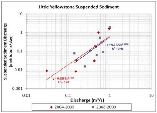
Figure 4.9. LY suspended sediment rating curve comparison of 2004-2005 with 2008-2009. LY is upstream and unaffected by the 2003 debris flow, and no temporal trend is apparent.
