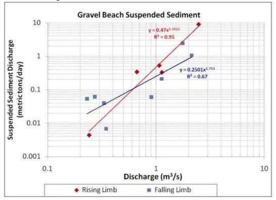
Figure 4.14. GB suspended sediment rating curve comparison of rising and falling limb flows. Data do not suggest hysteresis at low flows.
