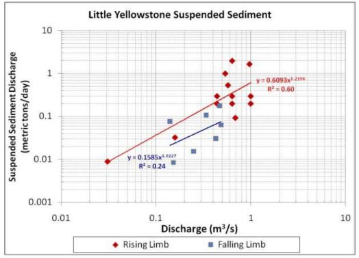
Figure 4.10. LY suspended sediment rating curve comparison of rising and falling limb flows. Data suggest clockwise hysteresis, which suggests depletion of fine sediment during the snowmelt period.
