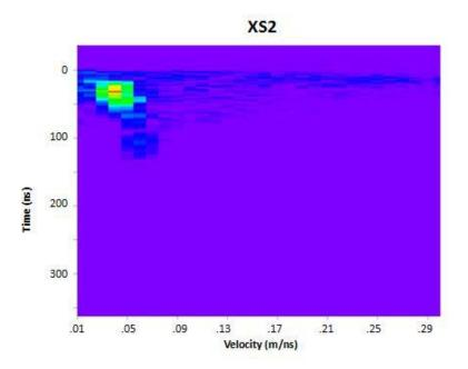
Figure 3.3. XS2 CMP survey velocities are indicated by warm colors over depth. Warm colors indicate electromagnetic propagation velocities and can be used to convert the time of radar return signals to depth in the GPR reflection surveys. In XS2 as well as XS4, a velocity of 0.05 m/ns was observed. The velocity of 0.05 m/ns was applied to all GPR transects to convert reflection time to depth.
