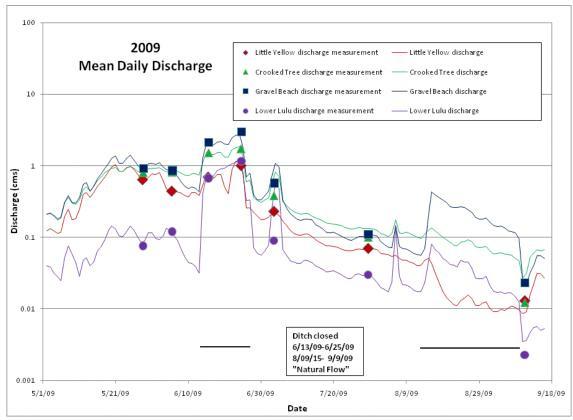
Figure 4.6. Mean daily discharge for 2009 from LY, CT, GB, and LL sites shows two periods where the Grand Ditch did not operate and flow was not diverted out of the Colorado River.
