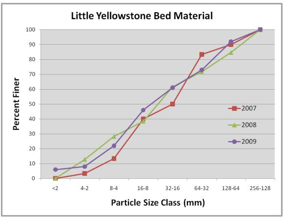
Figure 4.19. LY bed material size distribution 2007-2009. No change is detected during this period. LY was upstream of the 2003 debris flow and therefore not affected.
