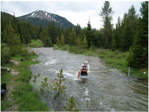
Figure 4.3. Discharge measurement taken at bankfull discharge at GB, June 24, 2009. View is looking downstream.
