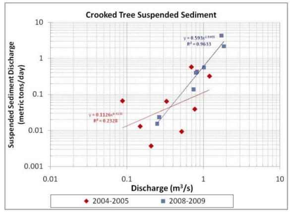
Figure 4.11. CT suspended sediment rating curve comparison of 2004-2005 with 2008-2009. Variability decreases in 2008-2009.
