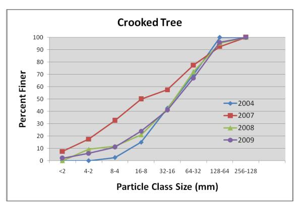
Figure 4.20. CT bed material size distribution 2004 and 2007-2009. Fining of the bed occurred in 2007, followed by coarsening in 2008 and no change in 2009.
