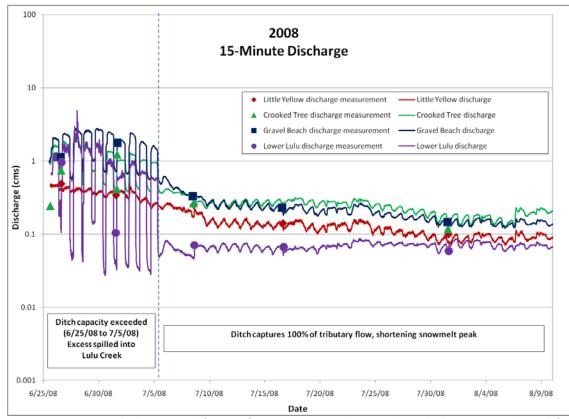
Figure 4.5. 15-minute discharge record for 2008 from LY, CT, GB, and LL sites shows discharges into Lulu Creek from the Grand Ditch. After July 5 no discharges from Grand Ditch occur.
