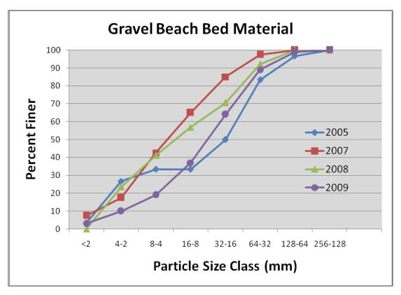
Figure 4.21. GB bed material size distribution 2005 and 2007-2009. Fining of the bed occurred in 2007, followed by coarsening in 2008 and 2009.
