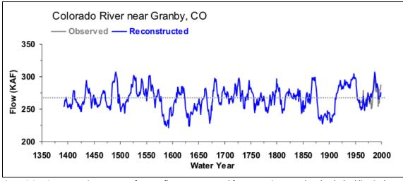
Figure 2.2. 10-year running average of streamflow reconstructed from tree-ring records. The dashed line is the mean annual flow of the period of record for the Granby gage (1951-1999). Image from www.treeflow.info/upco/coloradogranby.html
