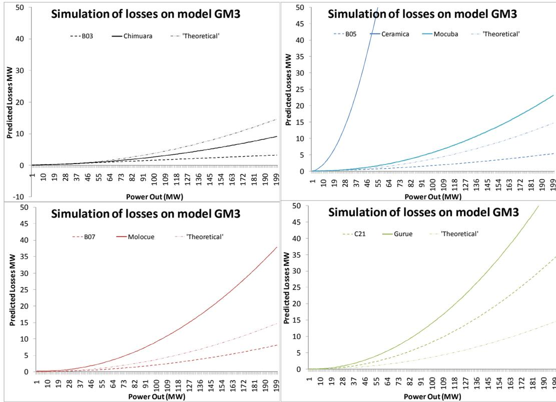
Figure V.23 - Comparison of  $I^2R$  losses regression-predicted for each system's component and the analytical (theoretical), for a summer day at peak hour
