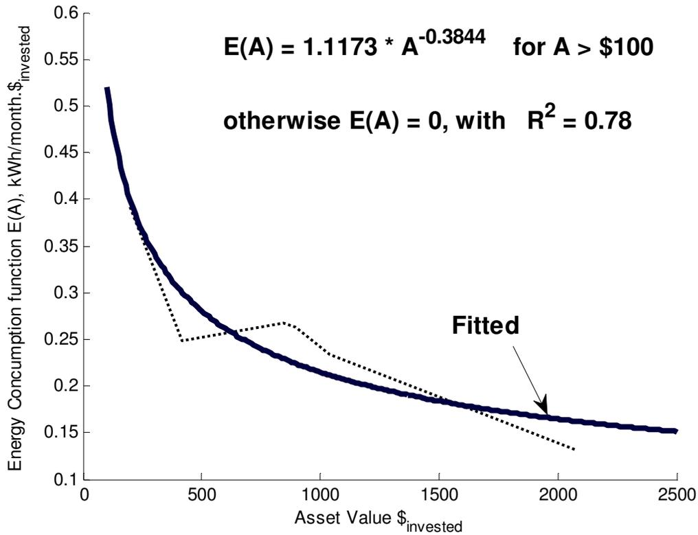
Figure VI.44 – Approximate function for electricity consumption
