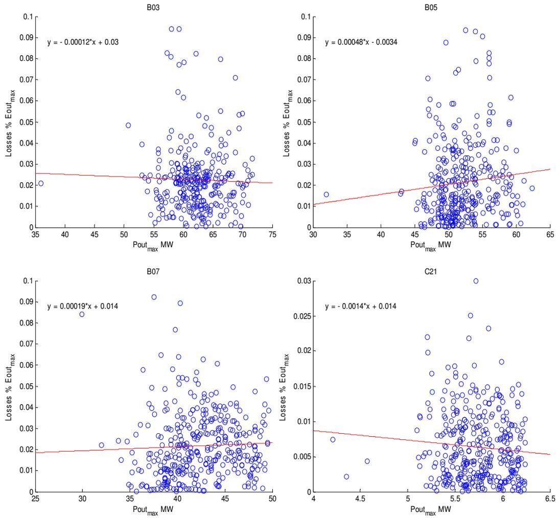
Figure V.28 – Daily Energy Losses recorded in the Transmission lines
