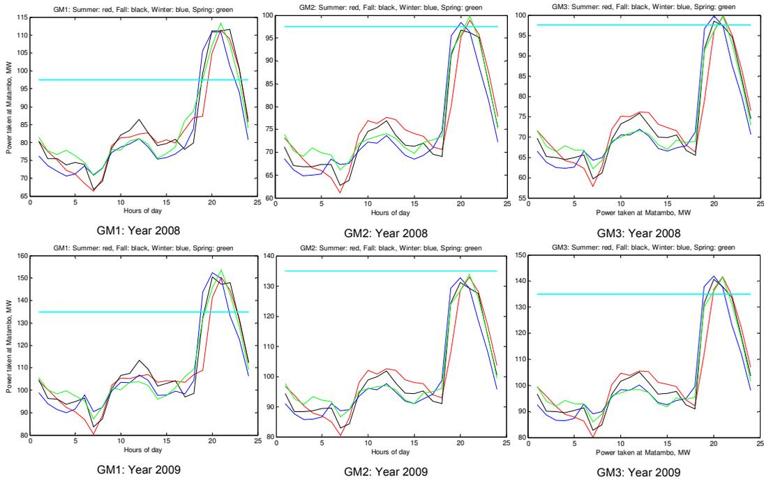
Figure V.32 – Forecast of the power taken at the Matambo based on PSS/E simulations
