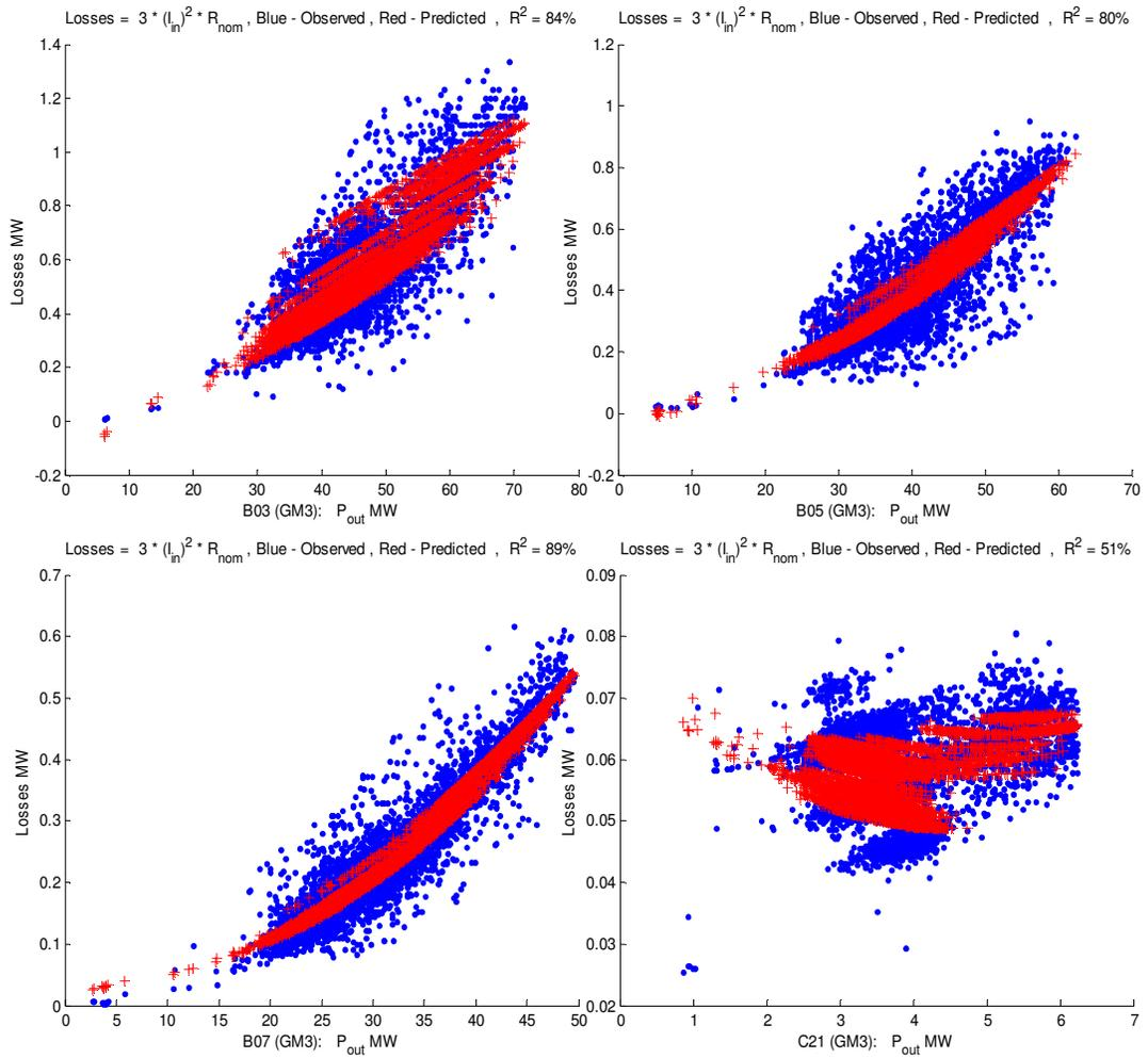
Figure V.21 -  $I^2R$  losses in MW observed and predicted in the system's transmission lines, as a function of  $P_{out}$  in MW
