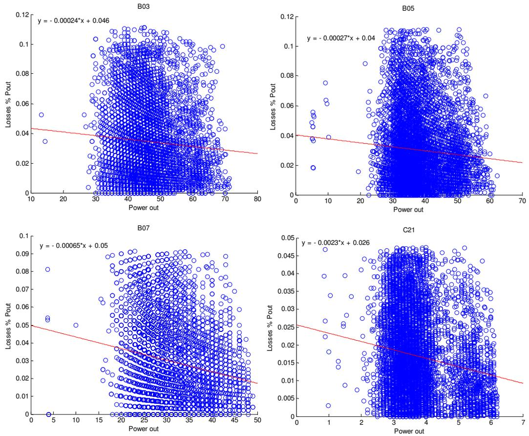
Figure V.30 – Hourly Energy Losses recorded for Transmission lines
