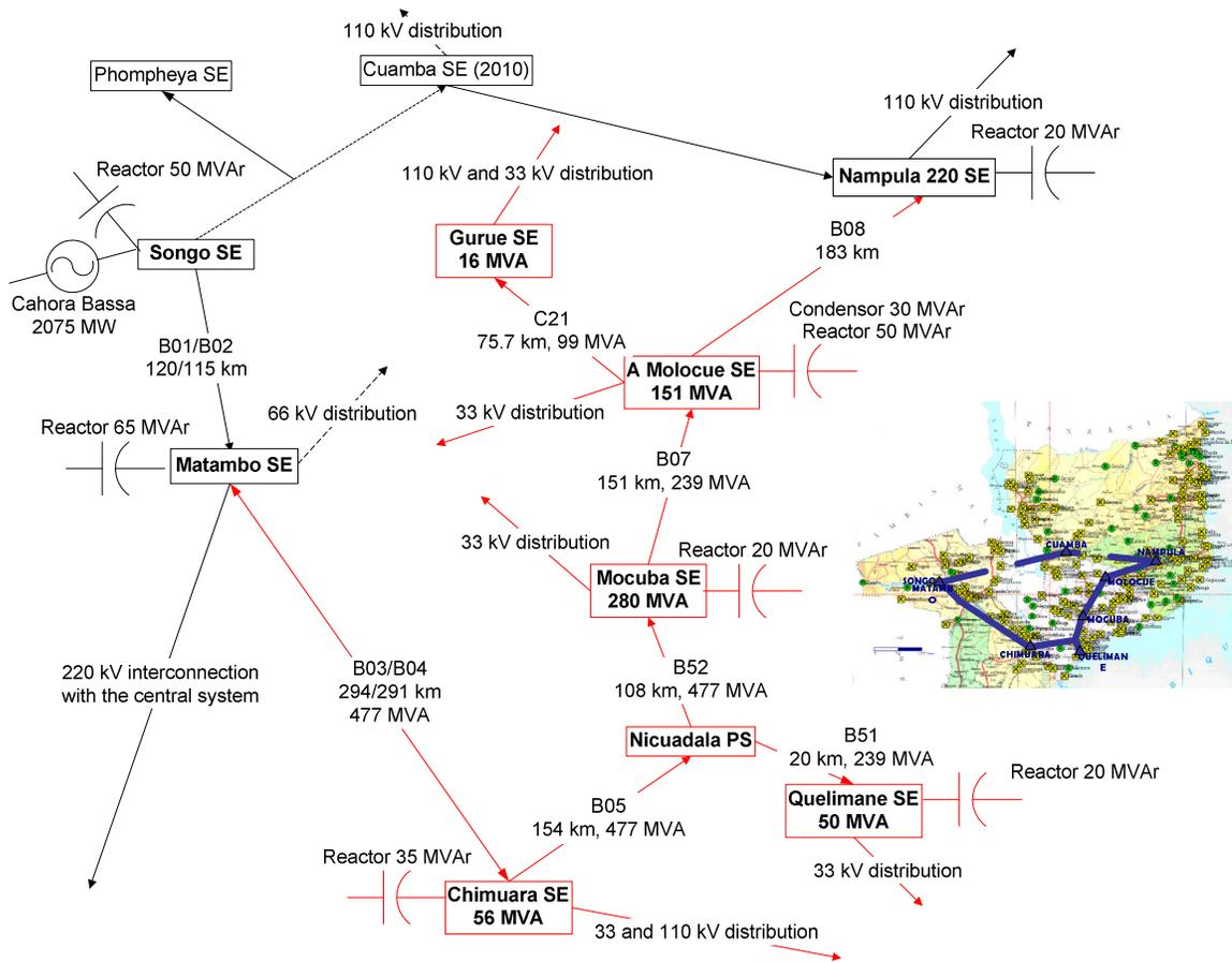
Figure I.5 – Schematic representation of the linha centro-norte (LCN)
