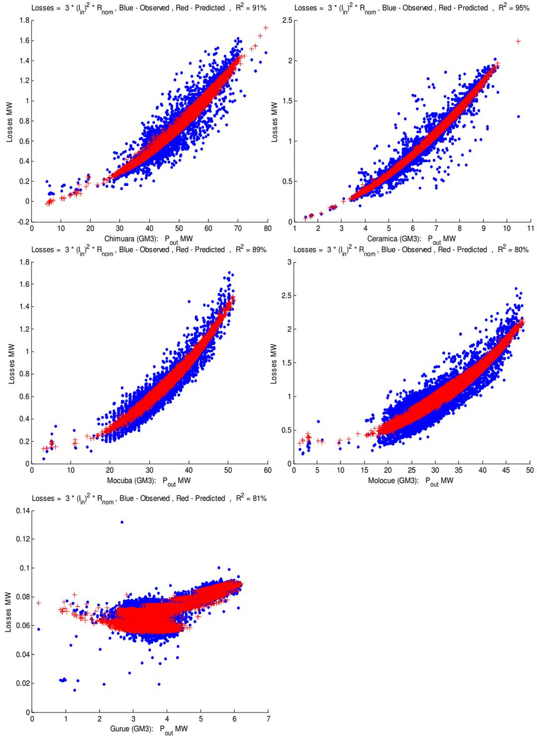
Figure V.22 -  $I^2R$  losses in MW observed and predicted in the system's substations, as a function of  $P_{out}$  in MW
