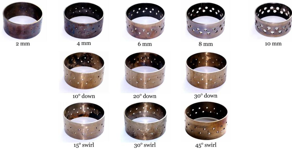
Figure 4.3: Photographs of the secondary air inlets tested in this study.
