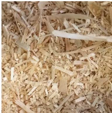
(a) Douglas fir chips used for Test Matrix 1
