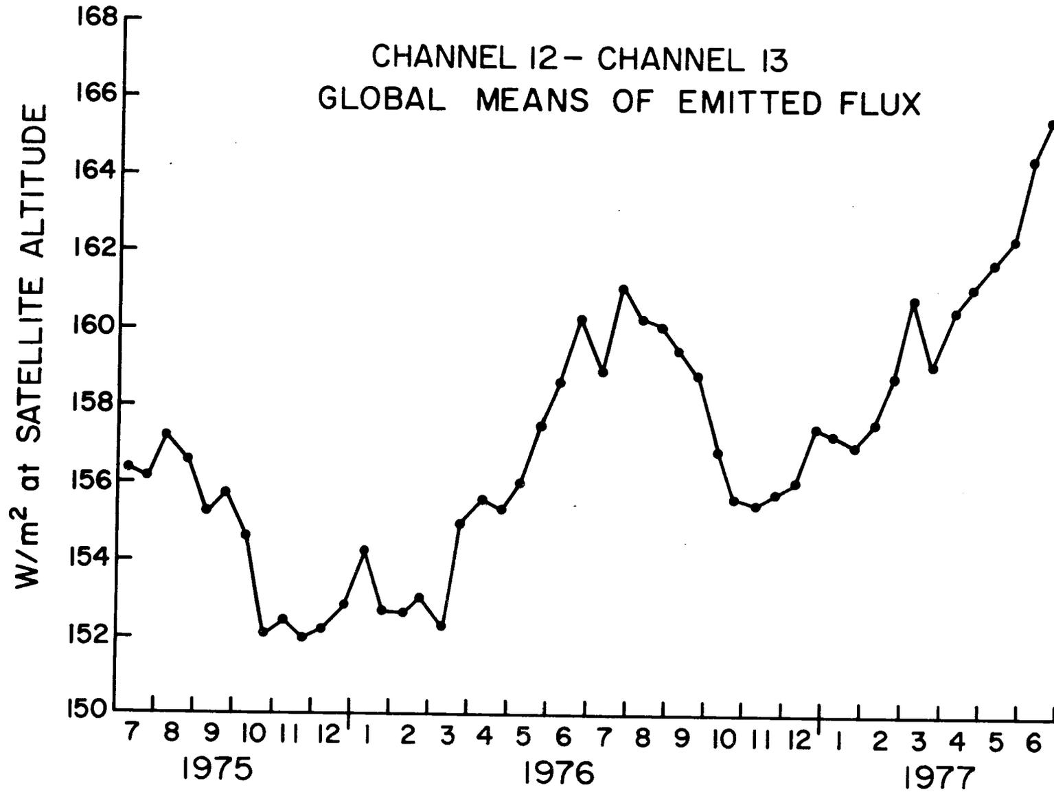
Fig. 5a. Time series of two week orbital means for two years. The trend in reflected and emitted was removed by fitting the first year observations to the second. This assumed a linear decline in transmission of the channel #13 filter produced the trend.
