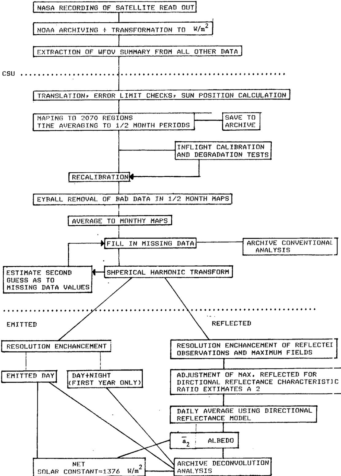
view (WFOV) integrating sensors to measure low resolution, 200 km, fluxes and the global integral budgets. We will discuss results from the WFOV detectors of the earth fluxes. Results from the other systems have been discussed elsewhere (Hickey et al., 1977; Jacobowitz et al., 1979). Perhaps the most interesting result is the stability of the solar constant with no variations detected to the instrument accuracy ( $\pm .5\%$ ) over 4 years (Hickey, 1980).
