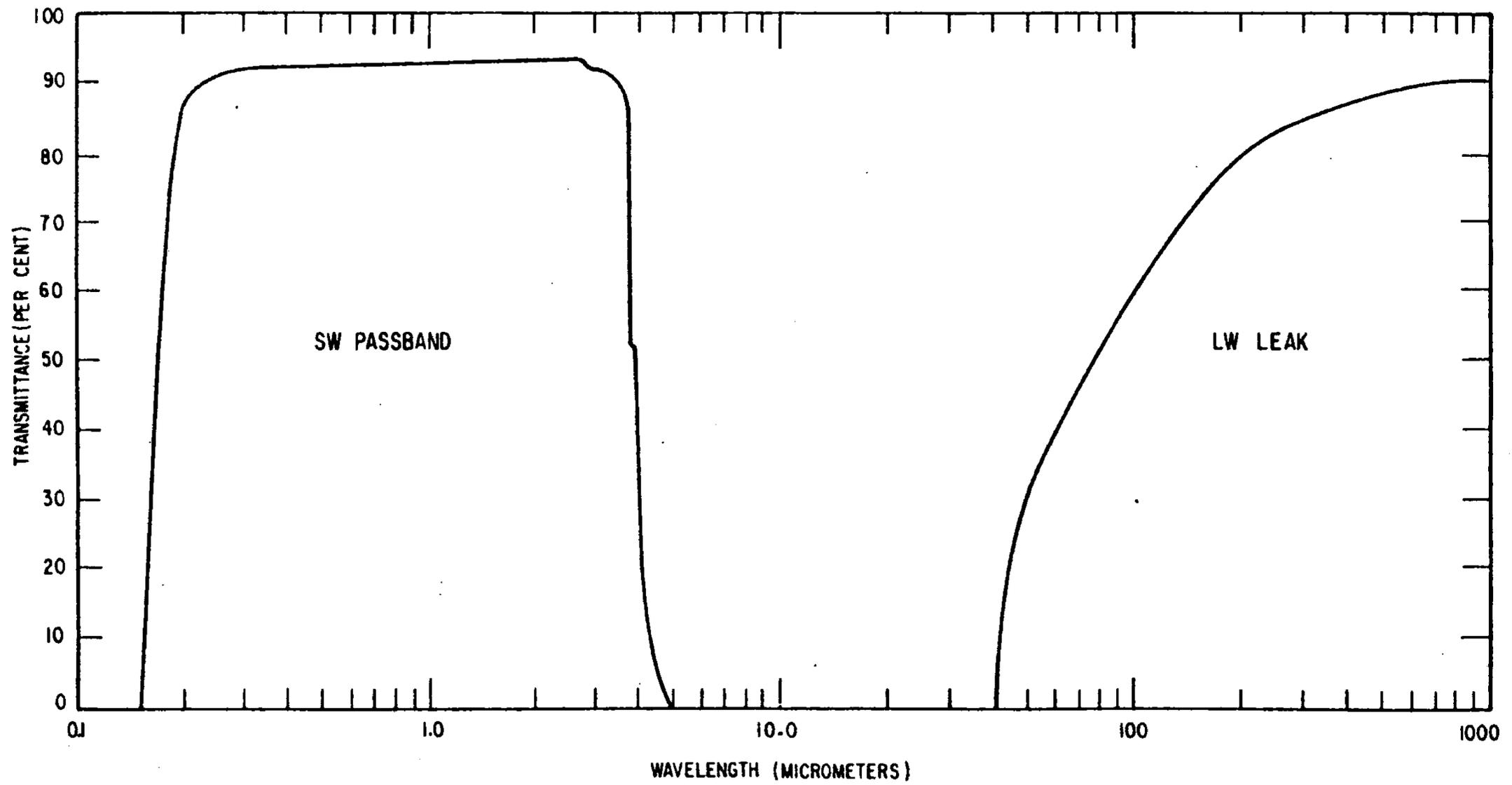
Fig. 2. Transmittance of Supersil W fused quartz filters, channel 13.
