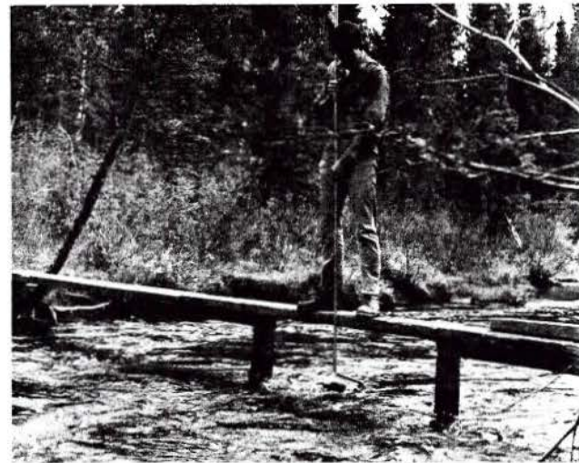
Figure 4-- Wintertime collection of bacteria sample (top) and summer sediment collection with "depth-integrating" sediment sampler (bottom).
