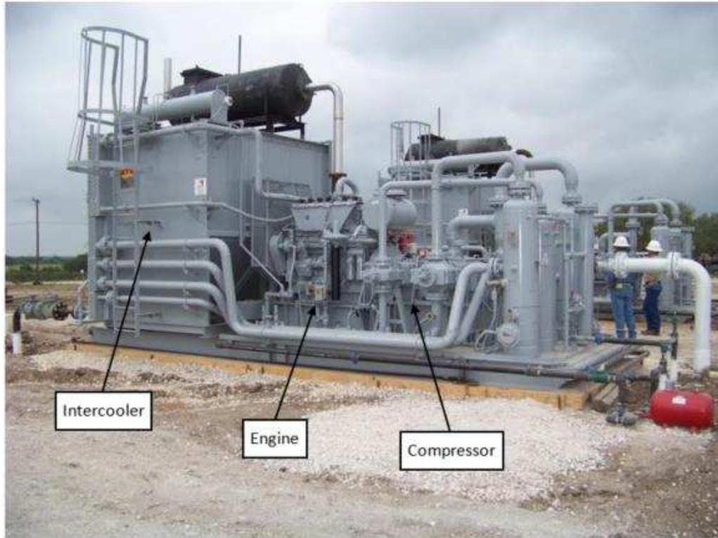
Figure 1: Cummins KTA19GC Natural Gas Compressor Engine at Well Site (Photo provided by Cummins, Inc)
