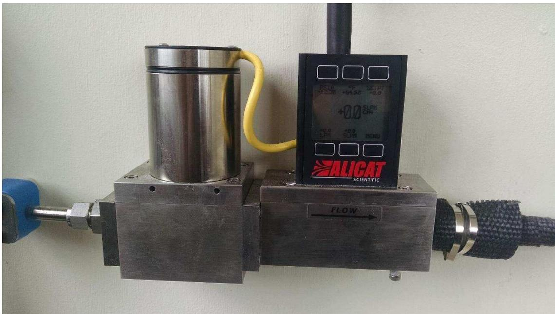
Figure 14: Alicat Scientific MC-Series Mass Flow Controller
