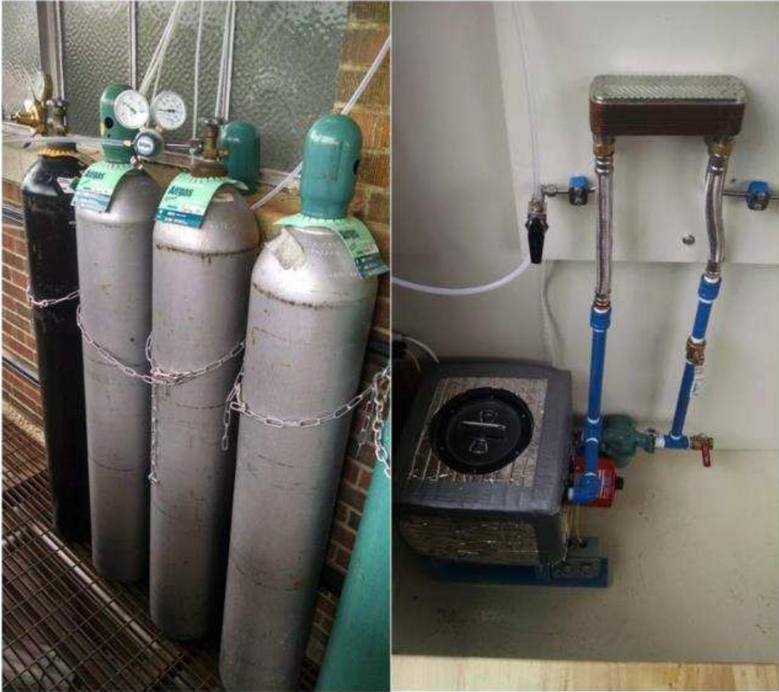
Figure 13: (Left) Gas Bottles and Pressure Regulator, (Right) Heat Exchanger and Water Recirculation System
