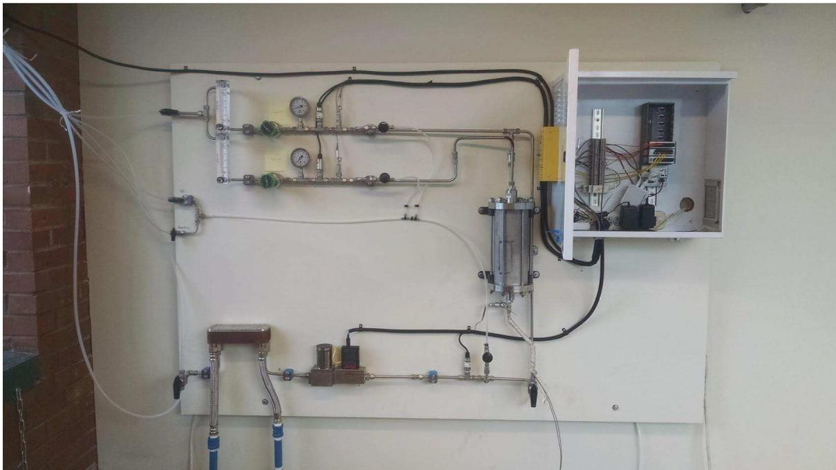
Figure 39: Membrane module testing setup
