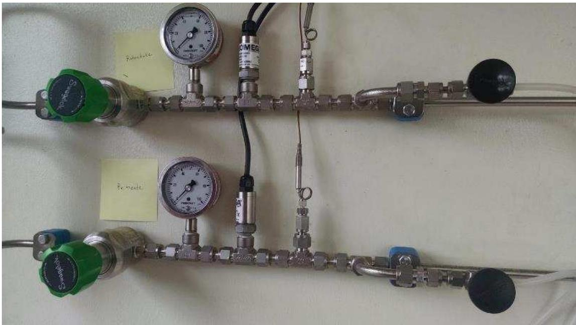
Figure 16: From left to right: Backpressure regulator, analog pressure gauge, pressure transducer, thermocouple, bleed valve
