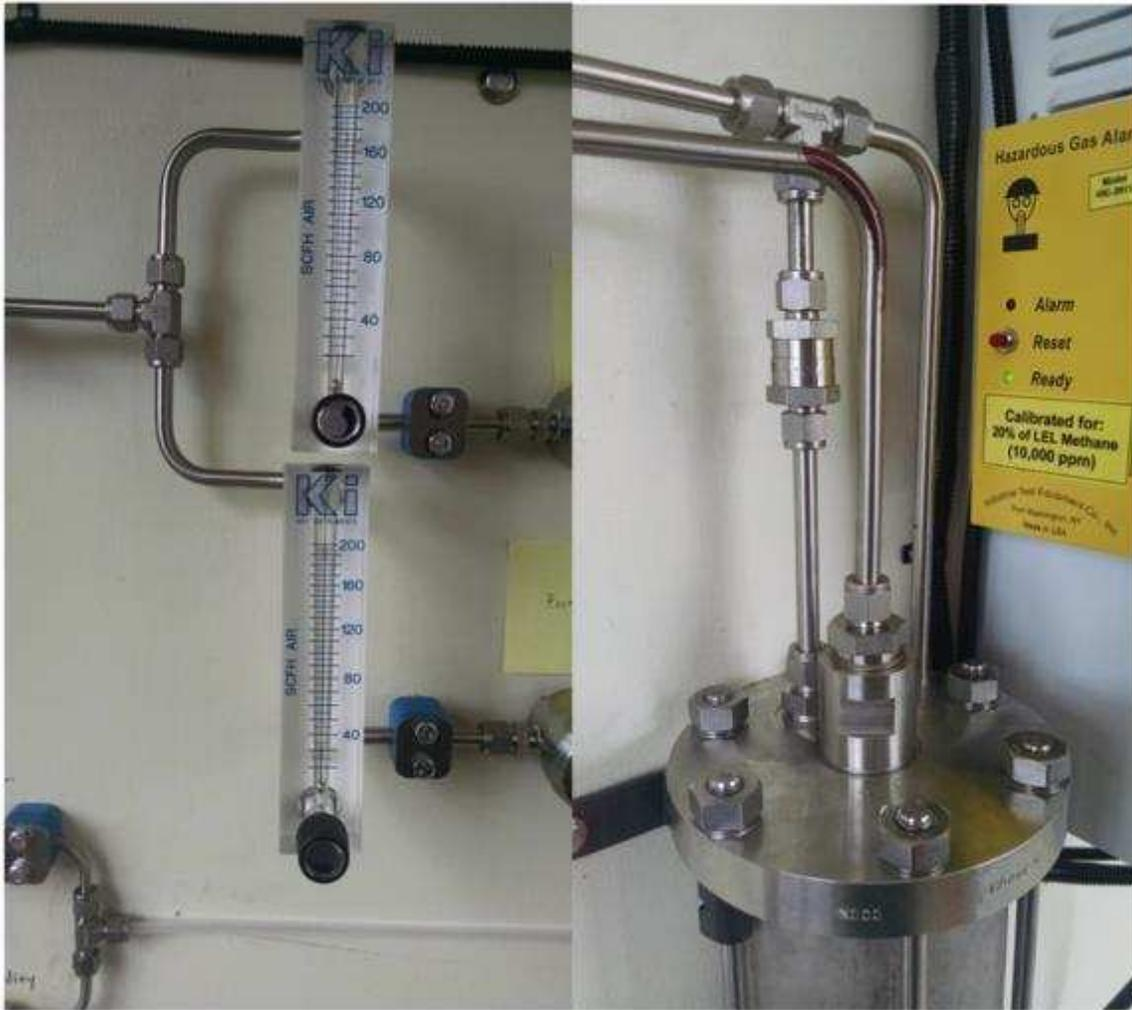
Figure 17: (Left) Brooks rotameters (Right) methane detector, retentate, and permeate ports on membrane module
