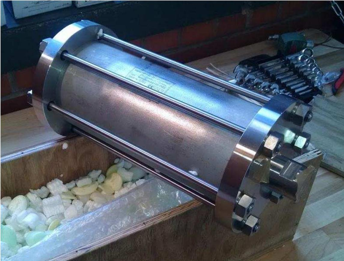
Figure 11: Plate and Frame Membrane Module
