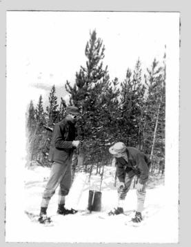
Figure Seven - Weighing a modified Weather Bureau gage to determine the amount of snowfall for the previous week. Average depth of the course is obtained by determining the arithmetic mean of the depths measured during the survey. The average depth is entered on standard forms.
