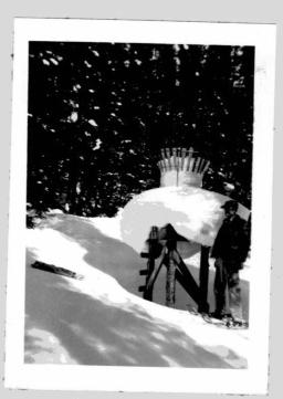
Figure Two - A Sacramento gage fitted with an Alter snow shield. This gage, at 10,000 feet elevation, is a source of data used in forecasting streamflow for the Colorado River.
