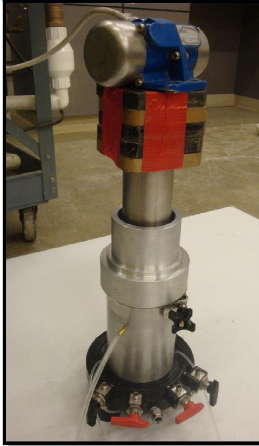
Figure 3.7 Set up of the equipments used to create dense specimen
