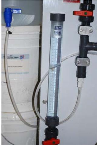
**Figure 6 - Pump Calibration Column**
