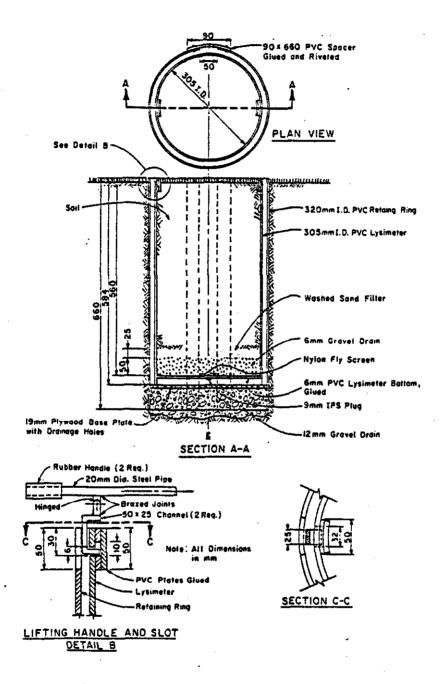
Figure 2.3 Construction details of the bucket lysimeter.
