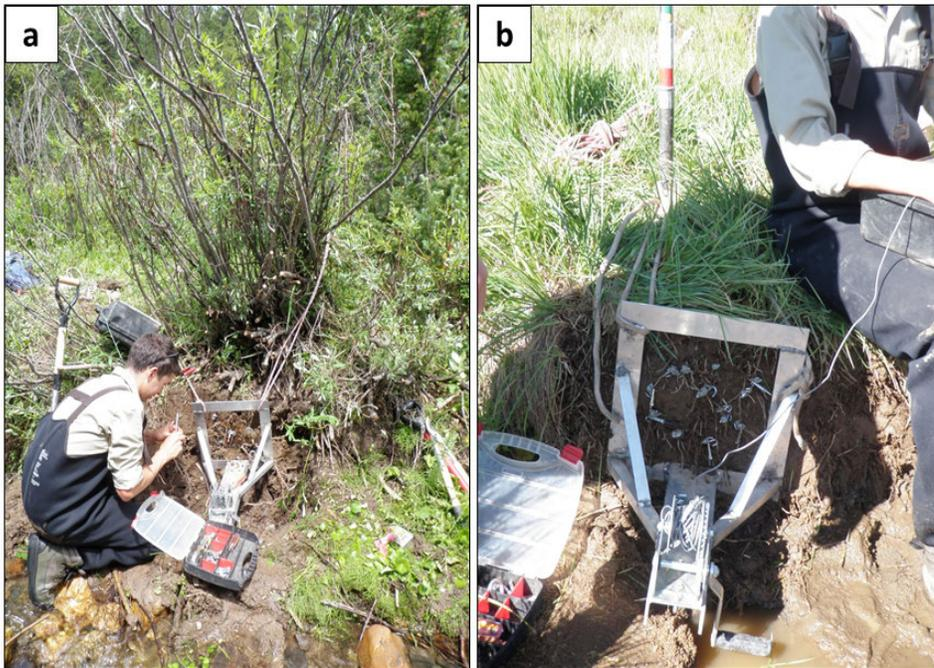
**Figure 20. Photographs showing Root Puller attached to low cutbanks. U-bolts are attached to roots before being pulled. (a) Below *S. monticola* specimen along N. Joe Wright Creek. (b) On a cleaned face below dense *C. aquatilis* patch along a side channel of Corral Creek.**
