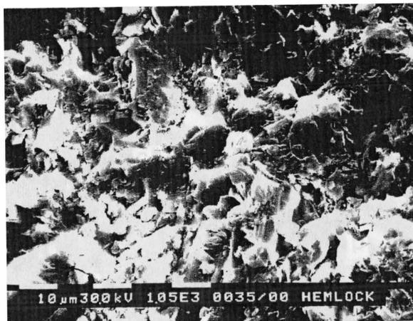
Fig. 30. SEM image of the spot analyzed in figure 30. The small, bright crystals in the lower left and center left may be calcite rhombohedrons.
