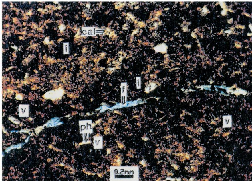
Fig. 48. Porosity created by a microfracture (f) passing through volcanic rock fragments and iron oxide cement. Sample 1-2393-15; plane light photomicrograph.
