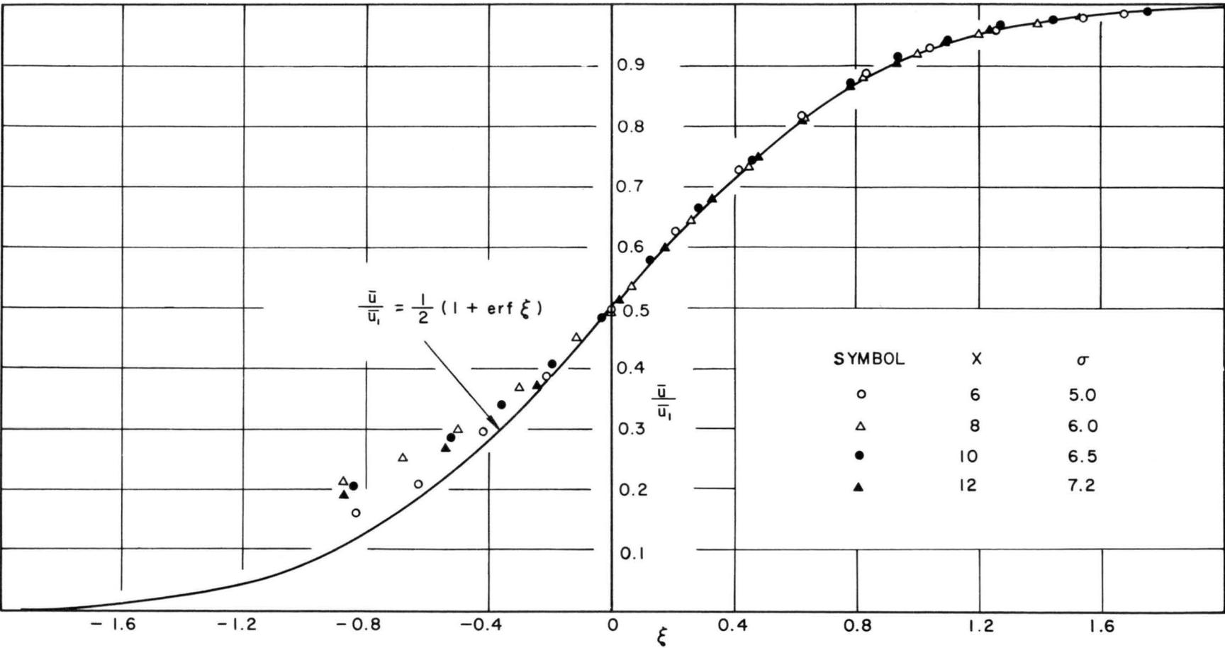
FIG. 23-1 COMPARISON OF THEORY AND VELOCITY MEASUREMENTS FOR  $U_\infty = 45$  fps
