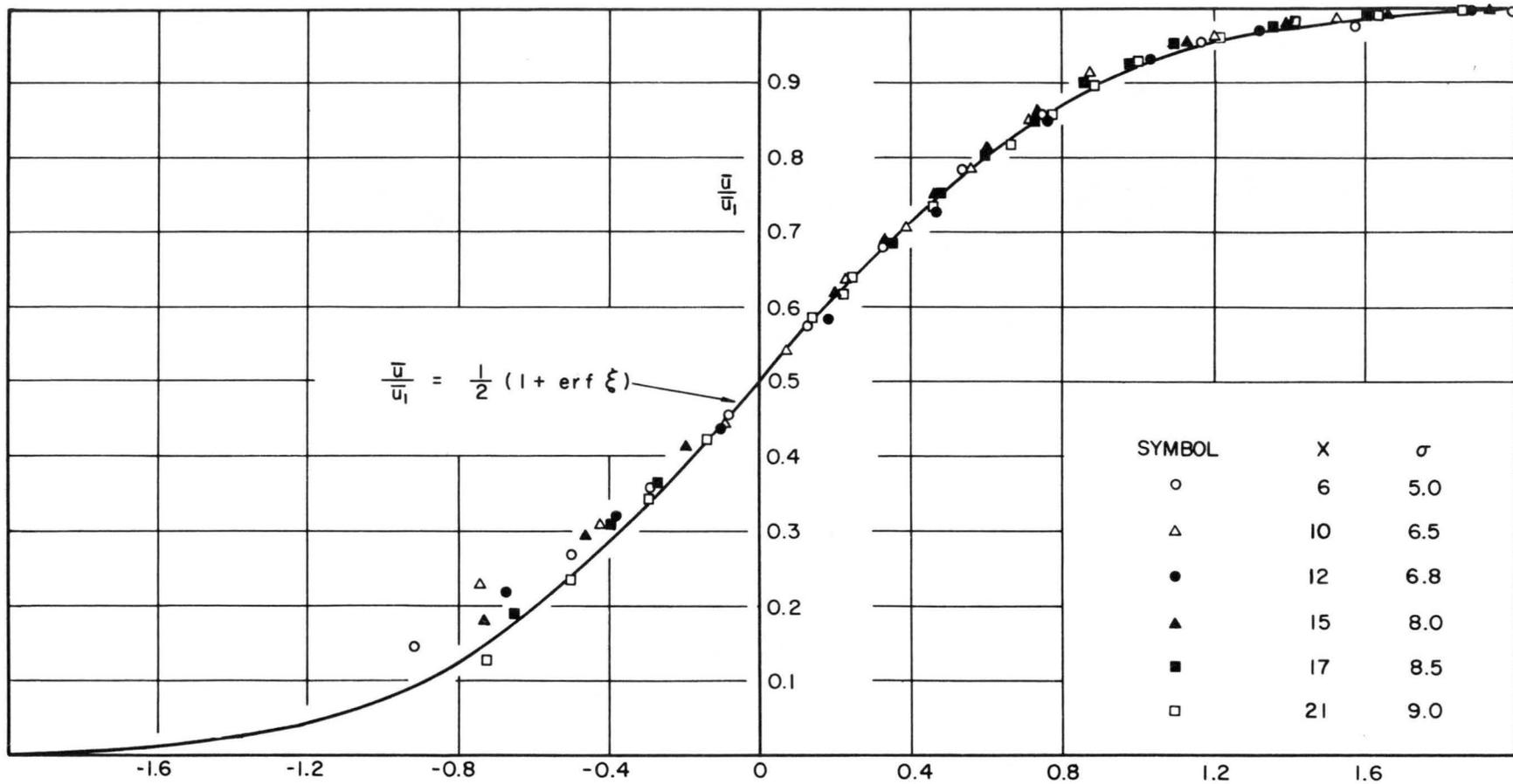
FIG. 23-4 COMPARISON OF THEORY AND VELOCITY MEASUREMENT FOR  $U_\infty = 30$  fps
