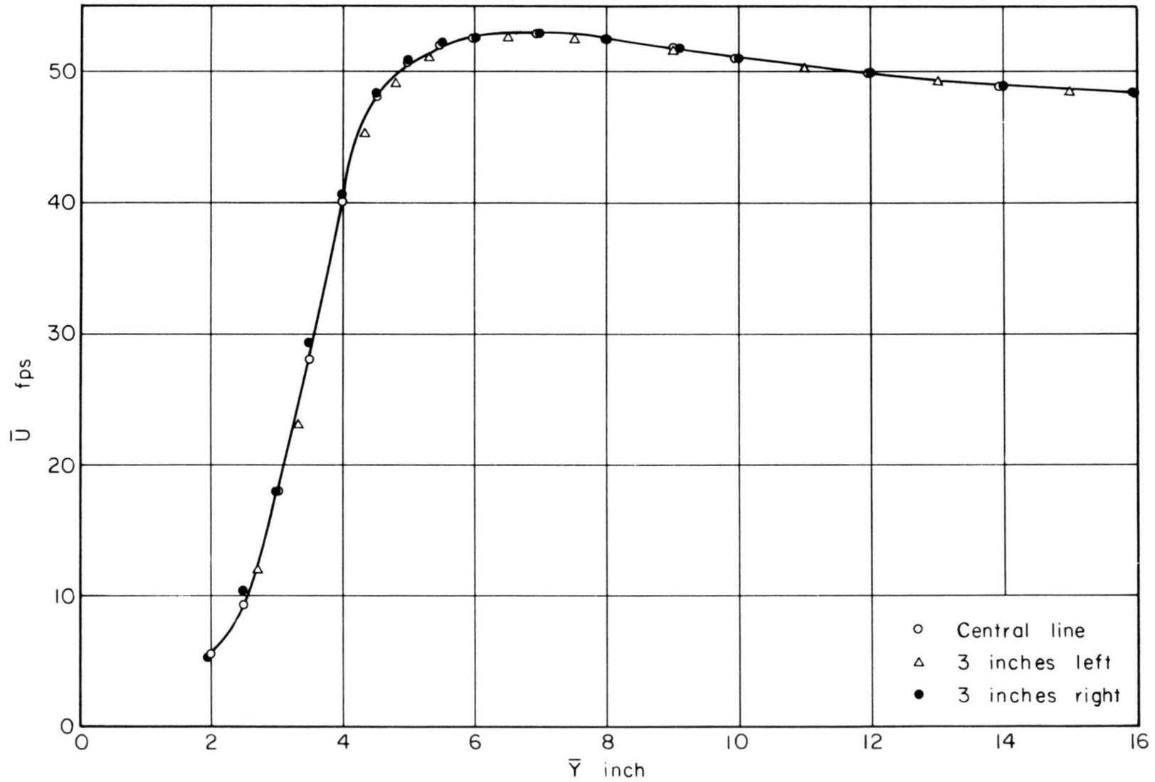
Fig. 5 Velocity profiles at  $X = 5''$  behind the wedge hill
