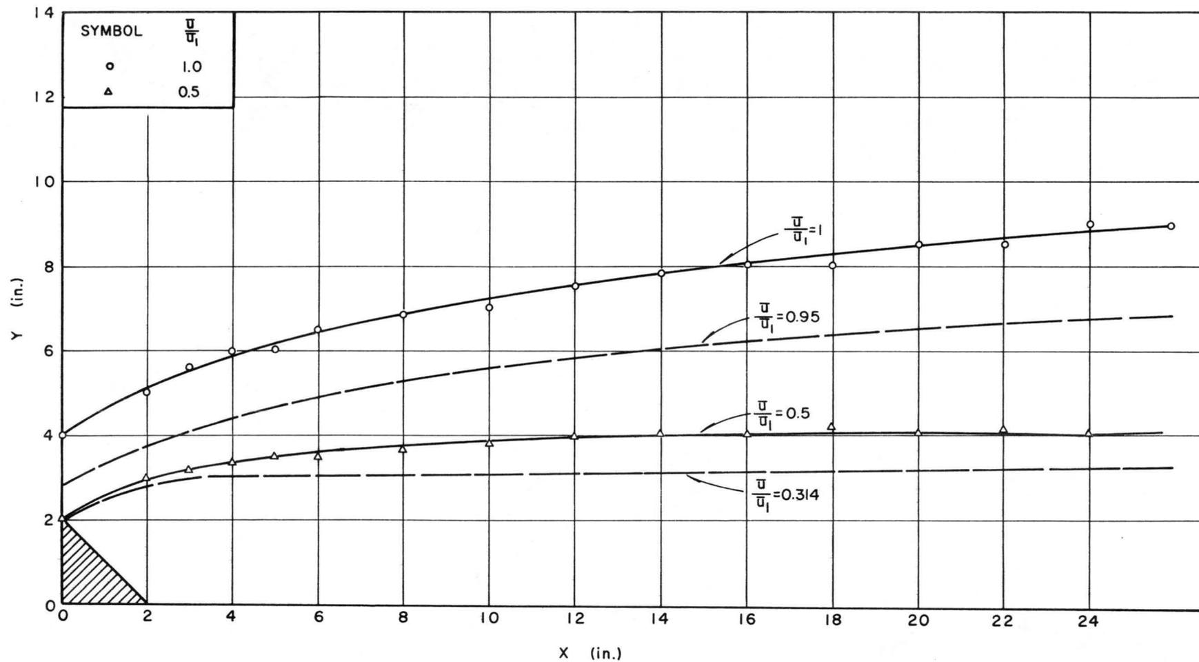
FIG. 13 UPPER JET BOUNDARY AND JET-AXIS WITH  $U_\infty = 45$  fps
