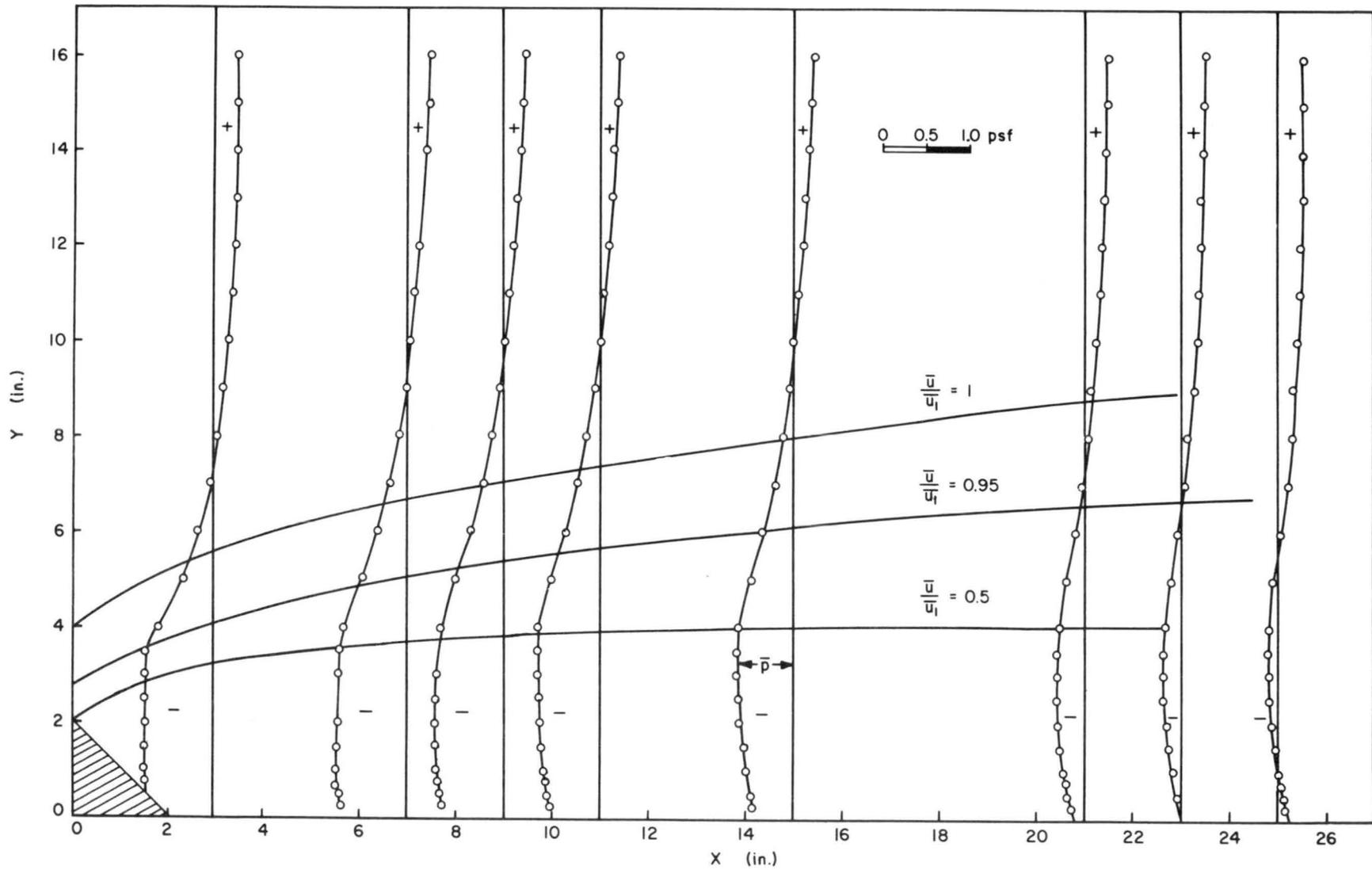
FIG. 20 DEVELOPMENT OF STATIC PRESSURE BEHIND THE HILL WITH  $U_\infty = 45$  fps.
