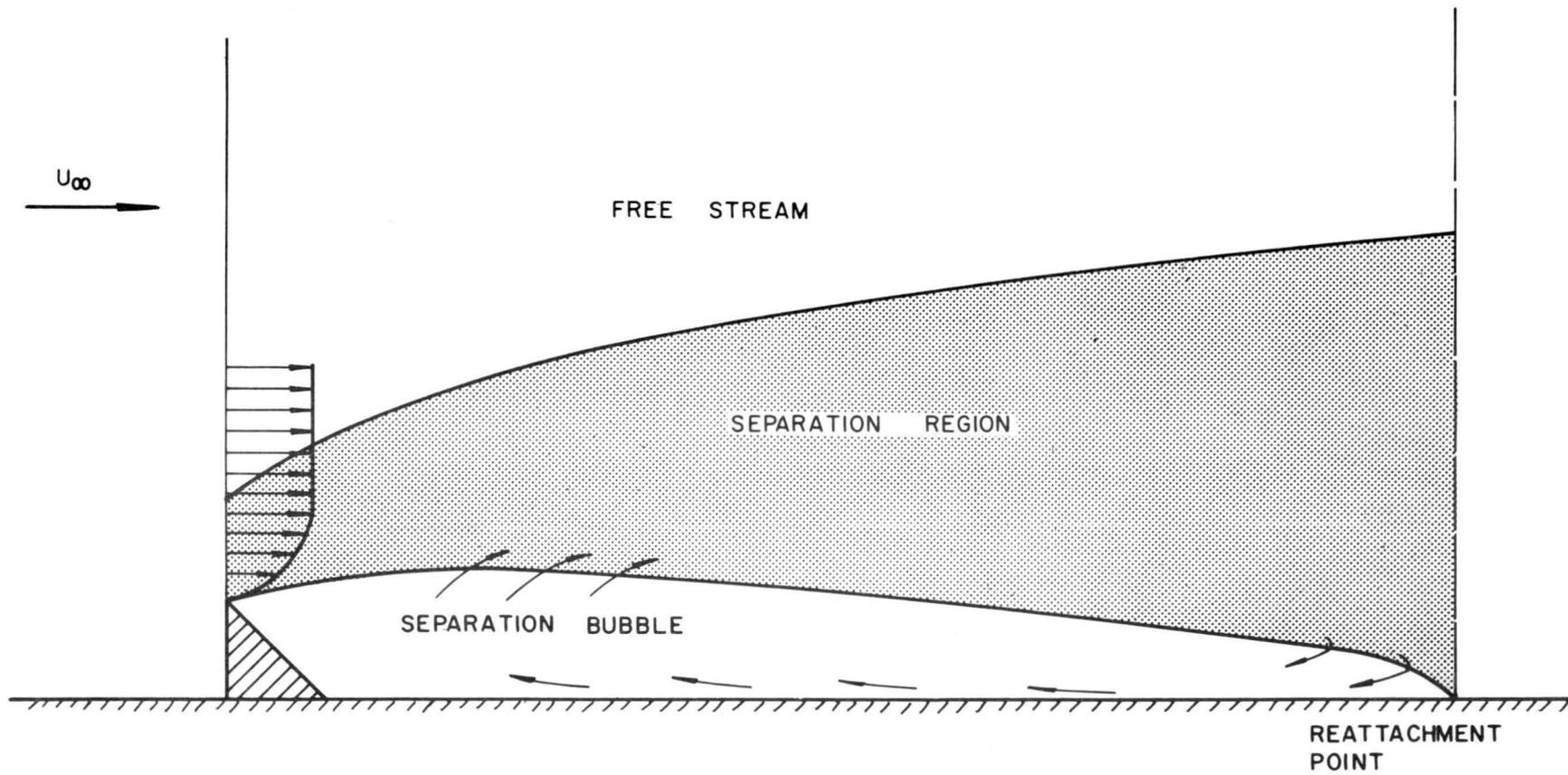
FIG. 1 FLOW FIELD BETWEEN HILL AND REATTACHMENT POINT.
