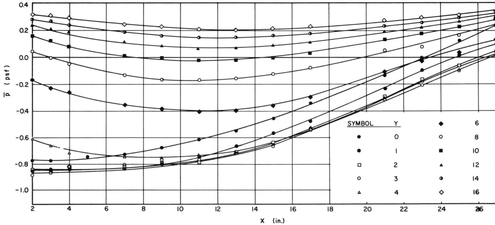
FIG. 19 VARIATION OF STATIC PRESSURE AT CONSTANT HEIGHTS ABOVE THE FLOOR WITH  $U_{\infty} = 45$  fps
