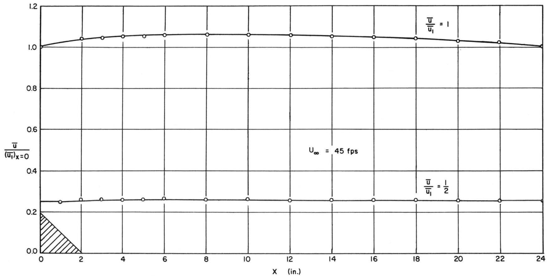
FIG. 14 VARIATION OF VELOCITY ALONG JET BOUNDARY AND JET AXIS.
