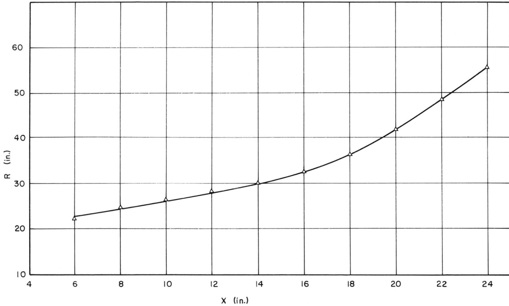
FIG. 22 VARIATION OF RADIUS OF CURVATURE  $R$  WITH  $X$   $U_{\infty} = 45$  fps
