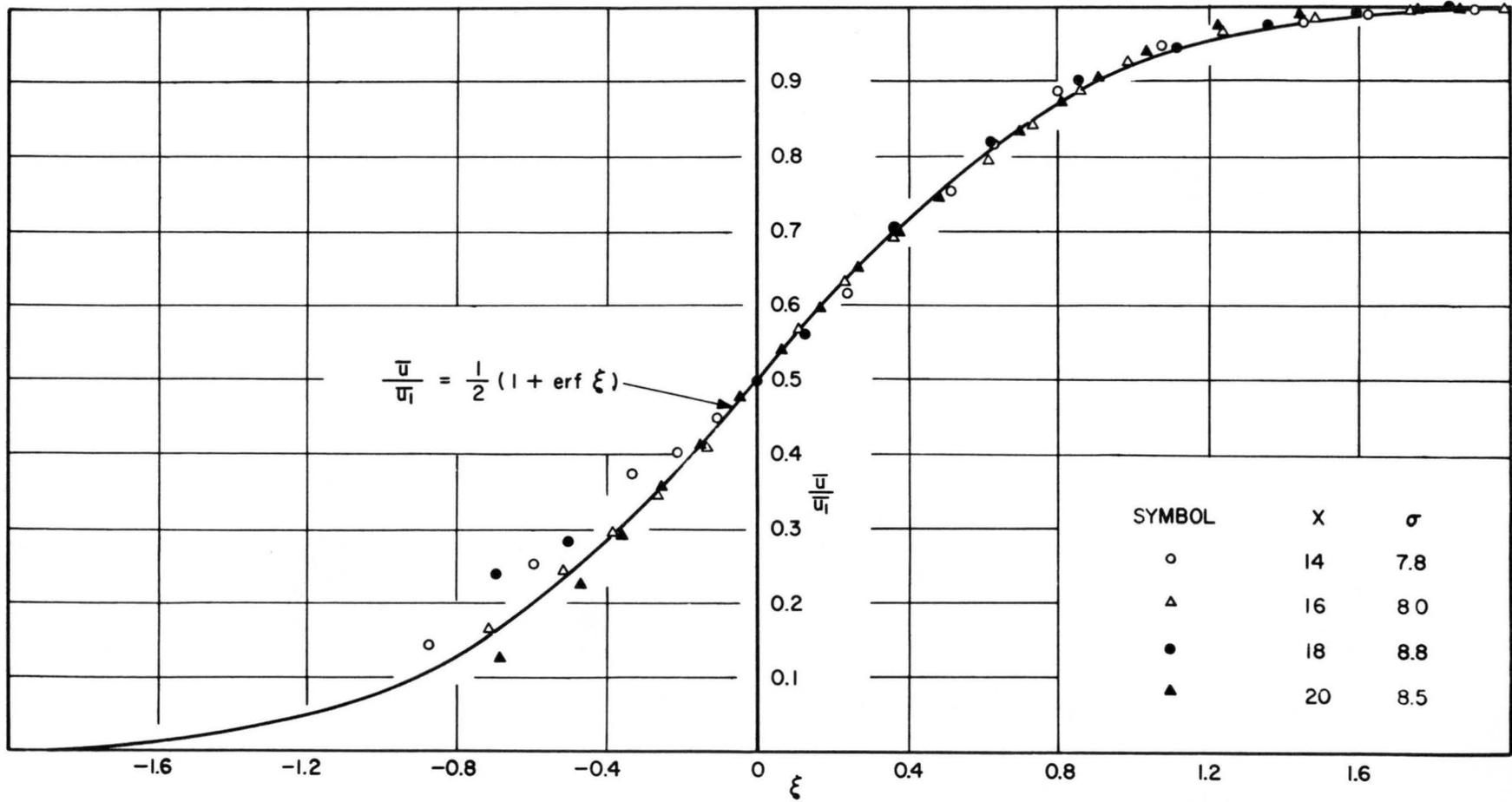
FIG. 23-2 COMPARISON OF THEORY AND VELOCITY MEASUREMENTS FOR  $U_{\infty} = 45$  fps.
