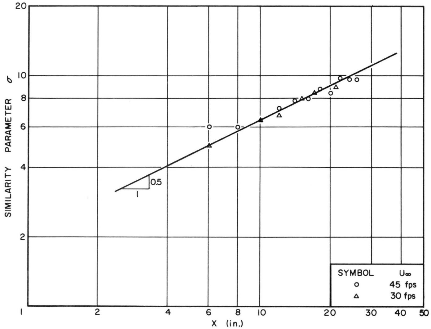
FIG. 24 VARIATION OF SIMILARITY PARAMETER  $\sigma$  WITH DISTANCE  $X$
