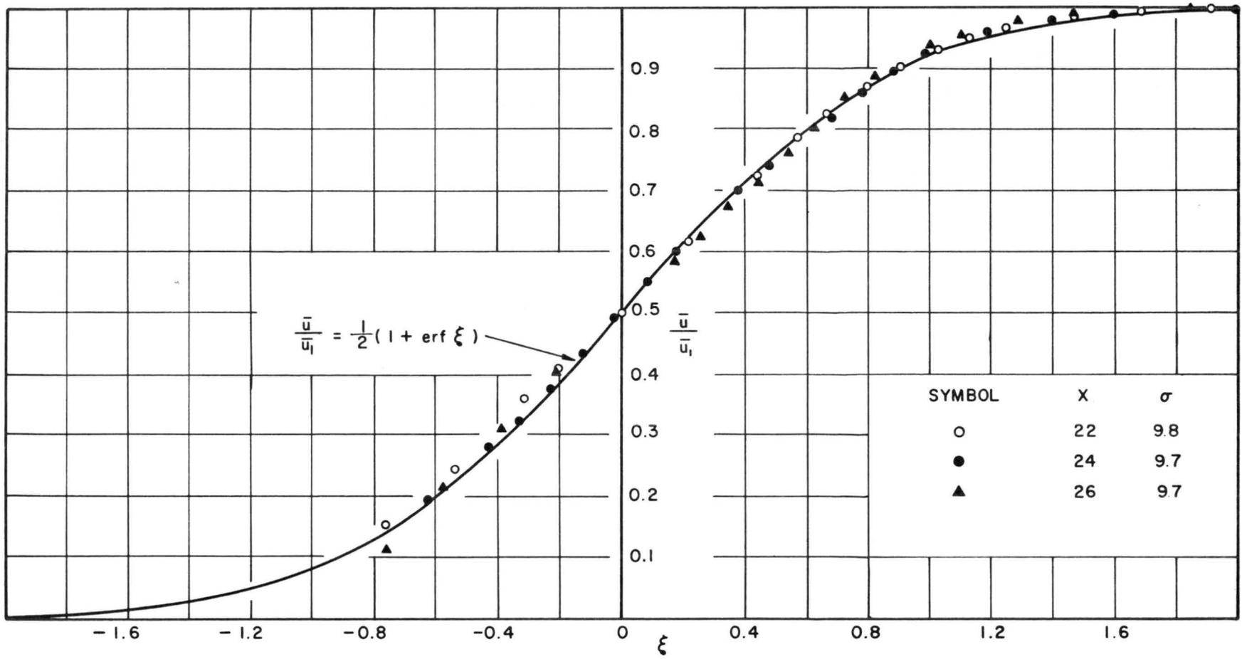
FIG. 23-3 COMPARISON OF THEORY AND VELOCITY MEASUREMENTS FOR  $U_\infty = 45$  fps
