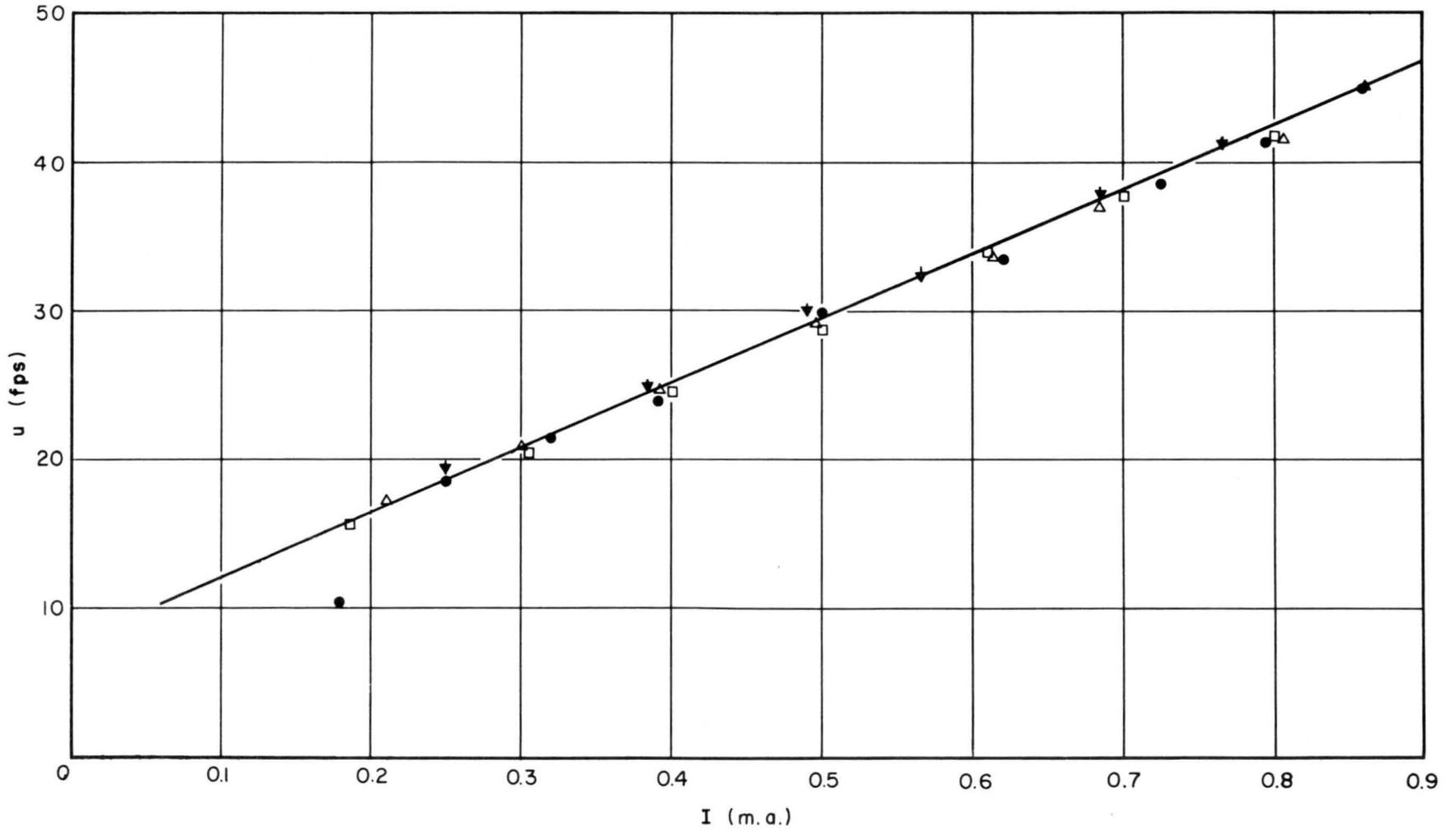
FIG. 9 CALIBRATION CURVE OF HOT WIRE
