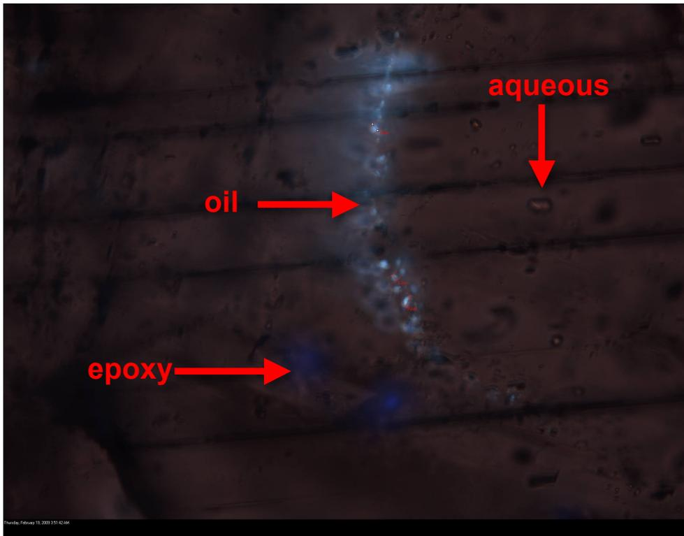
**Figure 3:** Micrograph from sample 30R 2263 showing the visible difference in fluorescence of oil inclusions, aqueous inclusions and epoxy under UV light. Field of view in this micrograph is 0.35mm.
