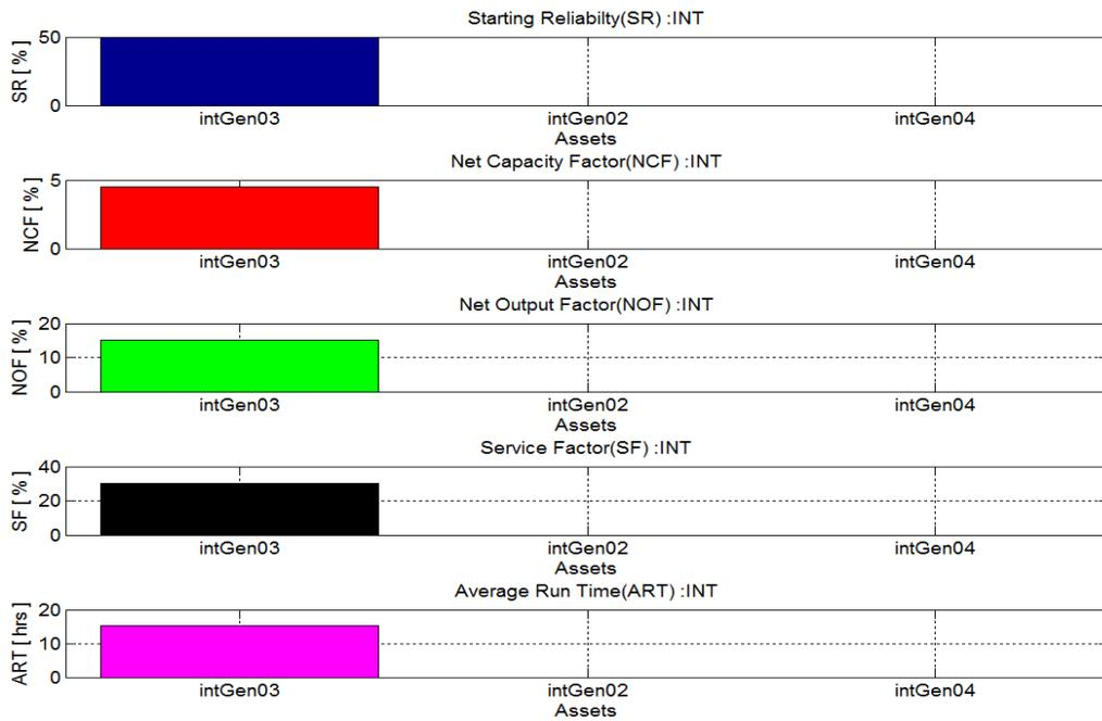
**Figure 4.4 NERC metrics for InteGrid Lab**
