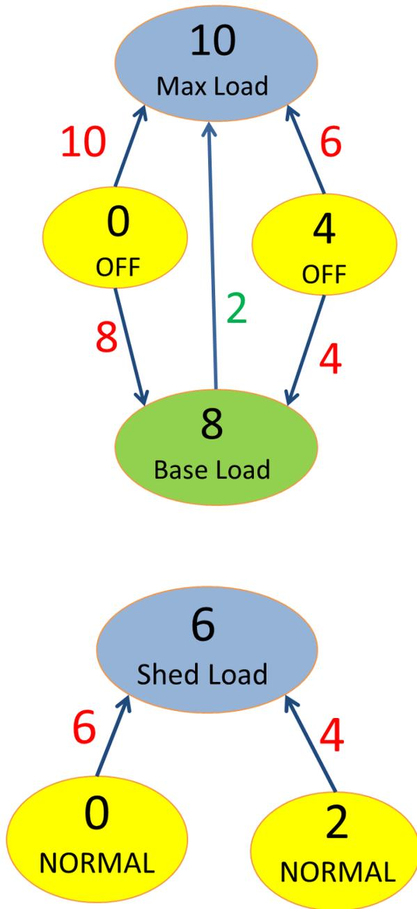
**Figure 3.2 Command change state diagram for generation and DR assets**
