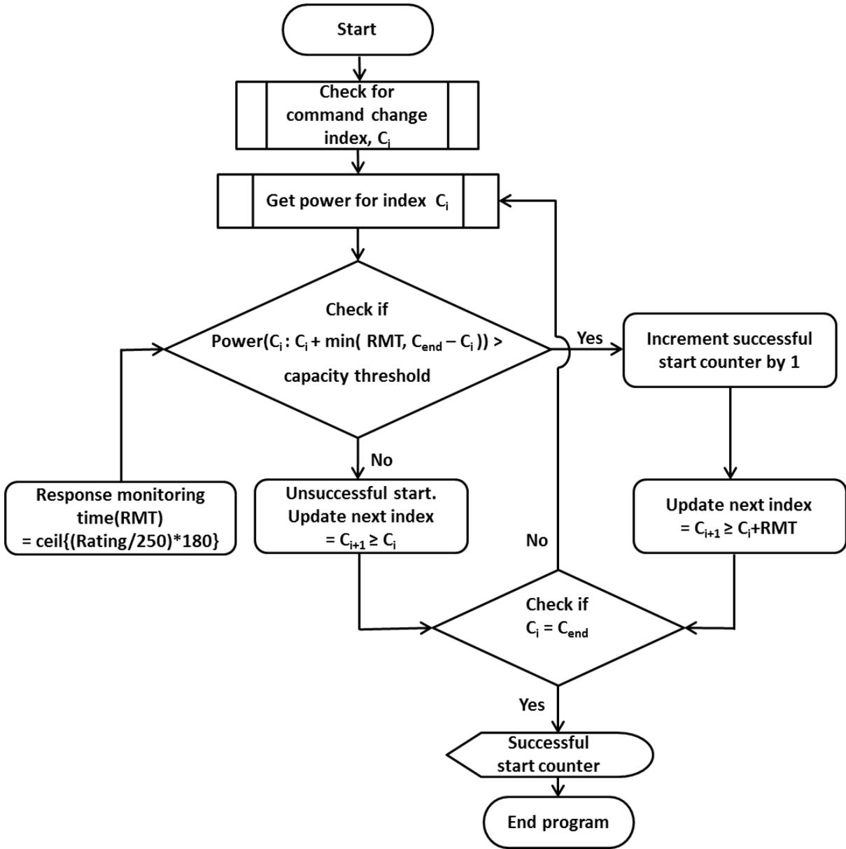
Figure 3.4 Flow chart for algorithm used to identify successful start of an asset
