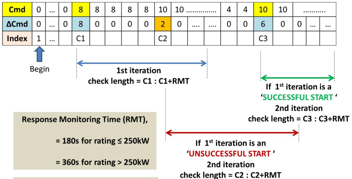
**Figure 3.3 Illustration of checking vectors for successful start**
