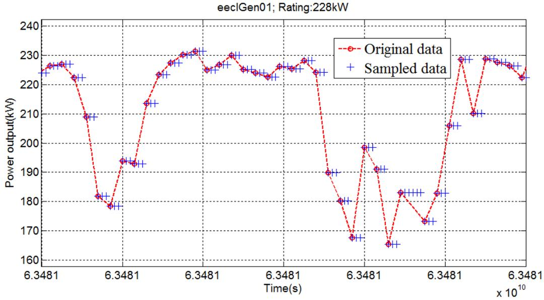
**Figure 2.11** Magnified views of the original and reduced data for asset *eeclGen01*
