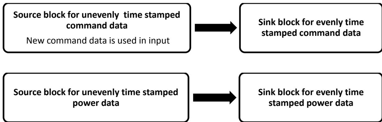
**Figure 2.7 Block diagram of Simulink model used for data interpolation**
