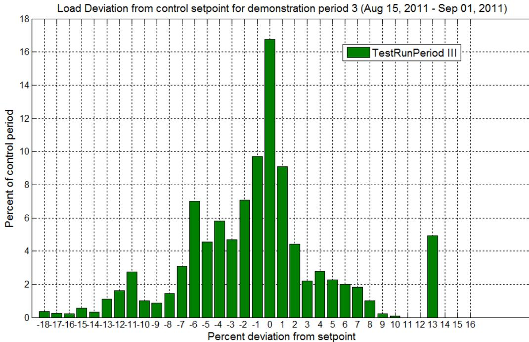
**Figure 3.10 Load deviations from control set points as percent of control set points for the third demonstration period of FortZED RDSI**
