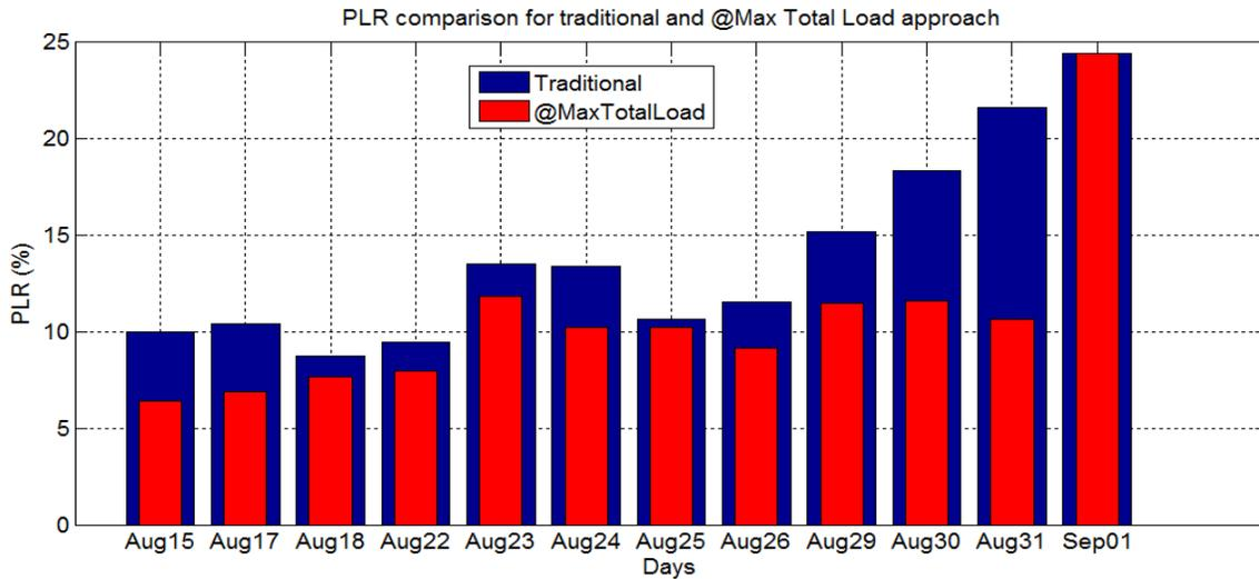
**Figure 3.7 Comparison of percent peak load reduction calculations for the traditional approach and at time when total feeder peak occurs**
