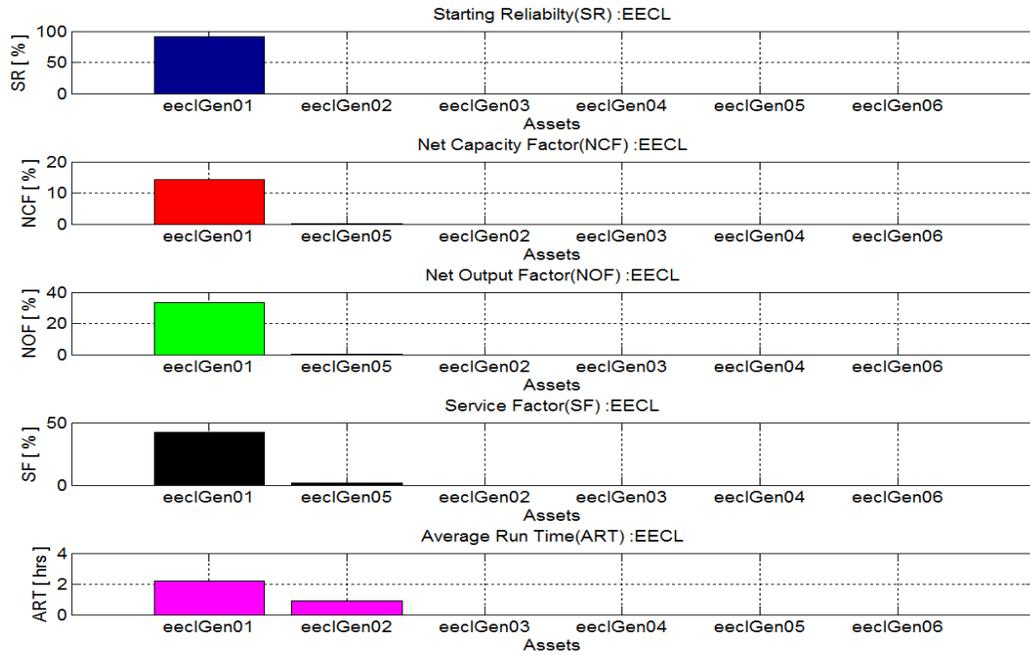
**Figure 4.3 NERC metrics for Engines and Energy Conversion Lab**
