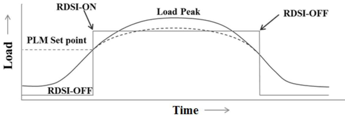
Figure 2.2 Illustrative diagram of peak load Reduction in RDSI [2.1]
