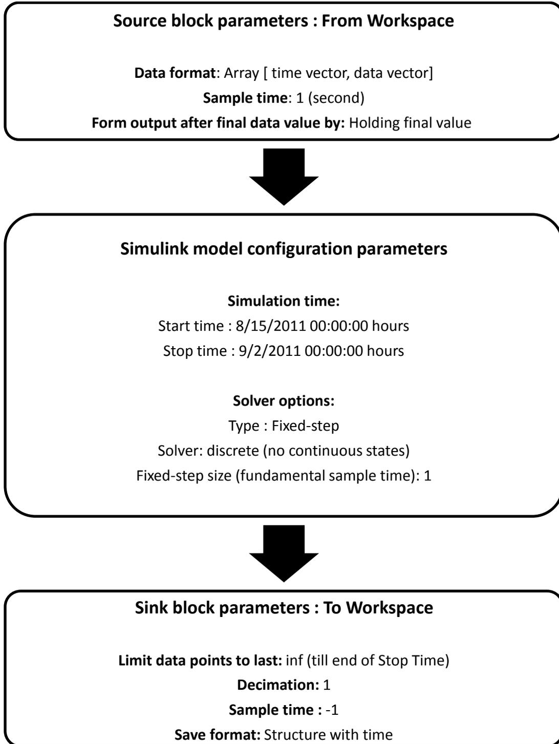
**Figure 2.14 Block diagram of Simulink model parameters.**
