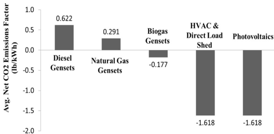
**Figure 2.3 Average net carbon dioxide emissions per unit electricity generated or saved through different kinds of generation and load shedding assets [2.1]**
