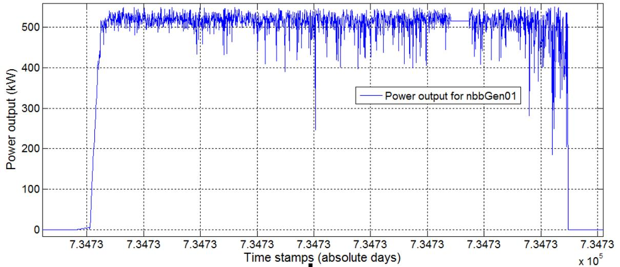
**Figure 2.6 Example of power values plotted against time stamps for *nbbGen01***
