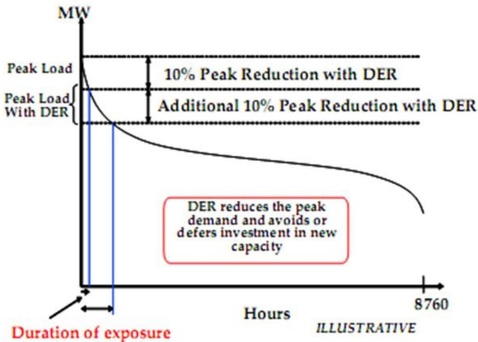
**Figure 3.6 Illustrative load curve for a year for peak load reduction calculation (Image taken directly from [3.9])**
