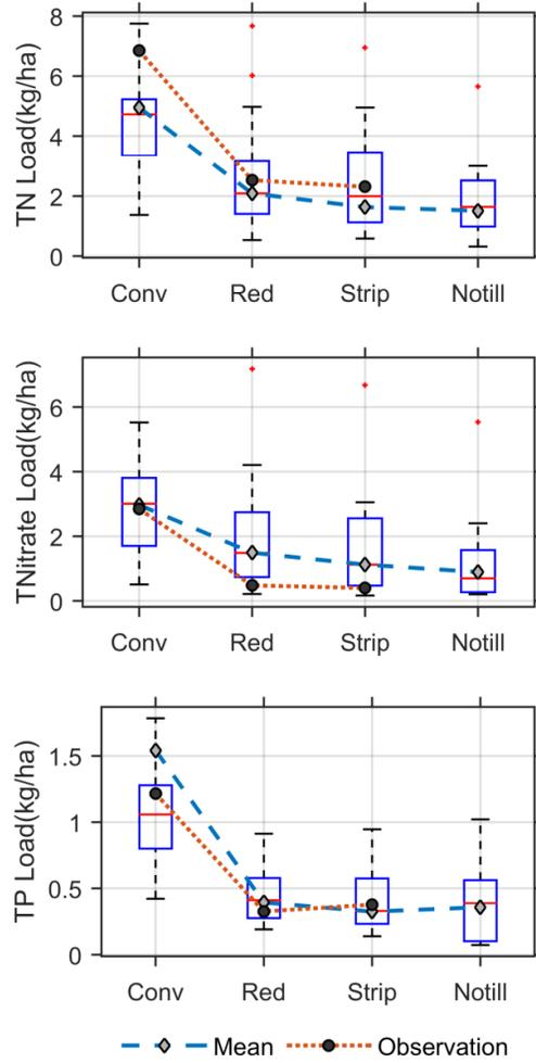
**Figure 2.2: SWAT-CP output of average annual loads over a 16 year period (2002-2017) for total nitrate, total phosphorus, and total nitrogen with average annual field observation values**
