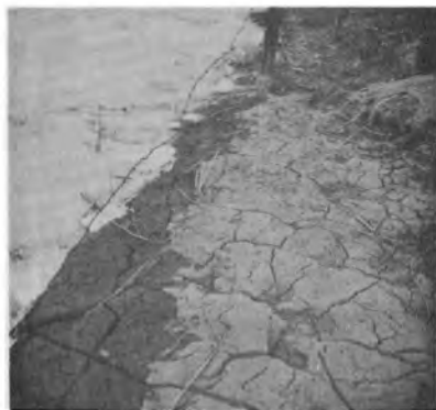
Close-up view of drying cracks and sedimenting mixture.
