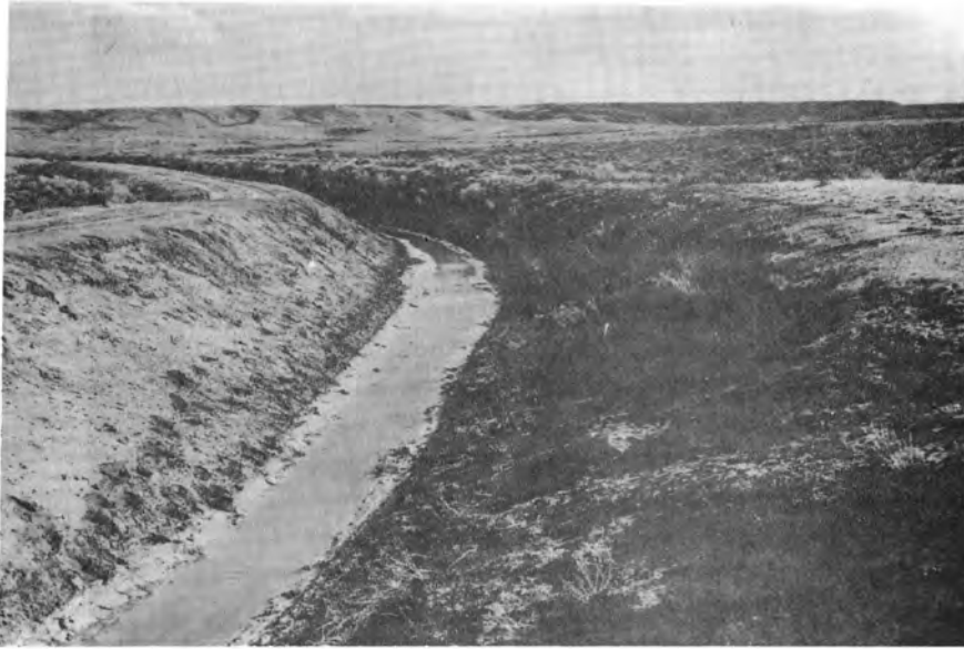
Bentonite filter cake in lateral bottom after ponding interval with sedimenting mixture. Irrigation deliveries were begun several weeks later. May 8, 1953
