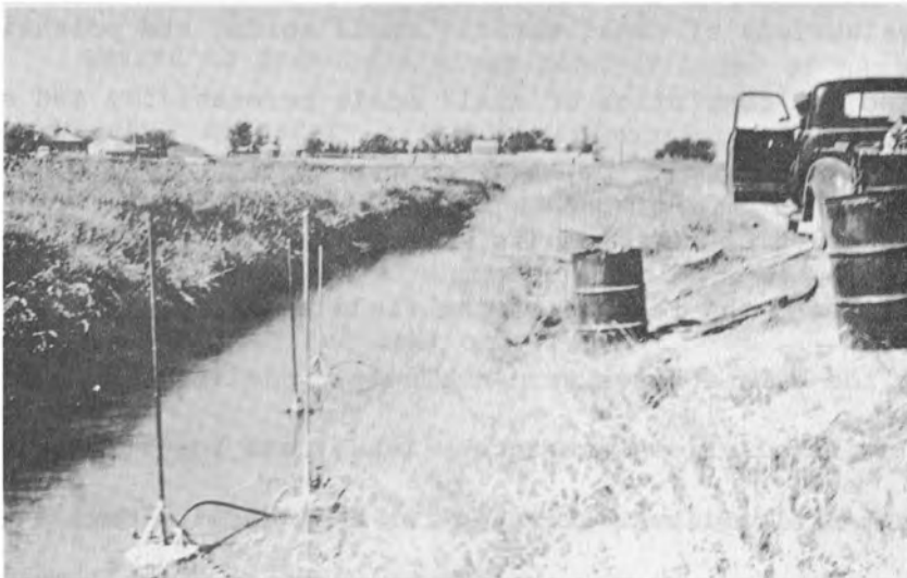
Seepage meter set-ups for feasibility tests in dune sand materials, Horse Creek Canal. Same equipment and procedure were used in Kendrick Project testing.
