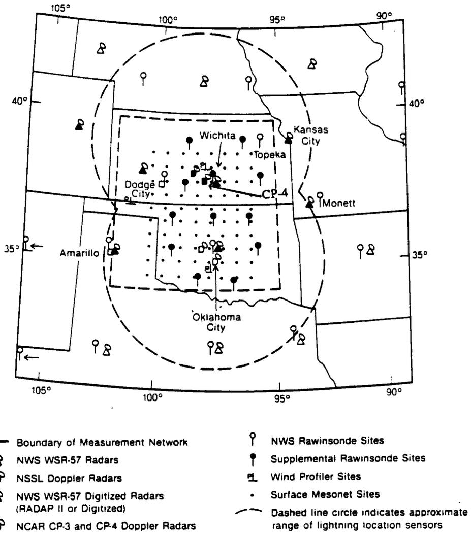
Fig. 2.1: The OK PRE-STORM observational mesonet. From Cuning (1986).
