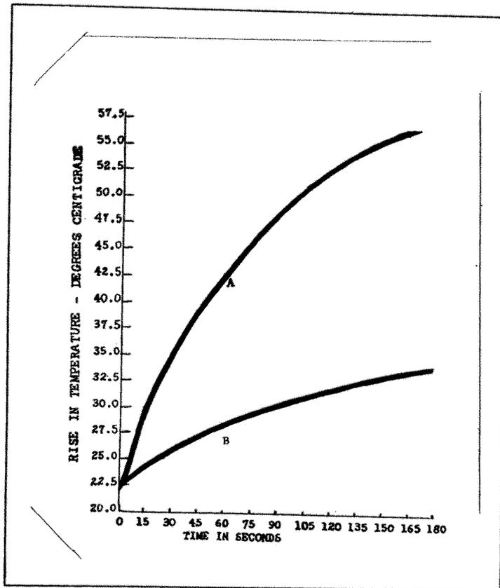
Fig. 1. Change in temperature as related to time of exposure to Quartz Mercury Vapor Lamp.
