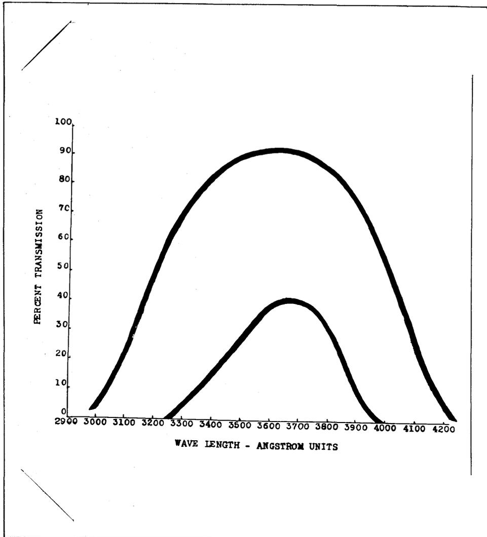
Fig. 2. Calculated transmission curves for filters A586 and red-purple 3.29mm. thick.
