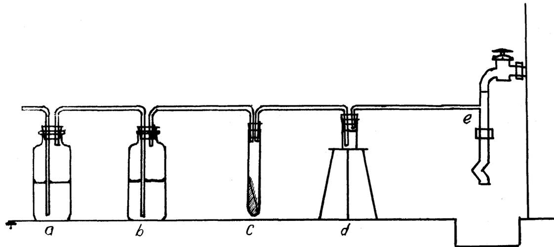
Fig. 19. Apparatus for determining amount of  $\text{CO}_2$  produced by a fungus when under variable light conditions.
