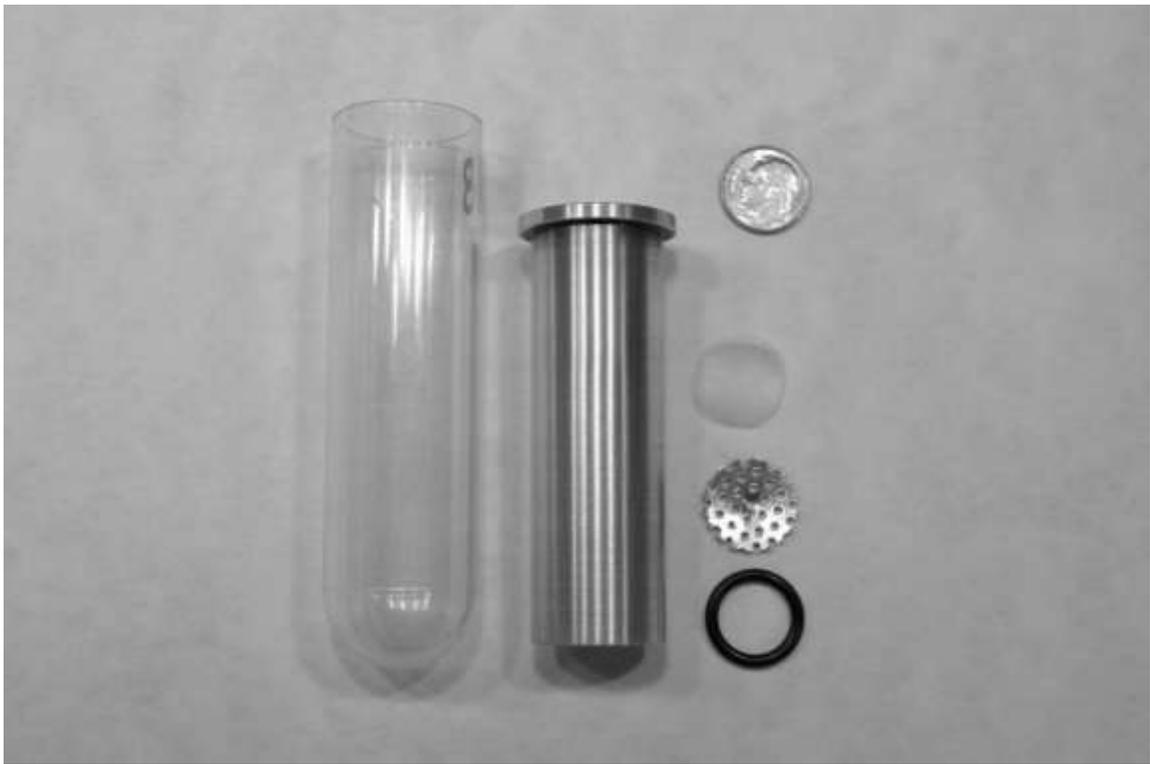
Figure 2.1. Centrifuge filter apparatus used for centrifugation  $K_d$  assay.
