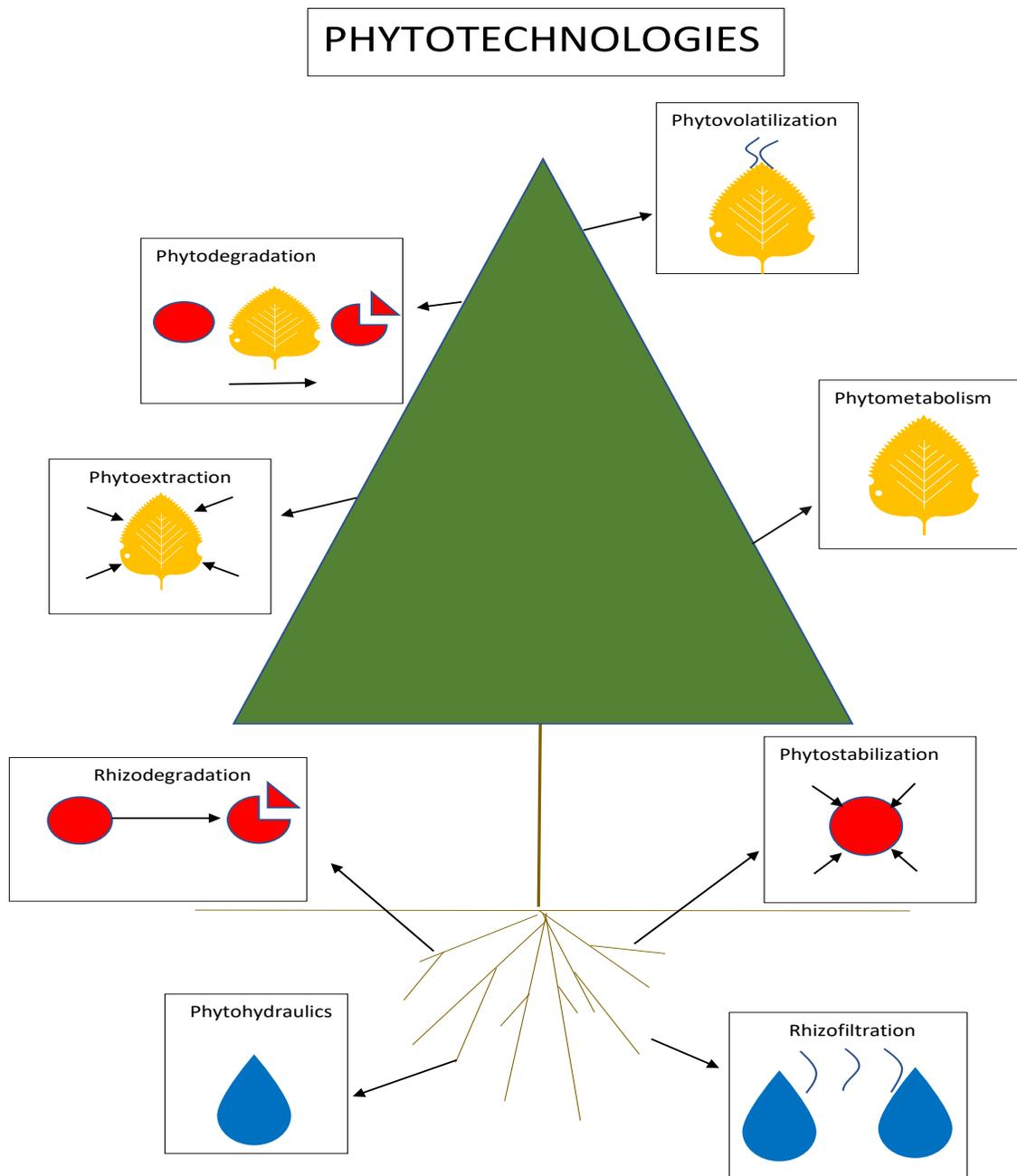
Figure 1.1 Different phytotechnologies used by plants. The utilized method is plant: pollutant specific. Red circles are pollutants. Wavy lines indicate release into the atmosphere. Arrows indicate direction of pollutants. Modified from Kennen and Kirkwood, 2015.
