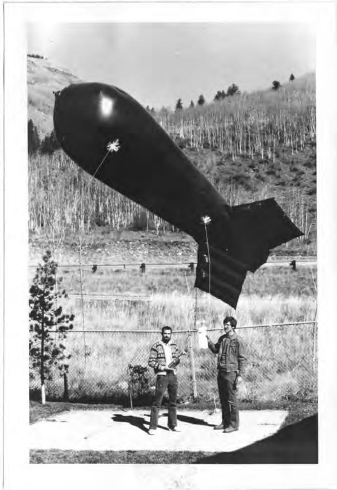
Figure 11. Normal operating configuration of tethered sonde balloon and airborne package.
