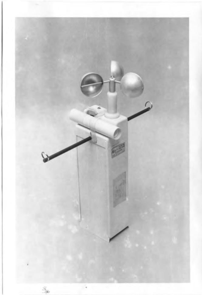
Figure 10. Tethersonde battery-powered airborne sensor and telemetry package.
