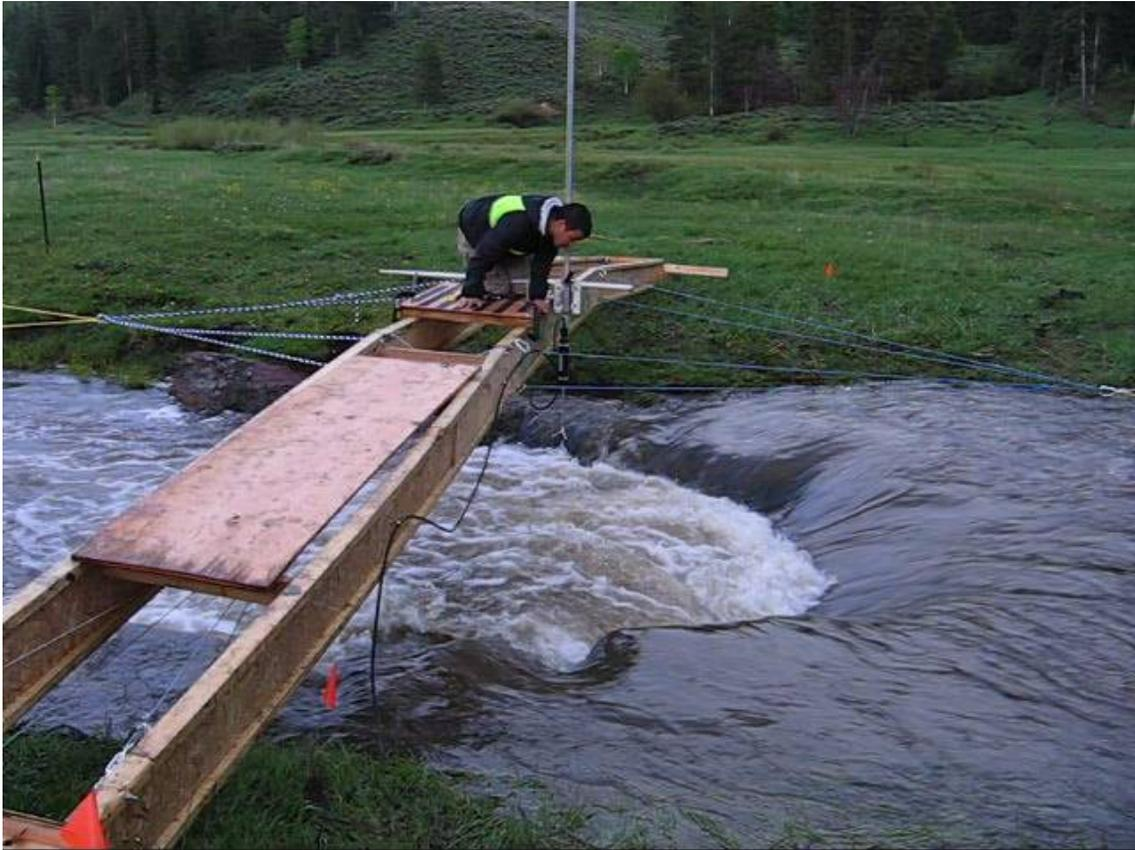
Figure 3.7 – Bridge with sampling platform and field ADV probe used for high flow measurements.
