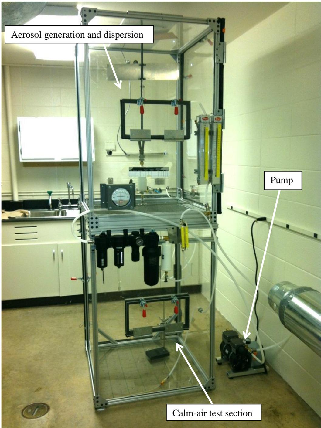
**Figure 7: The 2.5 m laboratory test chamber with aerosol generation and dispersion section (Figure 8) and calm-air test section (Figure 9), and pump.**
