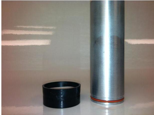
**Figure 11: PIPS tube and 37-mm cassette with filter.**
