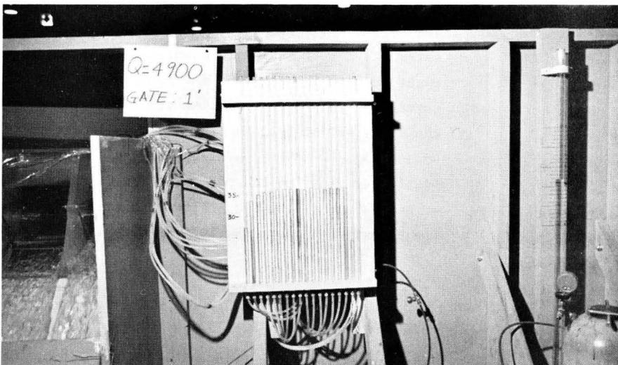
c. Manometer Board, and Tubing for Gate Piezometers
