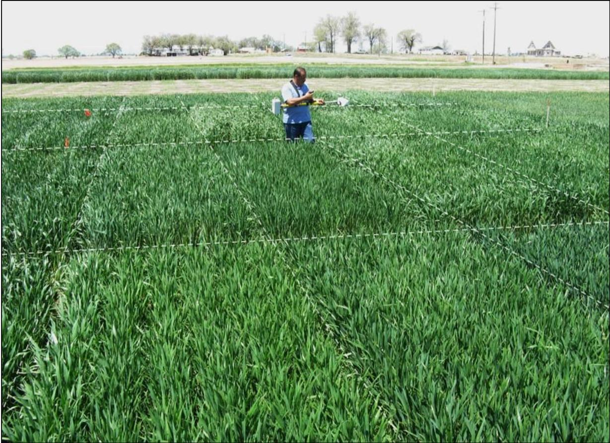
Figure 1.1 The NDVI readings were collecting using Greenseeker® handheld optical sensor. Plot boundaries are highlighted with white dashed lines.
