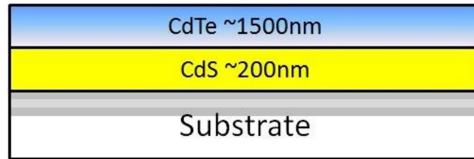
Figure 1.2: Schematic of Typical Layered Structure of Samples Produced Using the CSU ERC Manufacturing System.
