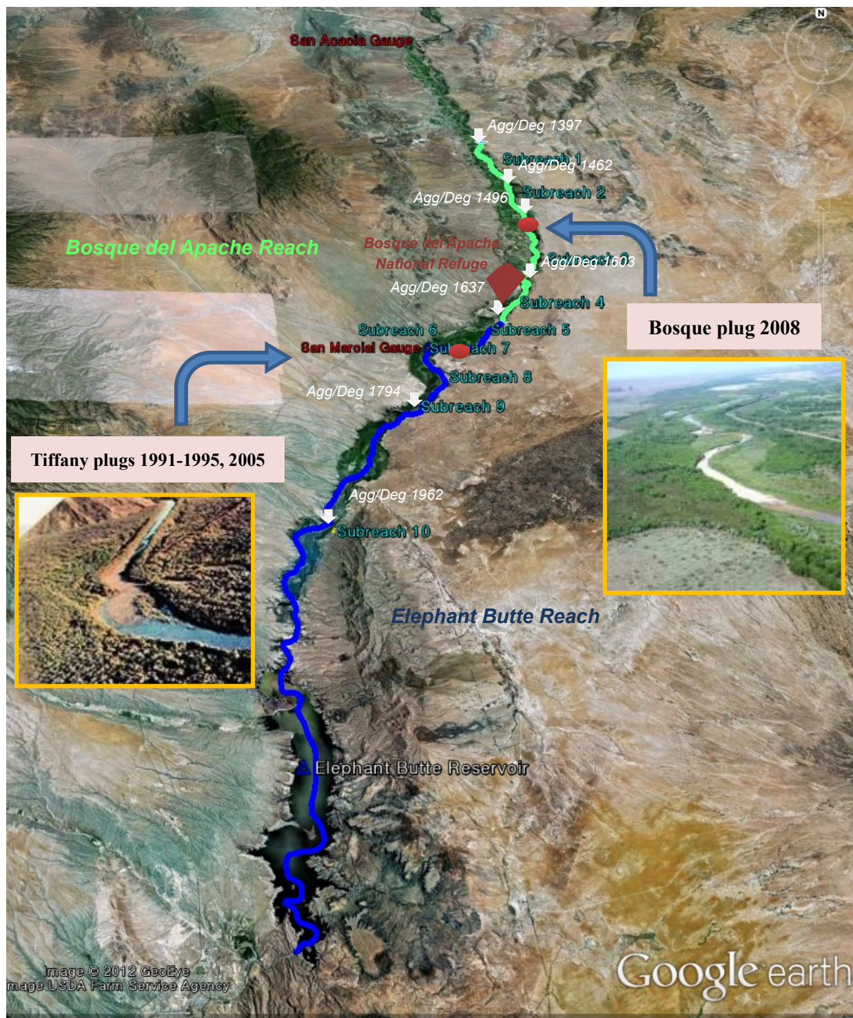
Figure 3.6. Delineation of sub-reaches and location of sediment plugs
