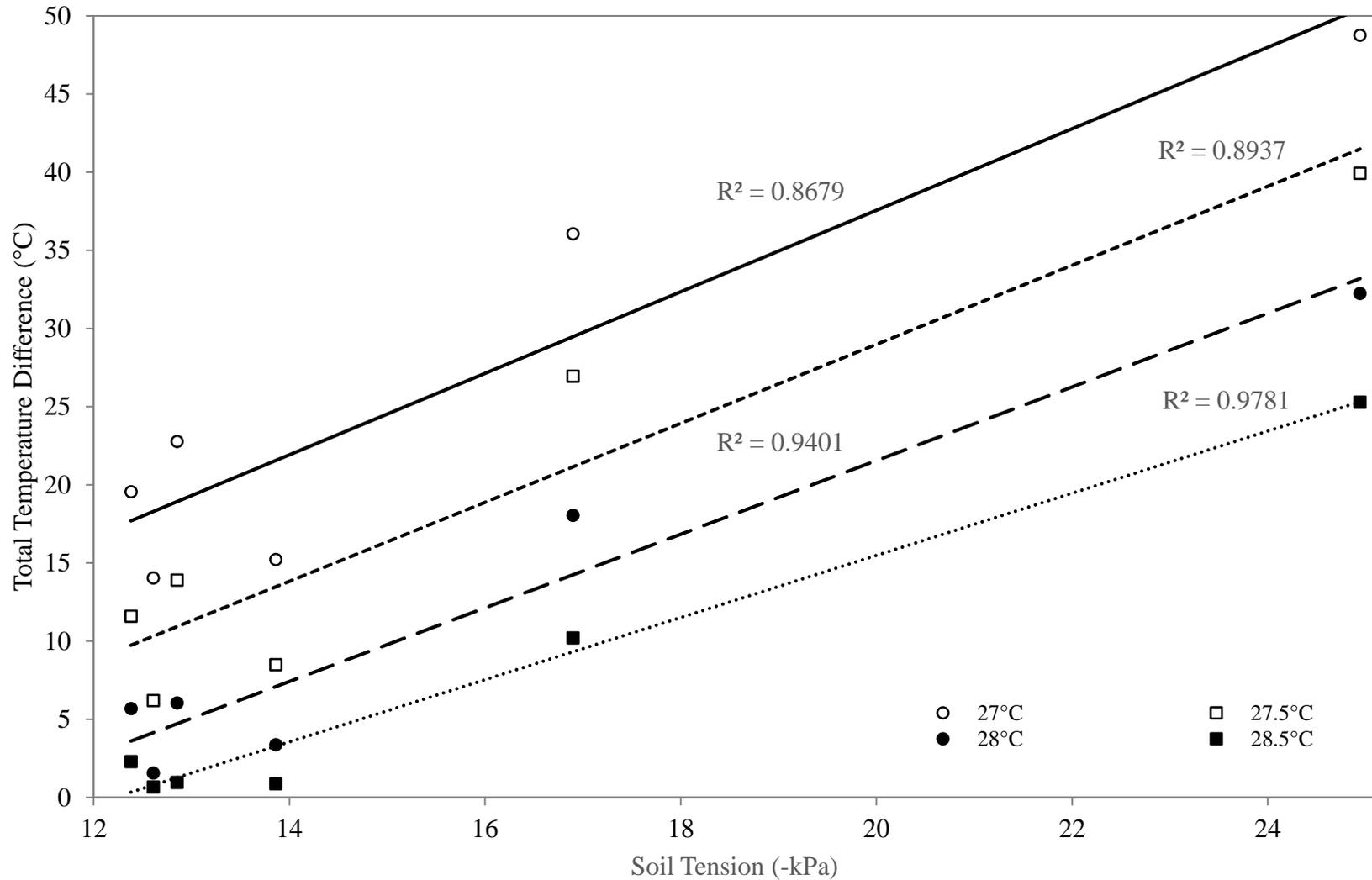
Figure 2.11. Total Temperature Difference, which is calculated over one day by subtracting the canopy temperature from the threshold temperature when it is exceeded, as a function of soil moisture tension on August 30. Four different temperature stress thresholds (27 – 28.5°C) are included to demonstrate the tendency of the coefficient of determination to increase up until zero stress values are produced.
