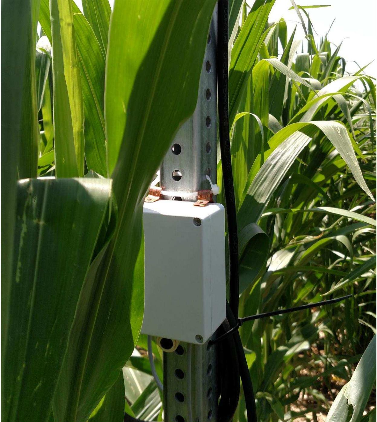
Figure 2.01. Image showing infrared thermometer pointed into the maize canopy. The actual thermometer (black) is at the bottom of the weather resistant box.
