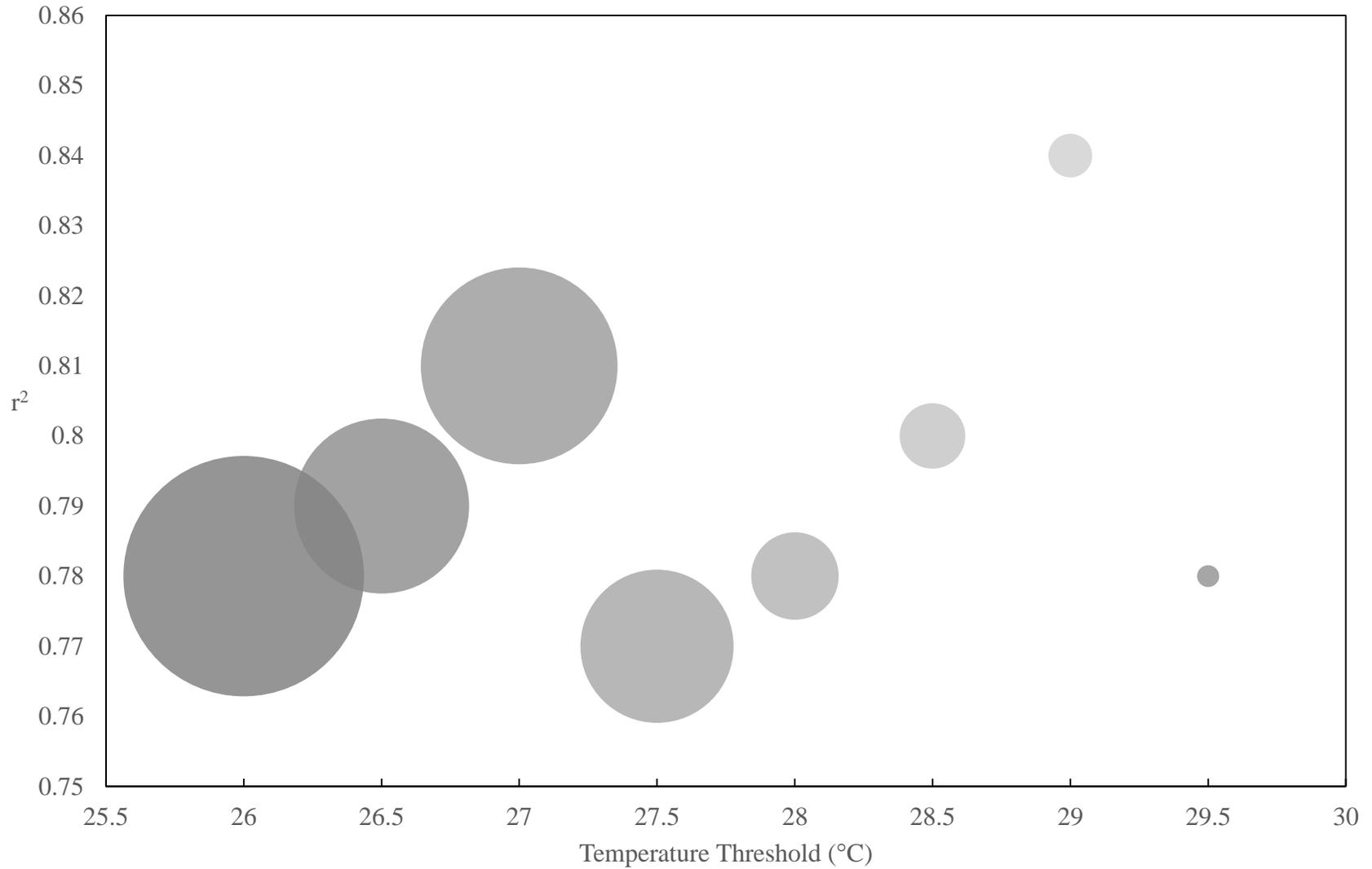
Figure 2.07. Average coefficient of determination ( $r^2$ ) for linear models using each temperature threshold examined in this study with soil moisture tension measured at 20 cm depth. The number of days statistically significant using the threshold is indicated by the size of each circle.
