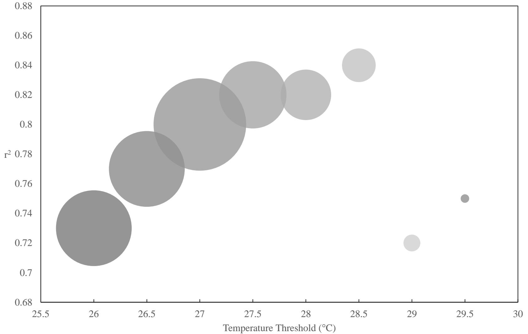
Figure 2.10. Average coefficient of determination ( $r^2$ ) for linear models using each temperature threshold examined in this study with soil moisture tension measured at 45 cm depth. The number of days statistically significant using the threshold is indicated by the size of each circle.
