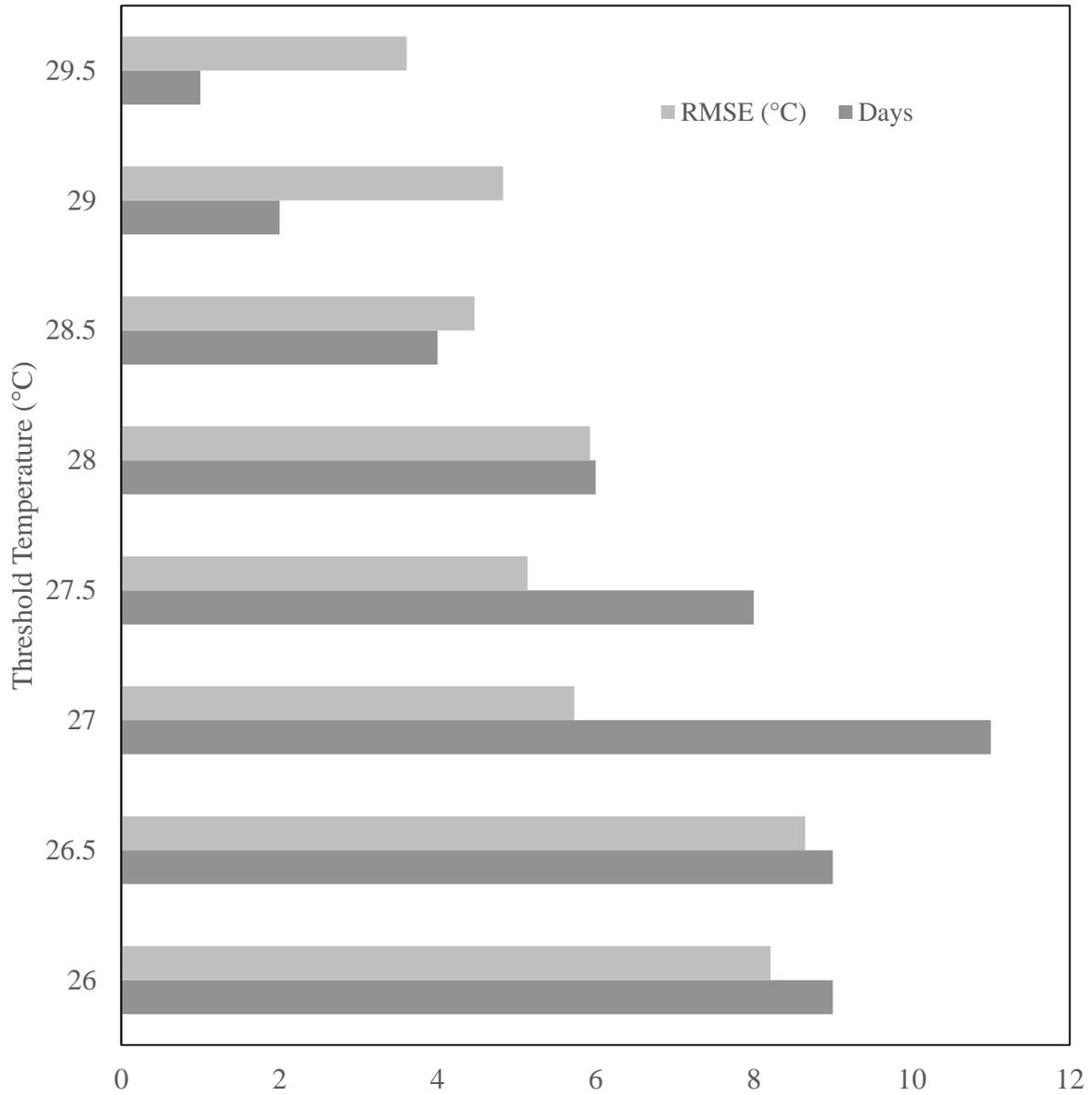
Figure 2.09. Number of statistically significant days and average root mean squared error (RMSE) for linear models using each of the temperature thresholds examined in this study for soil moisture tension measured at 45 cm depth.
