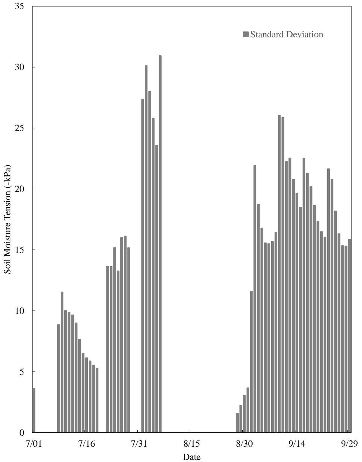
Figure 2.05. Standard deviation of soil moisture tension measured at 20 cm depth as a function of time. The gaps indicate time periods where data was removed during the data cleaning process.
