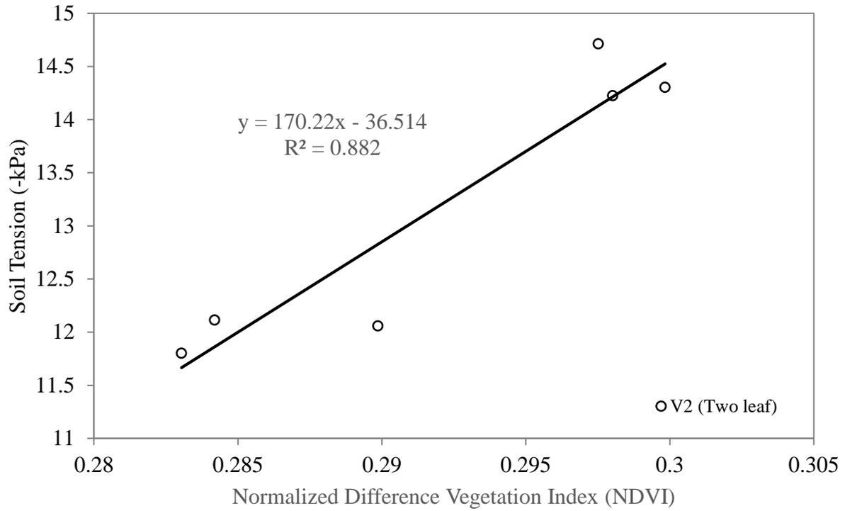
Figure 1.7. Soil tension (-kPa) as a function of NDVI for the V2 (two leaf) growth stage.
