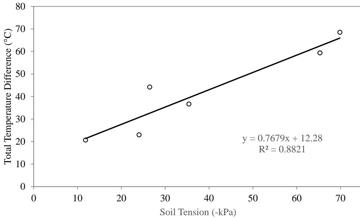
Figure 2.04. Total Temperature Difference, which is calculated over one day by subtracting the canopy temperature from the threshold temperature when it is exceeded, as a function of soil moisture tension measured at 20 cm depth on August 5 (tasseling crop growth stage).
