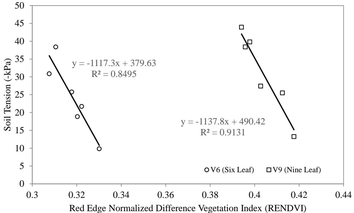
Figure 1.3. Soil tension (-kPa) as a function of RENDVI for V6 and V9 maize growth stages.
