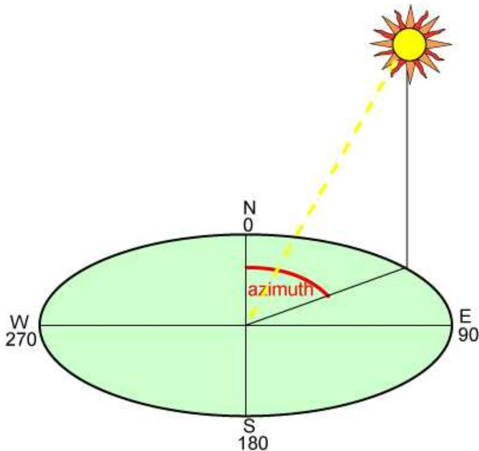
Figure 2.12. Solar azimuth represented by the red angle with solar incidence at the dotted yellow line. Adapted from Honsberg and Bowden (2016).
