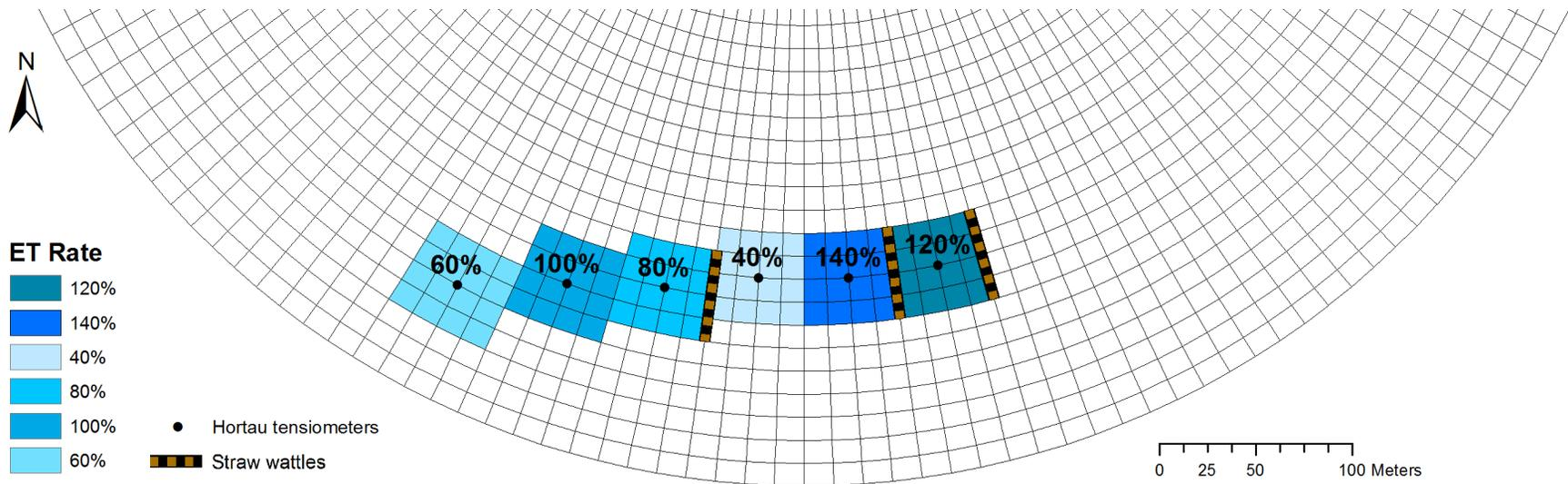
Figure 1.1. Variable rate irrigation grid used for the center pivot at Colorado State University Agricultural Research Development & Education Center. Irrigation treatments are represented as filled cells. A different color designates each zone and includes a point for the tensiometer locations, which are labeled with the percentage of estimated evapotranspiration used to calculate irrigation requirements for this study in 2015.
