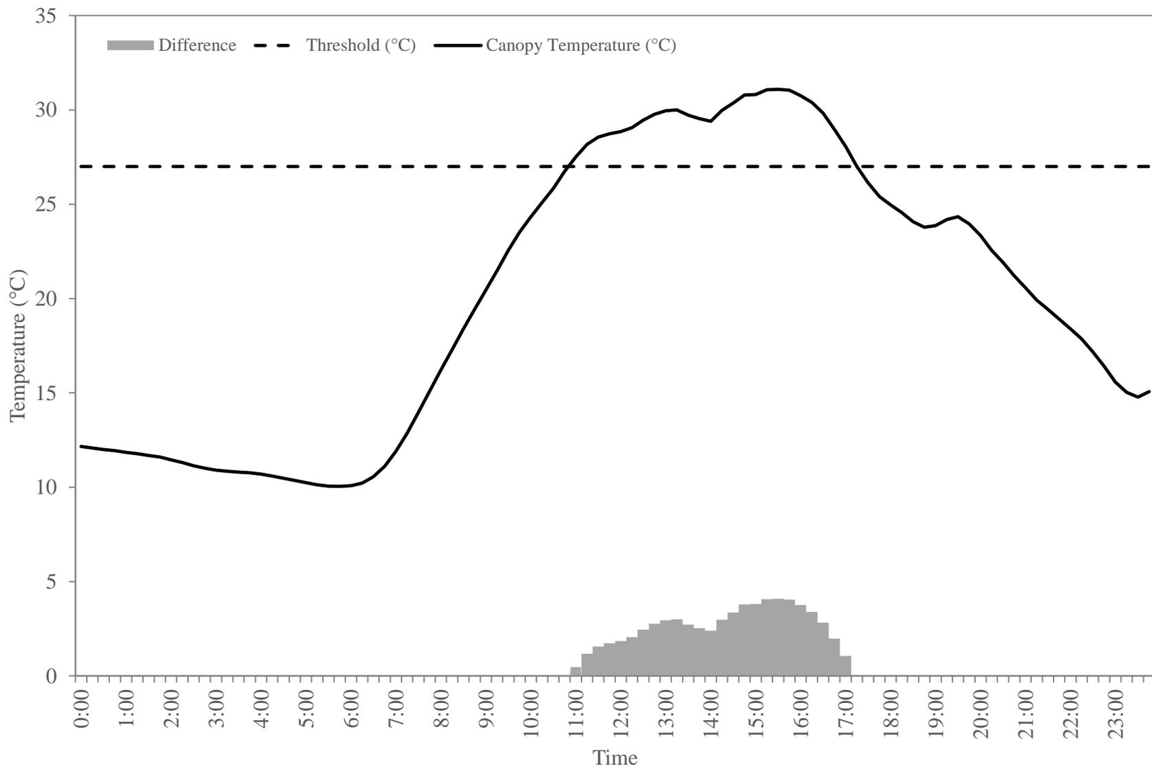
Figure 2.02. Representation of the daily total temperature difference, which is calculated by subtracting the canopy temperature (solid line) from the threshold temperature (dashed line) when it is exceeded. The resultant difference area is designated by the gray bars. For a more clear visual, the canopy temperature curve was formed using a five point triangular smoothing process for August 5<sup>th</sup> data.
