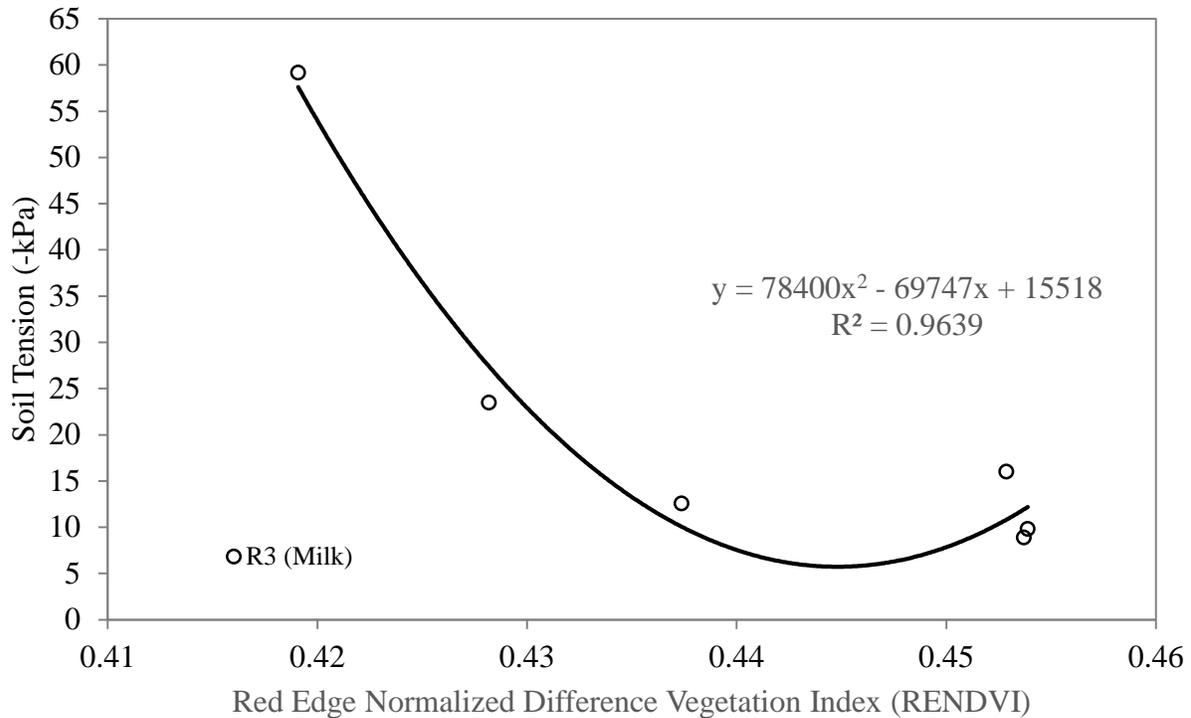
Figure 1.4. Soil tension (kPa) as a function of RENDVI at the R3 (milk) maize growth stage.
