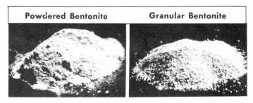
Good high-swell bentonite works best in most sealing jobs. It can be powdered or granular. Powdered bentonite costs less, but it is dusty. Granular bentonite has little dust, spreads easily as a blanket, but costs more.
