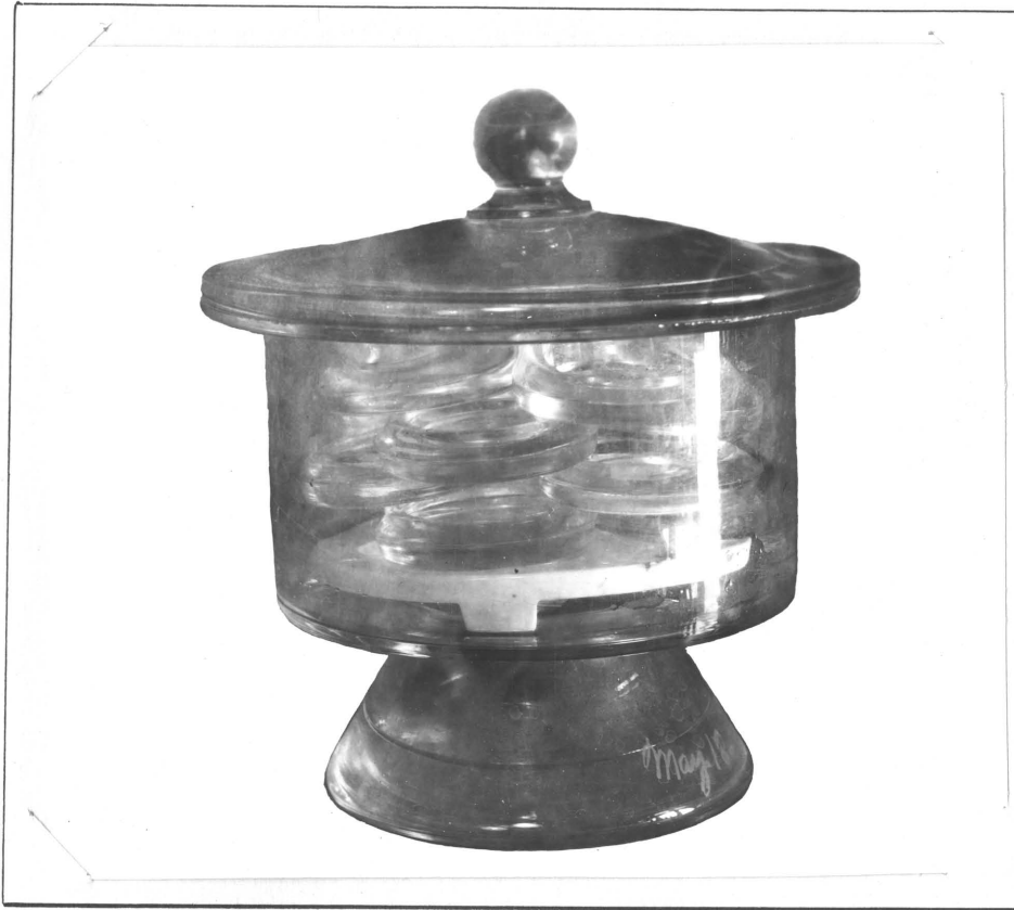
Fig. 1. Desiccator used as moist chamber showing method of spore germination in Syracuse dishes.
