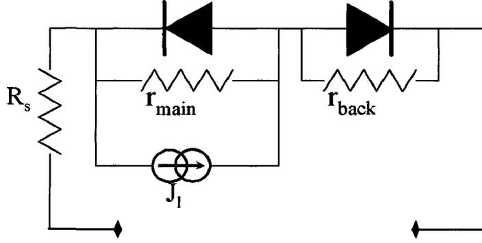
Figure 3.2: The two diode model proposed in [25] describes the behavior of a Schottky back contact as a leaky, reverse-polarity diode connected in series with the main junction diode.
