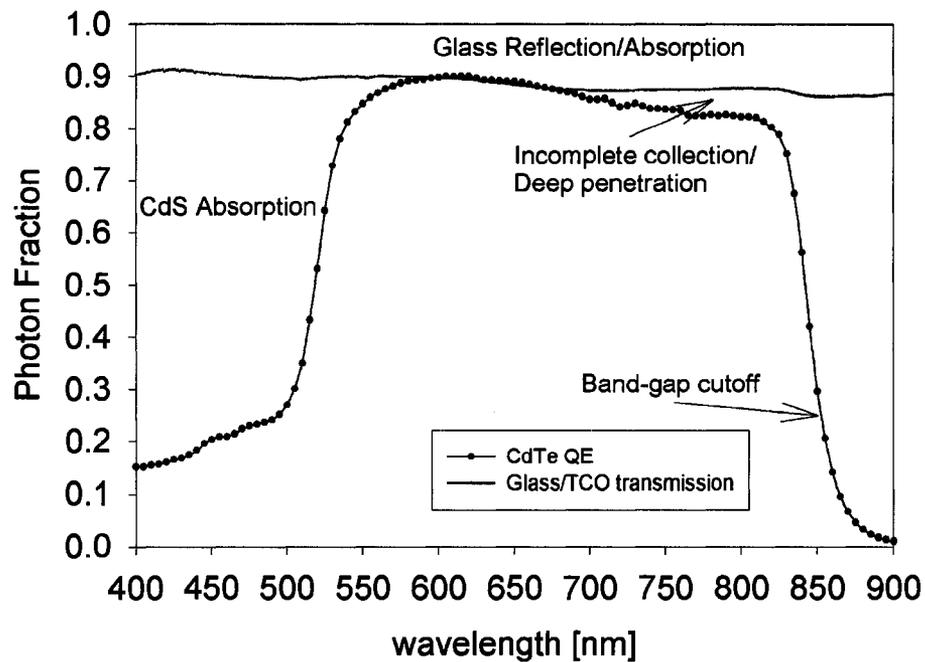
Figure 2.9: Analysis of QE data allows specific identification of current losses, and gives hints as to the mechanisms of the loss.
