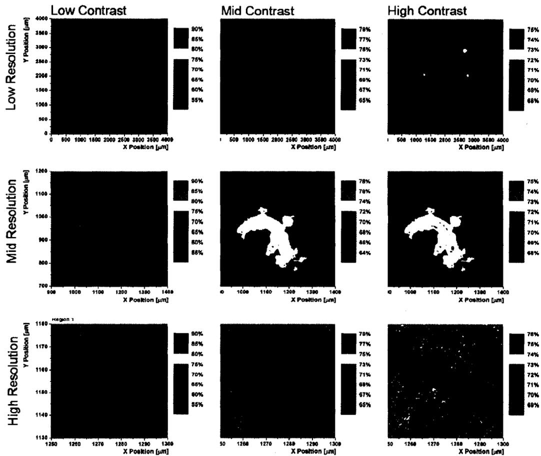
Figure 2.13: LBIC measurement results on CdTe at low, mid and high resolutions, presented with various color contrasts. The high-contrast figure emphasizes the size/shape of defects, while the low-contrast singles out the most severe areas.
