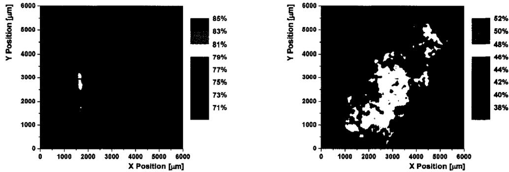
Figure 3.12: LBIC photomaps at short-circuit conditions (left) and 535 mV forward bias (right). The severe loss of uniformity in forward bias correlates to the presence of multiple diode turn-on regimes.
