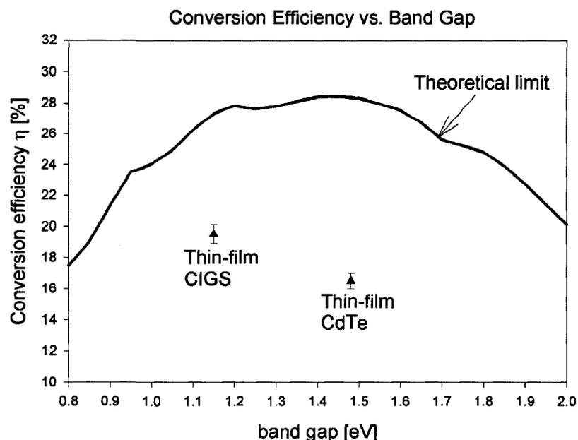
Figure 2.2: Ideal efficiency as a function of band-gap for a single junction device. The peak at around 29 % corresponds very nearly to the CdTe band-gap of 1.48 eV. The record efficiencies for thin-film CdTe and CIGS are also indicated.
