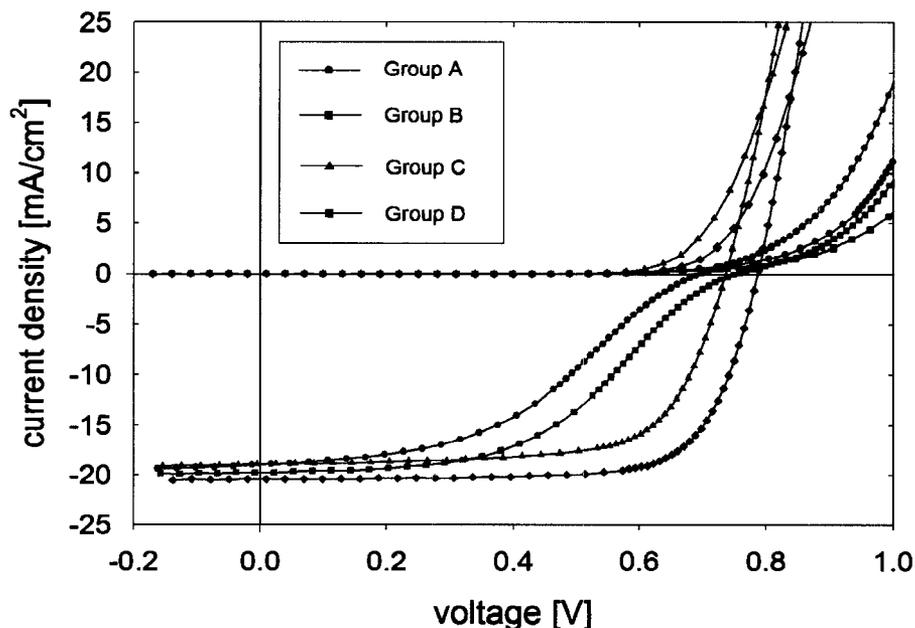
Figure 3.4: J-V curves for representative devices from each group. Adding Cu to the back contact cures the rollover behavior in an otherwise identically processed cell.
