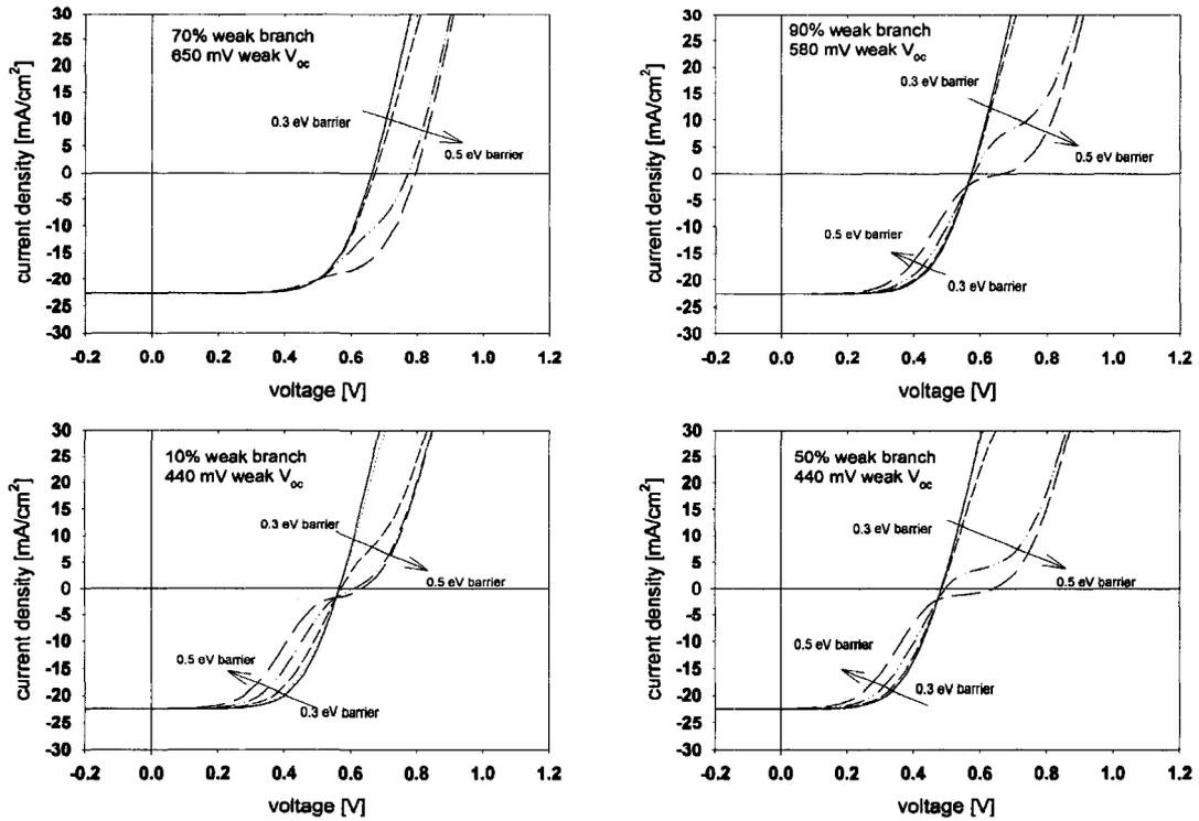
Figure 3.10: Simulation J-V with influence from back-contact based non-uniformities when they also induce reductions in main-junction performance. This combination of effects can result in rollover in the power quadrant, as observed in some experimental data.
