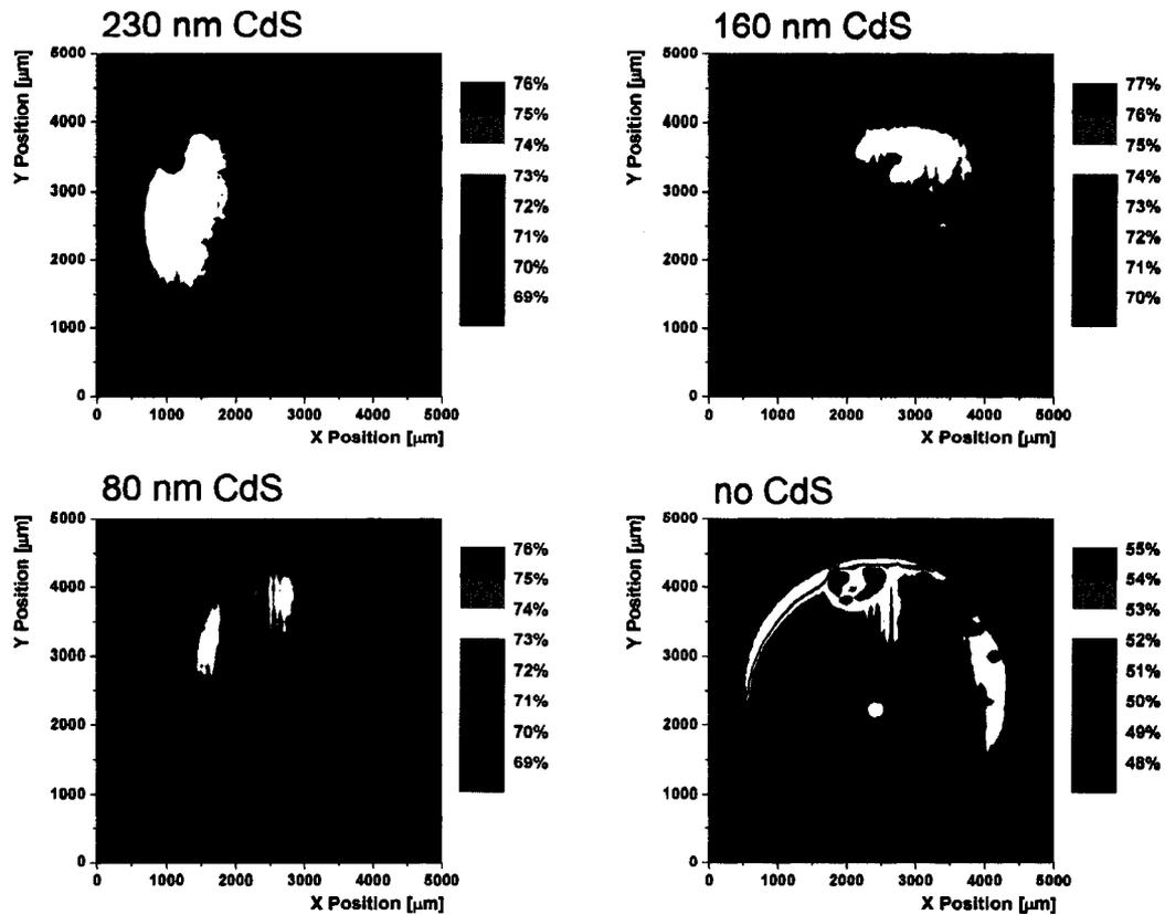
Figure 5.7: UT devices do not show strong variations on the same scales as the CSU devices. Instead edge-related effects seem to be responsible for the dominant LBIC features and may largely control the performance.
