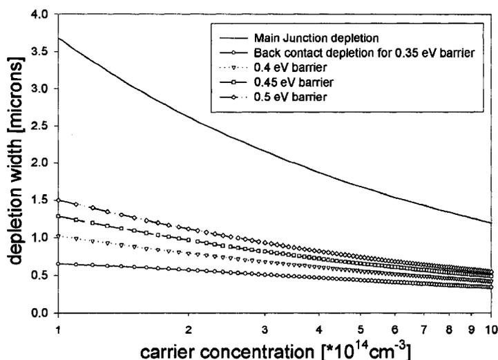
Figure 4.1: An absorber layer with thickness greater than the combined depletion widths from the front and back regions should be less susceptible to influence from non-uniformities in the back-contact
