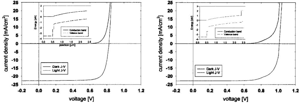
Figure 4.3: Simulated J-V curves and band-diagrams (insets) for CdTe devices with absorber thickness of  $1.8 \mu\text{m}$ ,  $p = 2 * 10^{14} \text{ cm}^{-3}$  (a and b) and a thin (100 nm) ZnTe layer (b only). The relatively low electron affinity of ZnTe establishes a positive conduction-band offset at the back of the device, reducing the number of electrons available to carry forward current.  $V_{oc}$  can be substantially increased as a result.
