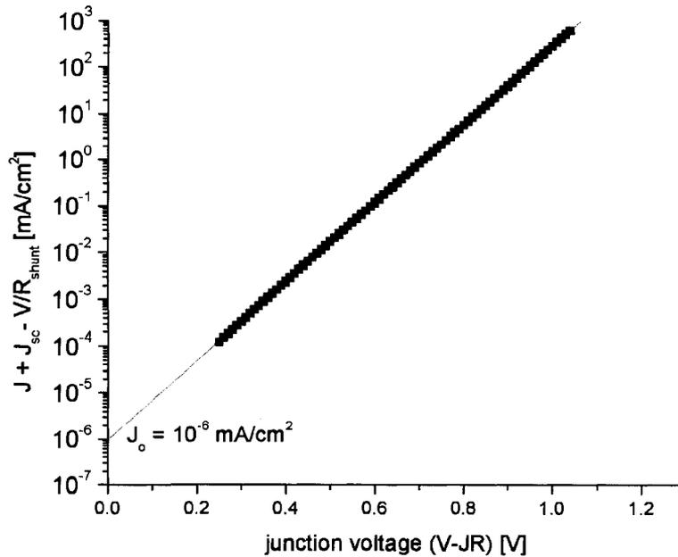
Figure 2.8: Linear extrapolation of the semi-log plot yields the diode saturation current, while the slope indicates the dominant forward current mechanism.
