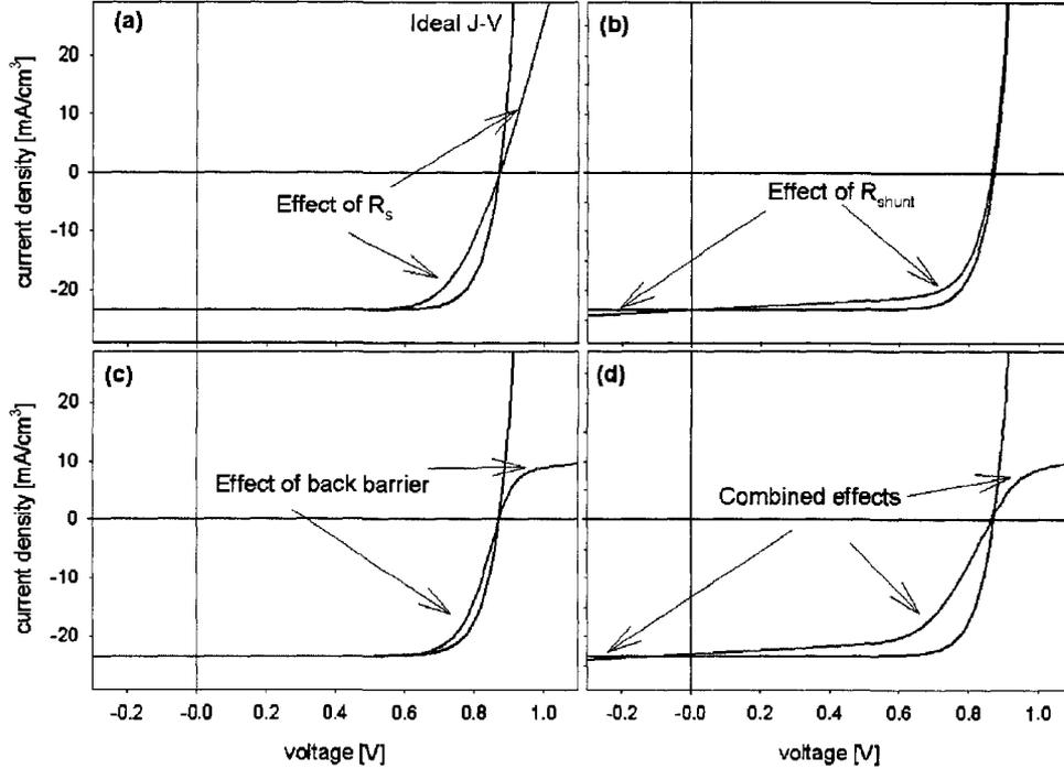
Figure 2.7: Simulation of an ideal illuminated solar cell J-V curve (black) develops linear slope components in the forward-current (a,d) and photocurrent (b,d) regimes due to series and shunt resistances. These tend to reduce the device fill-factor and efficiency, while not strongly affecting  $J_{sc}$  or  $V_{oc}$ . A back-contact Schottky barrier causes rollover in the first quadrant (c,d) and fill-factor loss.
