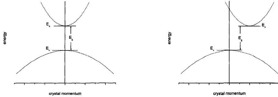
Figure 2.1: Schematic diagrams of allowed energy bands for direct (left) and indirect (right) semiconductors. The requirement for a simultaneous photon-electron-phonon interaction makes light absorption in indirect materials significantly less likely than in direct-gap semiconductors.
