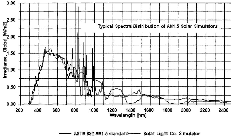
Figure 2.5: Spectrum of the solar simulator bulb compared to AM-1.5 terrestrial solar spectrum. The solar simulator gives a fairly faithful reproduction of outdoor illumination conditions, especially for  $\lambda < 840$  nm, where CdTe solar cells respond to illumination.
