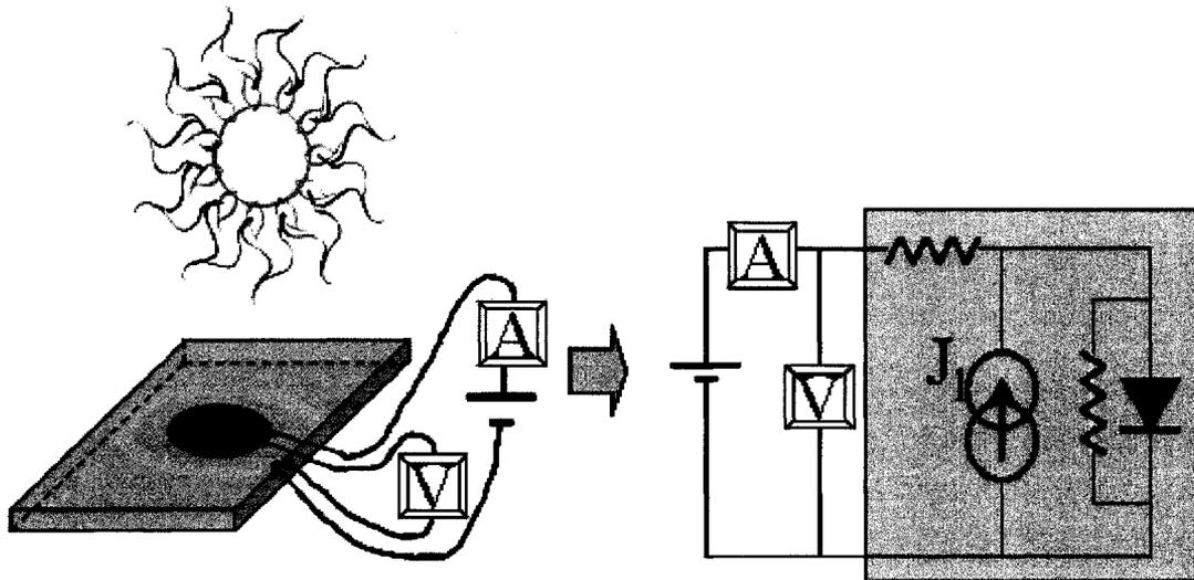
Figure 2.4: A light source of simulated solar spectrum and intensity illuminates the device in the test fixture. Independent circuits for voltage measurement and bias application/current sensing reduce inaccuracies. Analysis is aided by comparing solar cell behavior to an equivalent circuit with elements representing physical parts of the device.
