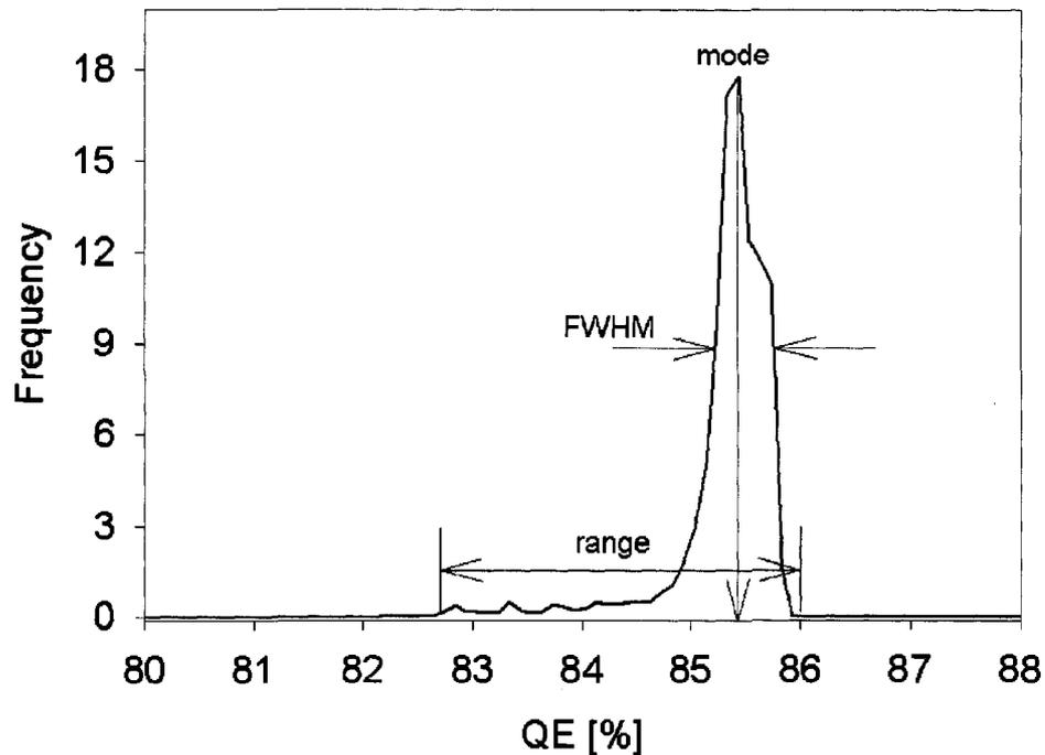
Figure 2.14: The mode, FWHM and range of the histogram distribution allow relative classification of device uniformity.
