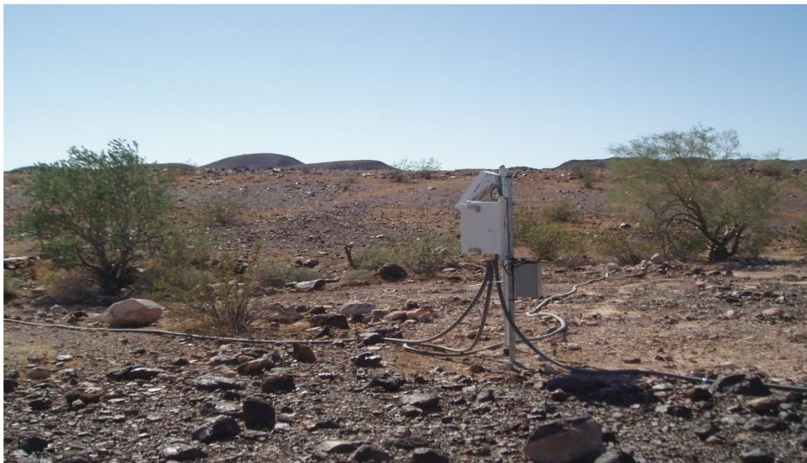
**Figure 2.4. SF3 station on middle terrace surface.** One of six soil moisture and soil temperature stations deployed in Yuma Wash. Instrumentation was emplaced beneath bare ground at 25, 50, and 100 cm (area not shown), and at 25, 50, and 100 cm beneath *P. microphylla* (photo right), and *O. tesota* (photo left).
