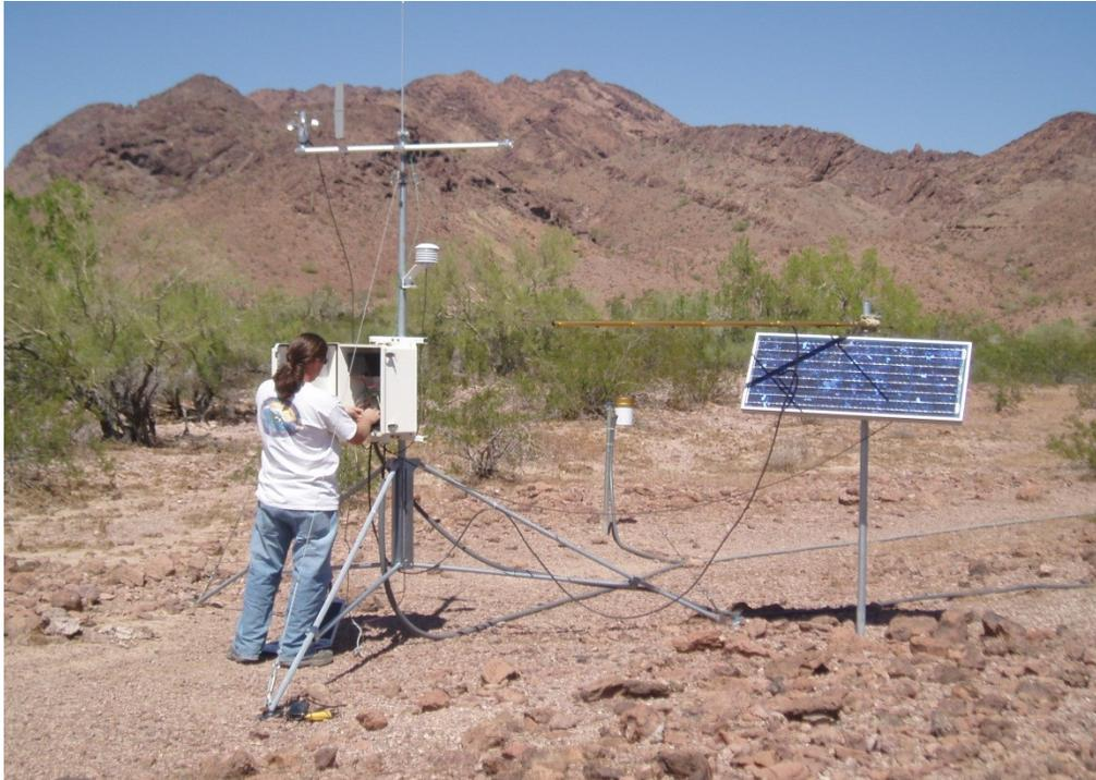
**Figure 2.1. MET3 meteorological station on the upper basin wash surface. One of six meteorological stations deployed in Yuma Wash. Tipping bucket rain gage is shown in photo center.**
