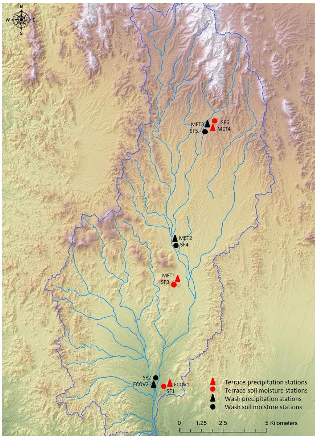
**Figure 1.3. Hydrometeorological instrumentation deployed in Yuma Wash.** ECOV and MET stations measured precipitation and soil moisture at 2.5 cm beneath bare ground. SF stations measured soil moisture at 25, 50, and 100 cm beneath bare ground, *P. microphylla* and *O. tesota*. Stations in red are located on relict alluvial terrace surfaces, and stations in black are located on alluvial wash surfaces.
