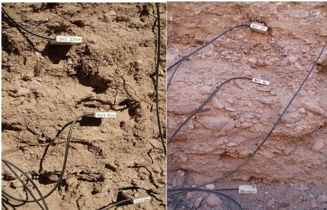
**Figure 2.6.** Soil moisture and soil temperature instrumentation installed at 25, 50, and 100cm beneath bare ground, *P. microphylla*, and *O. tesota* at six soil moisture (SF) stations in Yuma Wash.
