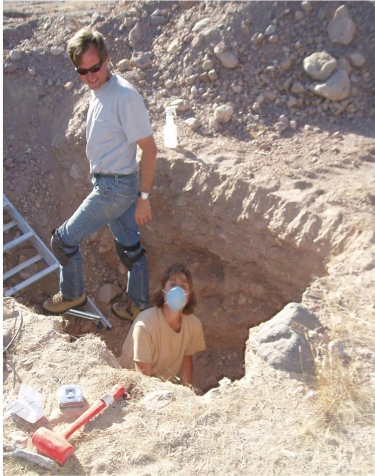
**Figure 2.7. Excavation of soil pits to one meter depth in Yuma Wash.**
