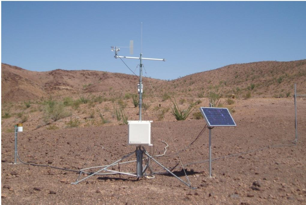
**Figure 2.2.** MET4 meteorological station on the upper basin relict terrace surface. One of six meteorological stations deployed in Yuma Wash. Tipping bucket rain gage is shown in photo left, and soil moisture and soil temperature probes at 2.5 cm are located in the subsurface of photo center.
