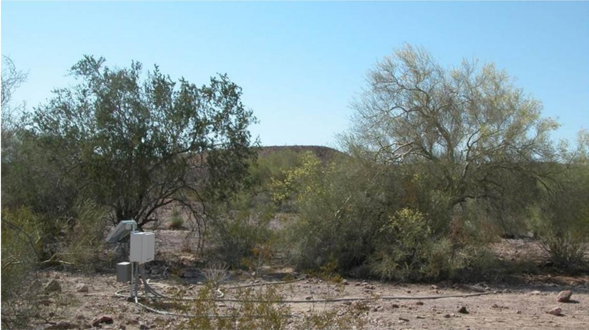
**Figure 2.3. SF5 station on upper wash surface. One of six soil moisture and soil temperature stations deployed in Yuma Wash. Instrumentation was emplaced beneath bare ground at 25, 50, and 100 cm (photo center), and at 25, 50, and 100 cm beneath *P. microphylla* (photo right), and *O. tesota* (photo left).**
