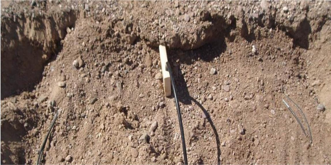
Figure 2.5. Soil moisture and soil temperature instrumentation installed at 2.5-4cm beneath bare ground at each of six meteorological (MET/ECOV) stations in Yuma Wash.
