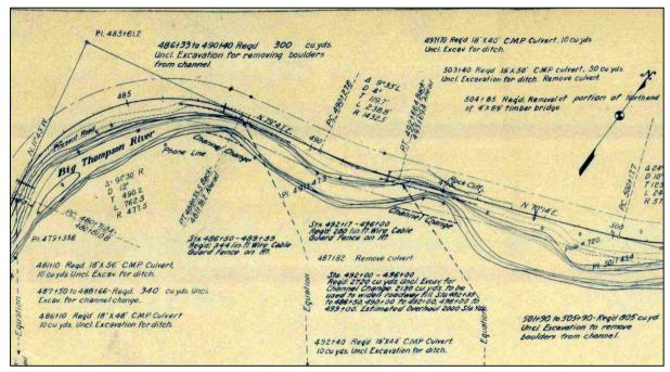
Figure 1.2. 1930s construction plans for U.S. Highway 34 between Estes Park and Drake. Note the "channel change" to Big Thompson River, twice. Courtesy of Colorado Department of Transportation.
