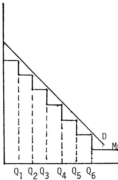
Figure 7b. Declining Block Rate Structure
