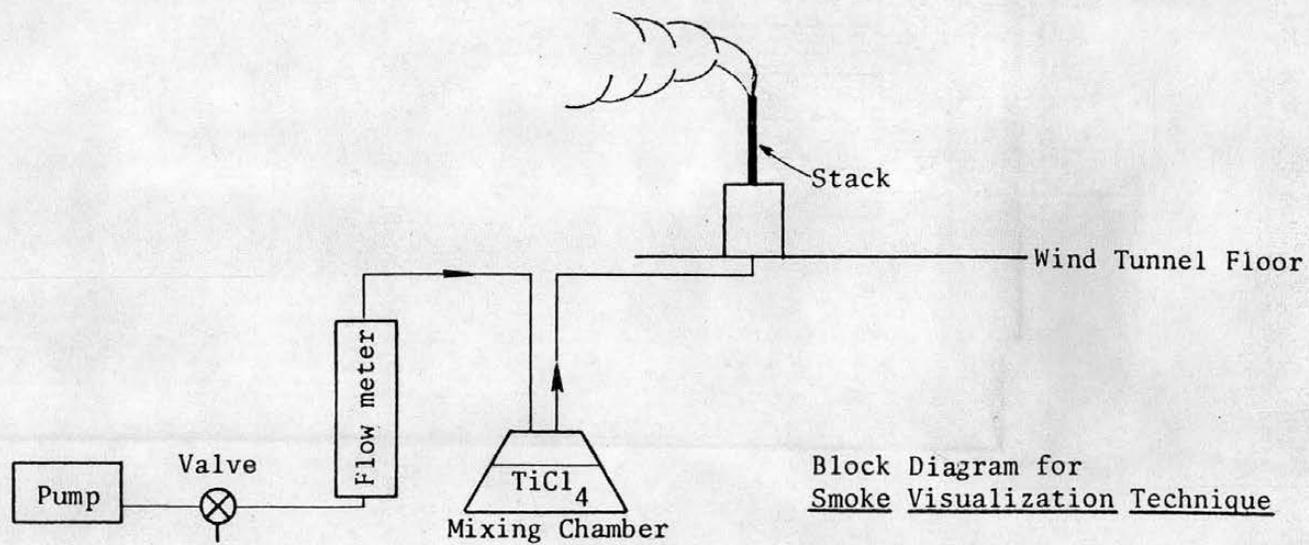
Figure 3.3-1 Schematic of plume visualization equipment.
