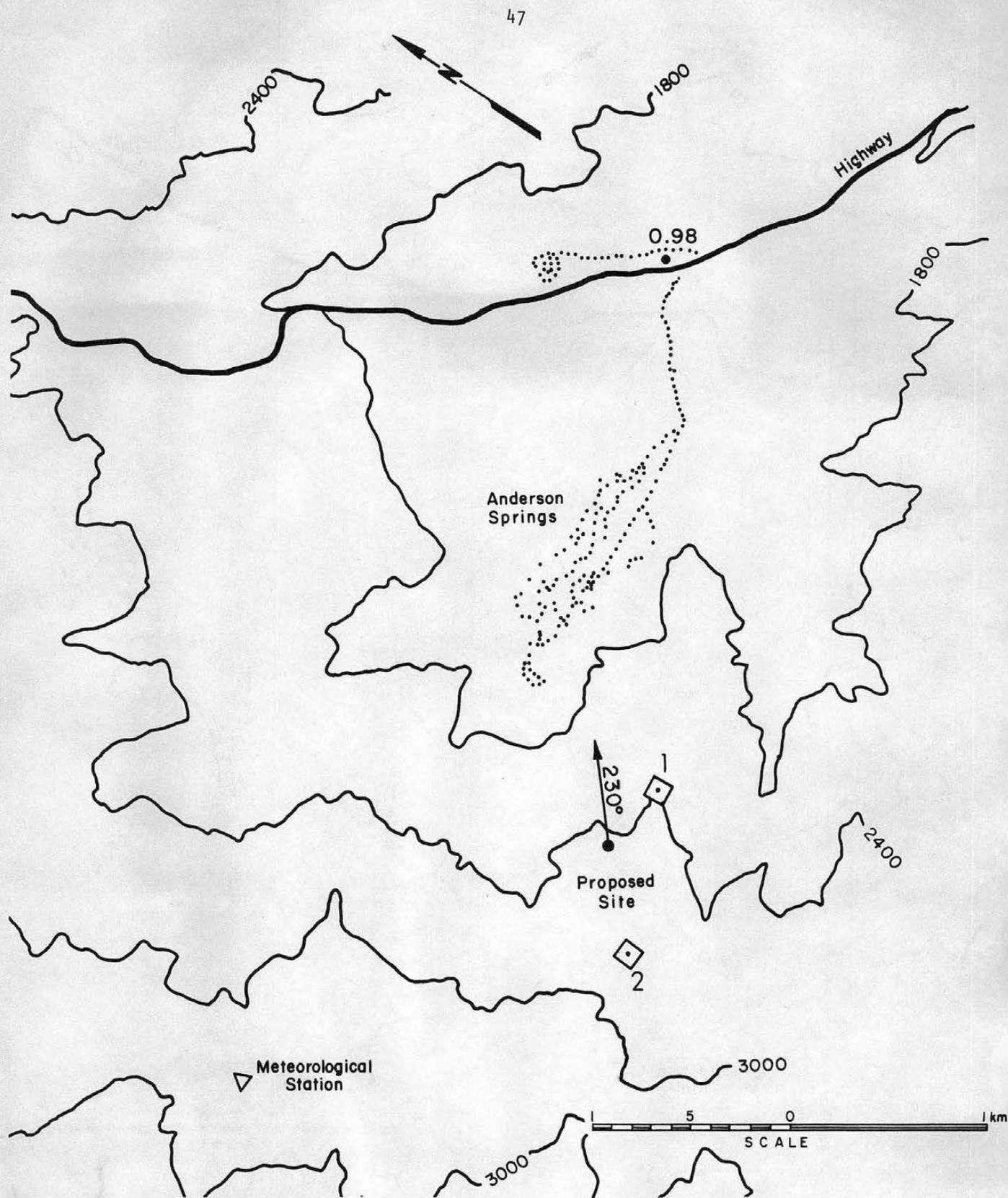
Figure 4.2-4 Isopleths of nondimensional concentration coefficient  $K$  ( $\times 10^5$ ) for Unit 16 - Site 1, wind direction  $230^\circ$ , and a wind speed of 3.2 m/s. (1 in = 610 m)
