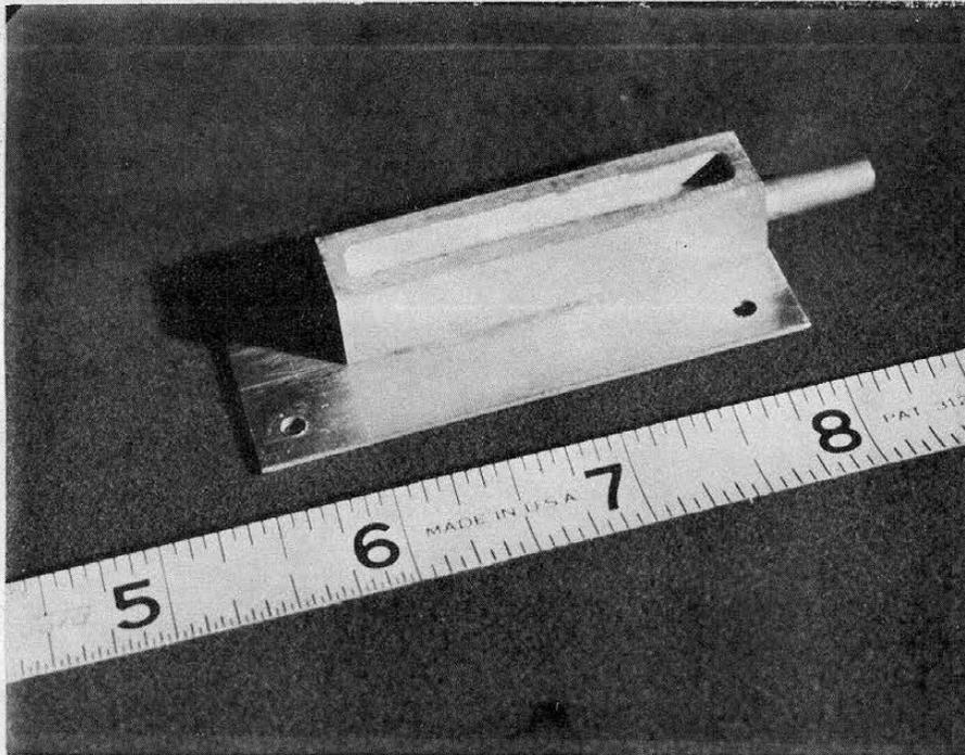
Figure 3.2-1 Photograph of Cooling Tower Model (Scale 1:1920)
