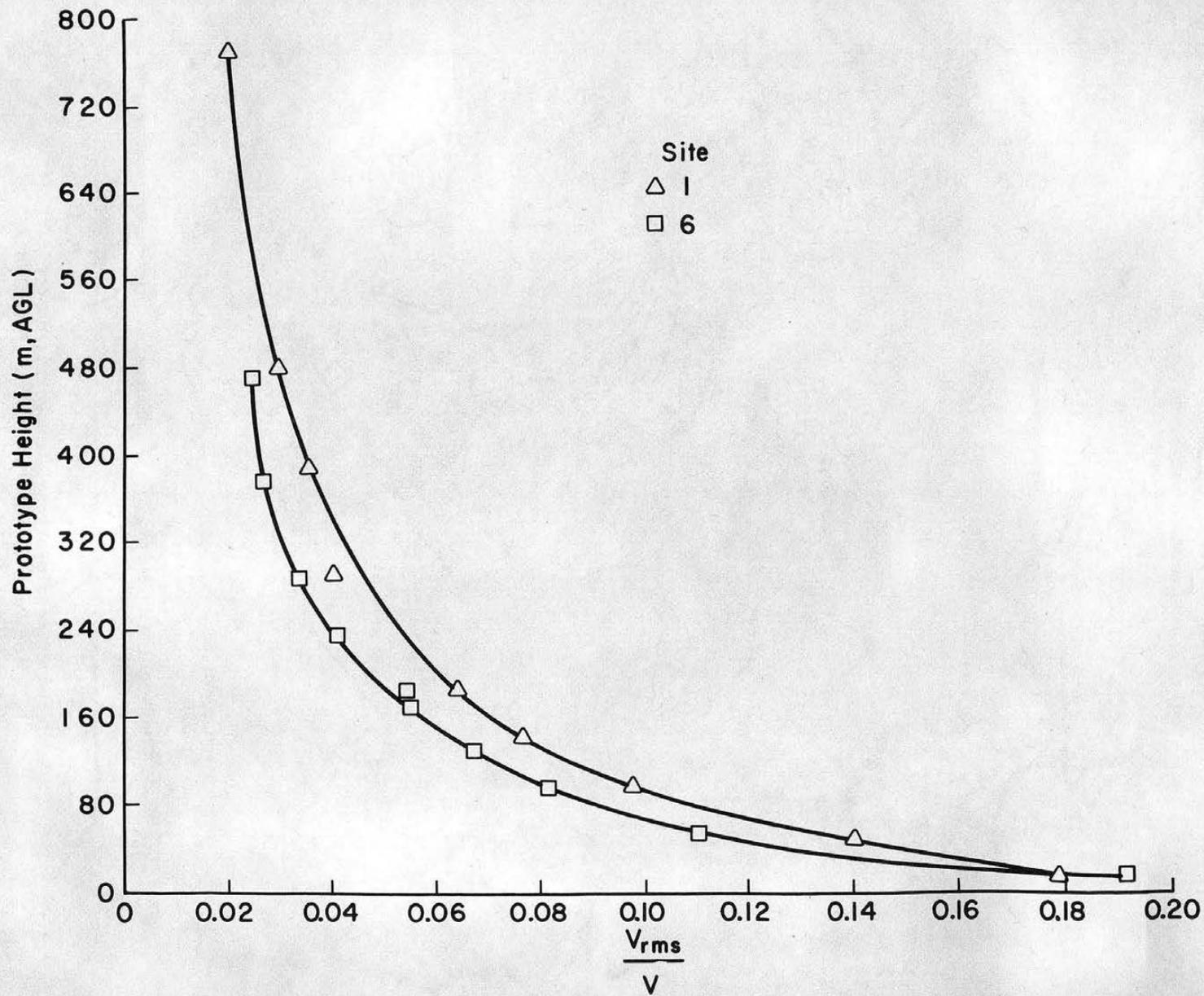
Figure 6-1 Turbulent intensity at Sites 1 and 6.
