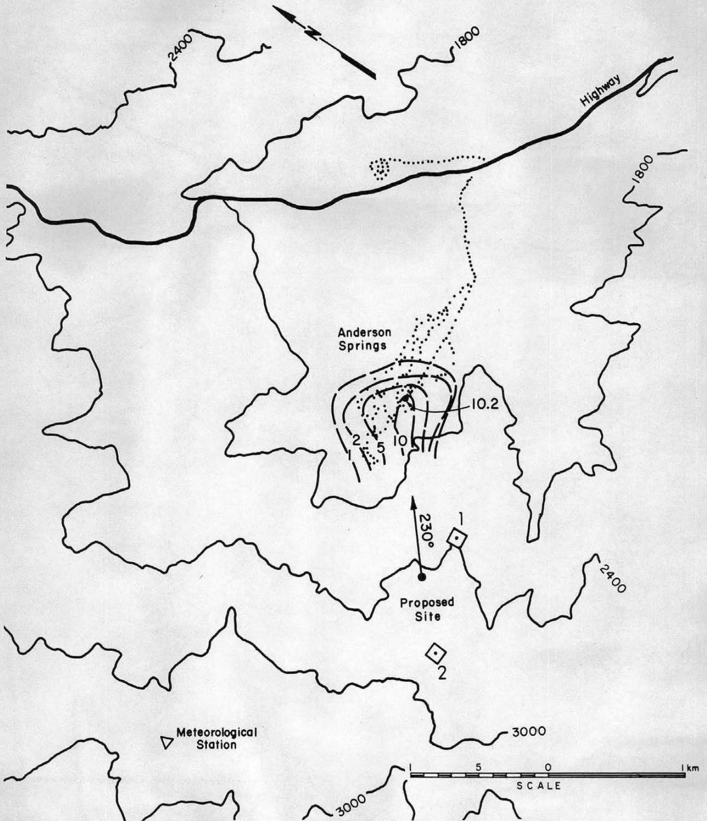
Figure 5.2-5 Isopleths of nondimensional concentration coefficient  $K$  ( $\times 10^5$ ) for Unit 16 - Site 2, wind direction  $230^\circ$ , and a wind speed of 6.5 m/s. (1 in = 610 m)
