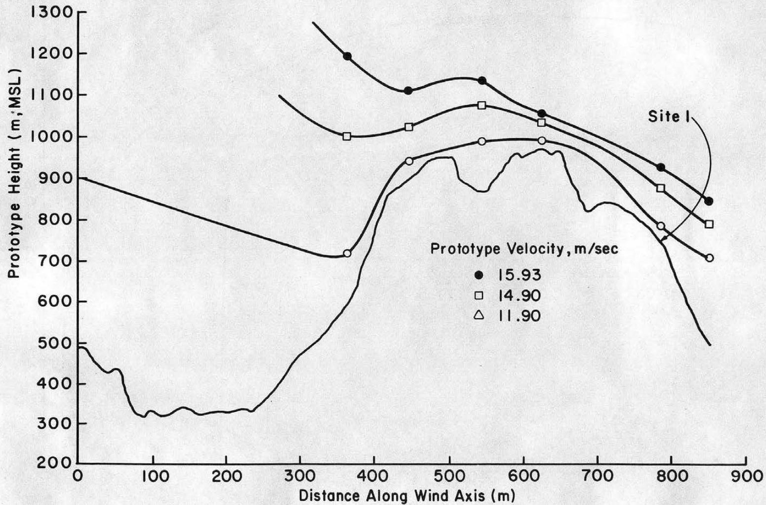
Figure 6-3 Constant velocity lines over the terrain.
