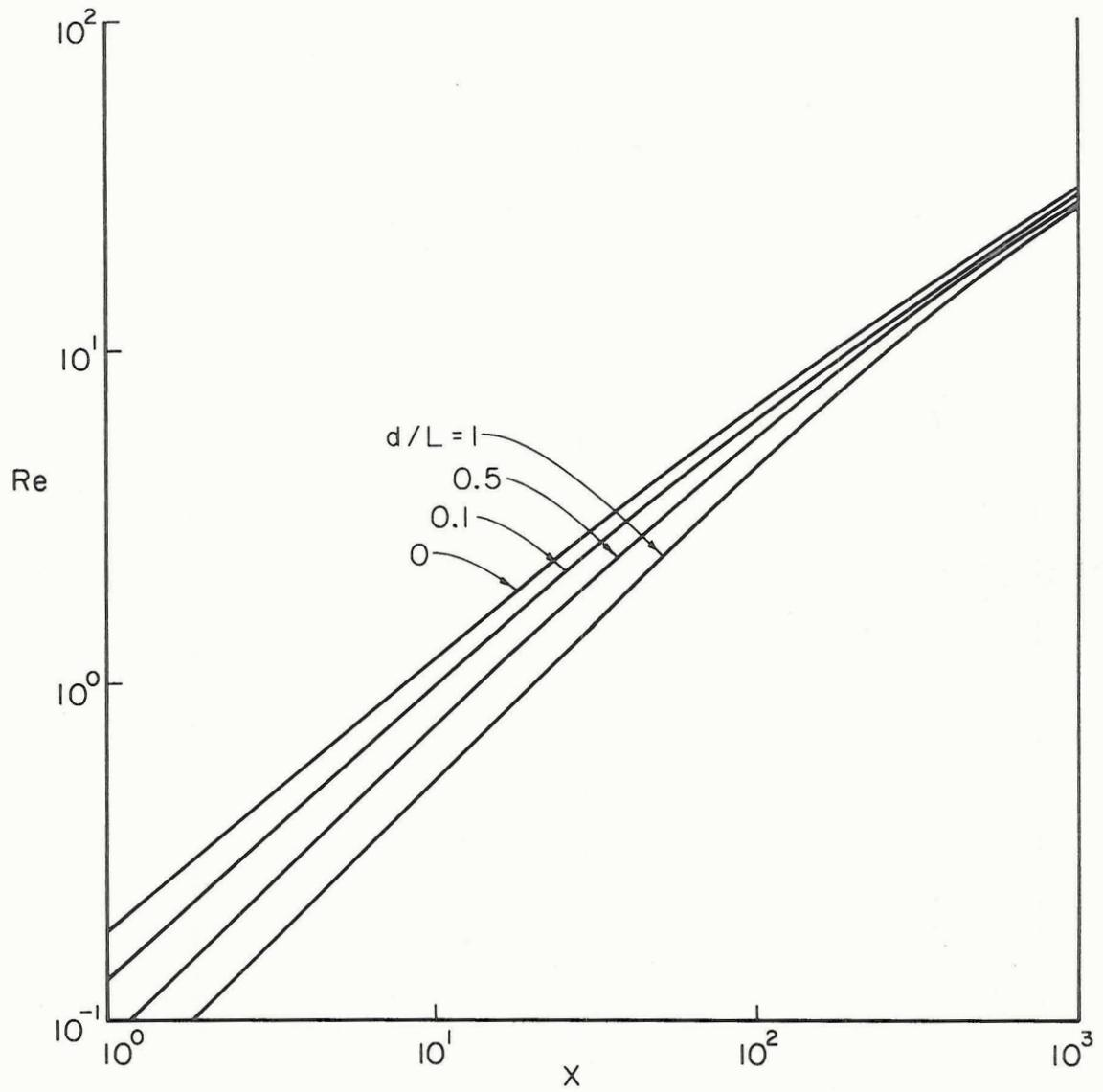
Figure 8. Relationship between X and Re for cylinders of various  $d/L$  ratio as found by Jayaweera and Cottis (1969)
