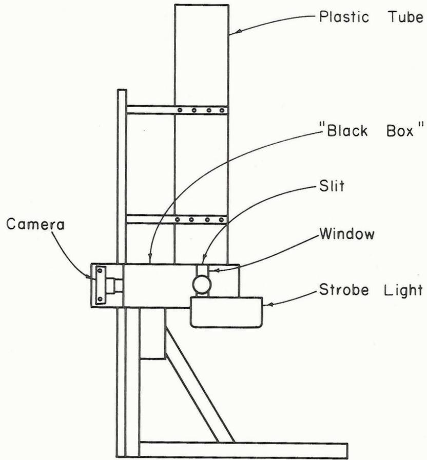
Figure 11. Physical arrangement of experimental apparatus
