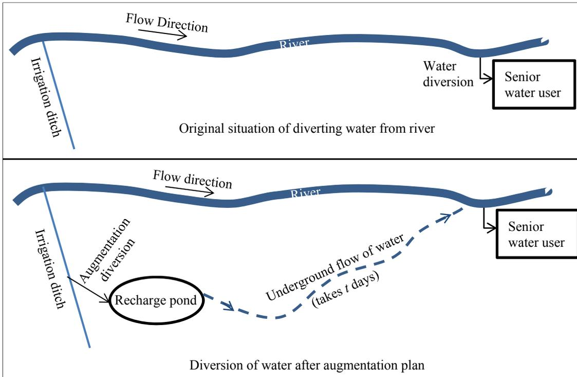
**Figure 2 Schematic presentation of function of a recharge pond**
