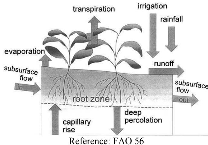
**Figure 20 Components of soil root zone water balance**
