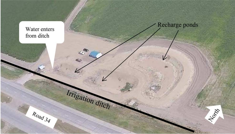
**Figure 3 Recharge ponds on Subsurface Irrigation Efficiency Project, in Kersey, CO**
