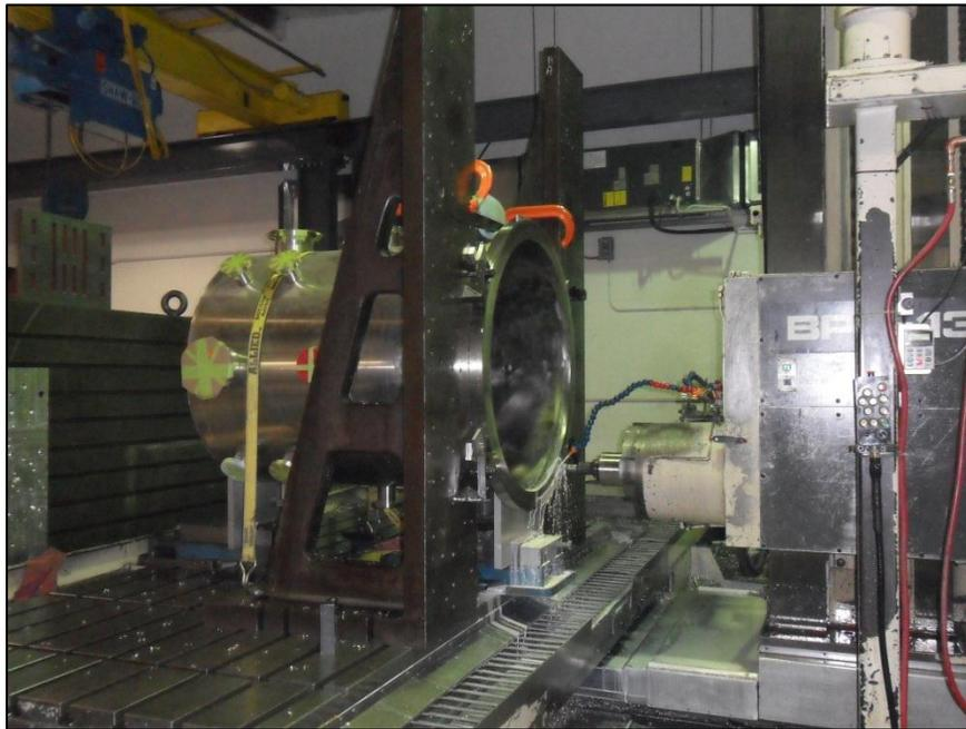
**Figure 2.3. Groove for O-ring being machined into the door flange.**
