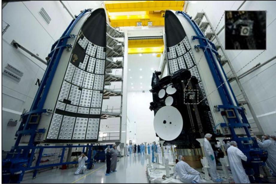
**Figure 1.3. BPT-4000 mounted on an AEHF satellite during launch preparation [22].**
