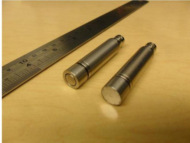
**Figure 3.5. Faraday probes used for plasma measurements.**
