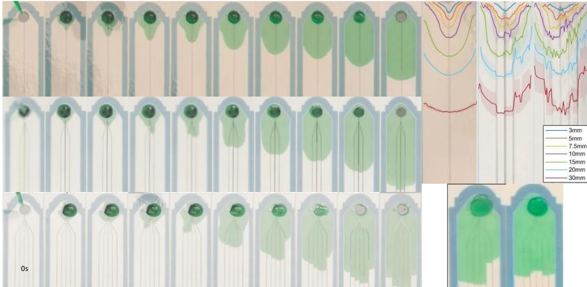
Figure 14(S1) – Timelapse displaying how liquid flows in channels. Left- 15mm channel with single, 3-branch and 5-branch grooves. Top right – Liquid flow profile at indicated distances from the inlet with standard deviation cloud (n=4). 3mm marks the branch point. Bottom right – Variability of channels increases with additional branches.
