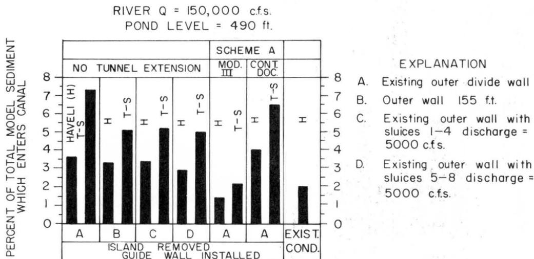
FIG. 20 COMPARATIVE RESULTS OF CHANGES IN EXISTING STRUCTURE WITH NO TUNNEL EXTENSION, WITH SCHEME A CONTR. DOC. AND WITH MODIFICATION III
