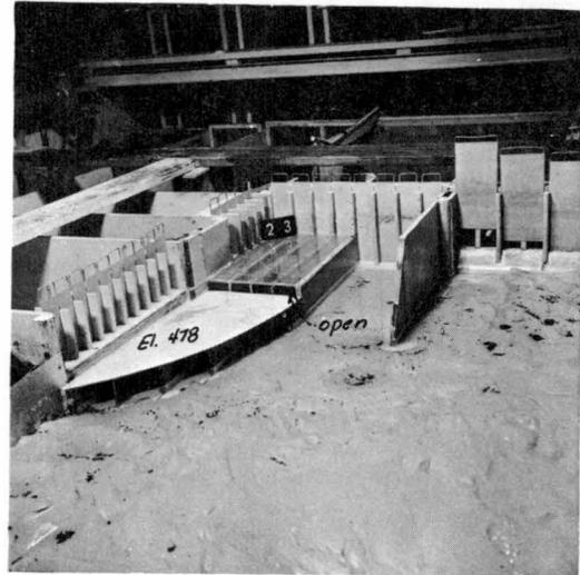
Fig. 13. Scheme A Modification II. Tunnel extension roof raised to elevation 478.
