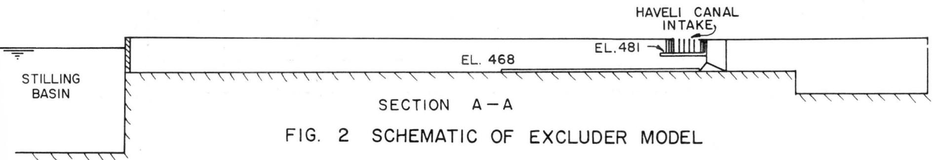
FIG. 2 SCHEMATIC OF EXCLUDER MODEL
