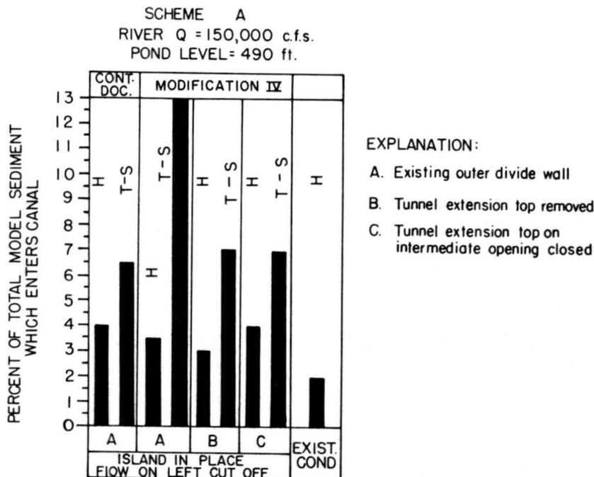
FIG. 17 SCHEME A MODIFICATION IV. T-S CANAL SET BACK 50 ft.
