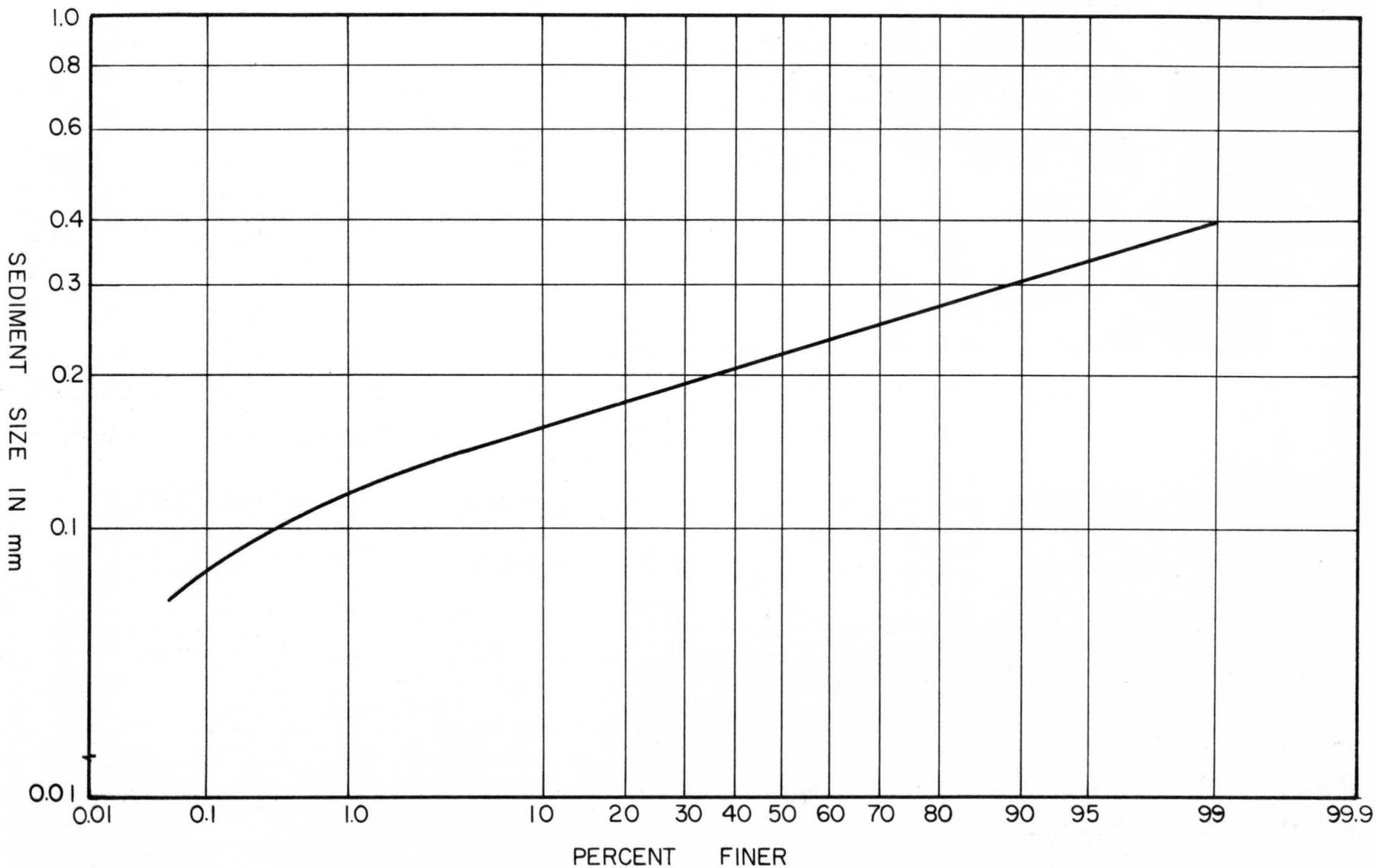
FIG. 3 SEDIMENT EXCLUDER MODEL SEDIMENT SIZE DISTRIBUTION CURVE
