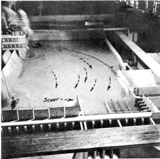
Fig. 21. Intermediate wall removed. No sluice tunnel extension.
