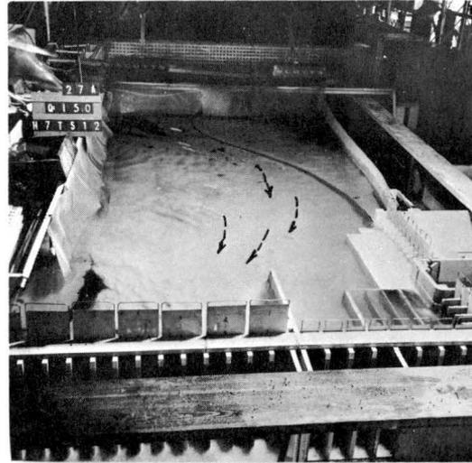
Fig. 23. Pattern of flow with existing outer divide wall and no sluices operating.
