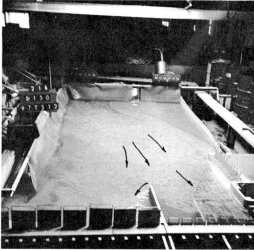
Fig. 9. Surface flow pattern of Scheme A (Cont. Doc.) with 4' drop curtain and existing outer wall.
