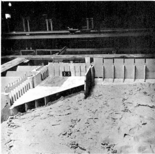
Fig. 18. Sluice tunnels extended to include left pocket area.
