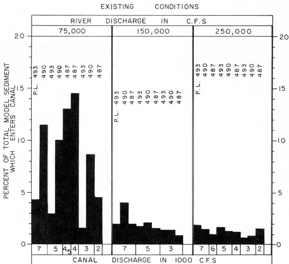
FIG. 5 PERCENT OF TOTAL SEDIMENT INTRODUCED IN THE MODEL ENTERING HAVELI CANAL
