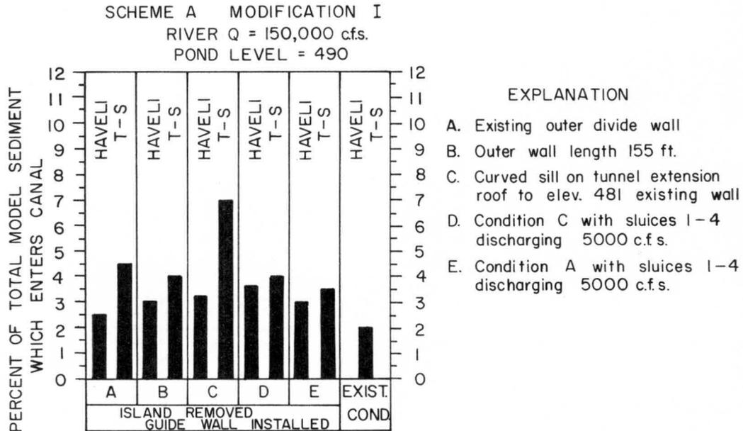
FIG. 12 COMPARATIVE RESULTS OF SCHEME A MODIFICATION I. REDUCTION OF SEDIMENT IN CANALS COMPARED TO FIG. 11
