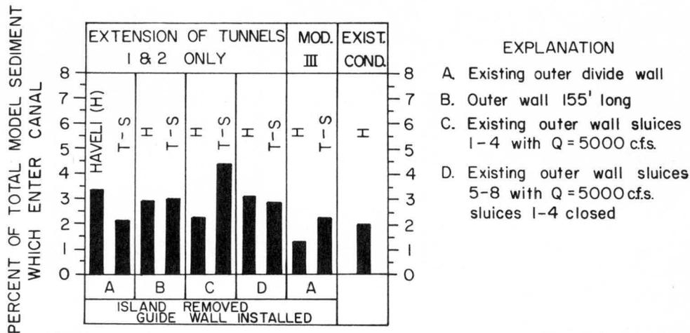
Fig. 24 COMPARISON OF EXTENSION OF TUNNELS I AND 2 ONLY WITH SCHEME A MODIFICATION III
