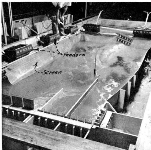
Fig. 4. View of sediment feeders used in model and screen in front of the feeders to ensure submergence of plastic particles.
