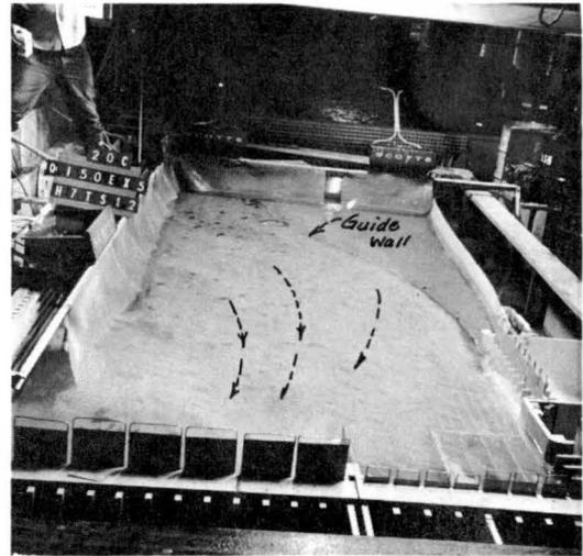
Fig. 7. Left guide wall installed in accordance with Pakistan model results. Arrows show pattern of bed-load movement.
