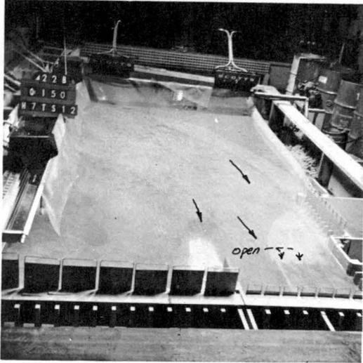
Fig. 11. Scheme A Modification I during test with shortened outer divide wall. The difference in tunnel top elevation between the extension and existing sluice tunnels can be seen.
