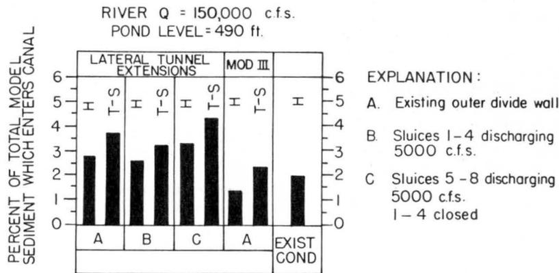
FIG. 19 RESULTS OF TUNNEL EXTENSIONS LATERALLY TO INCLUDE SLUICES 5 TO 8
