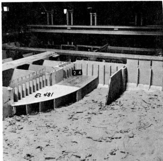
Fig. 14. Scheme A Modification III. Tunnel extension roof raised to elevation 481.
