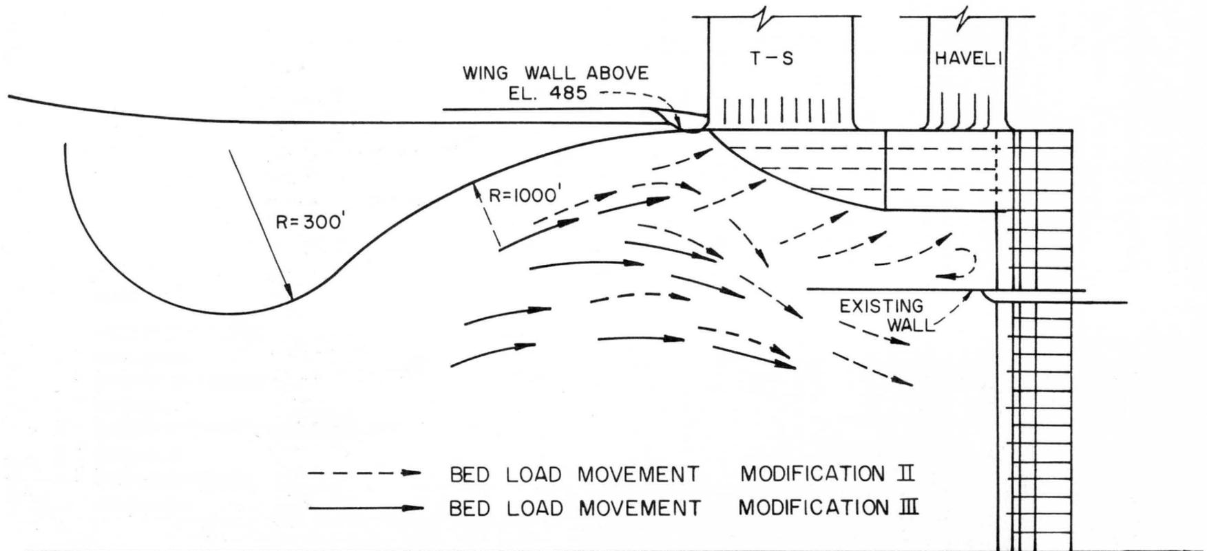
FIG. 16 COMPARATIVE BED LOAD MOVEMENTS WITH MODIFICATIONS II AND III.
