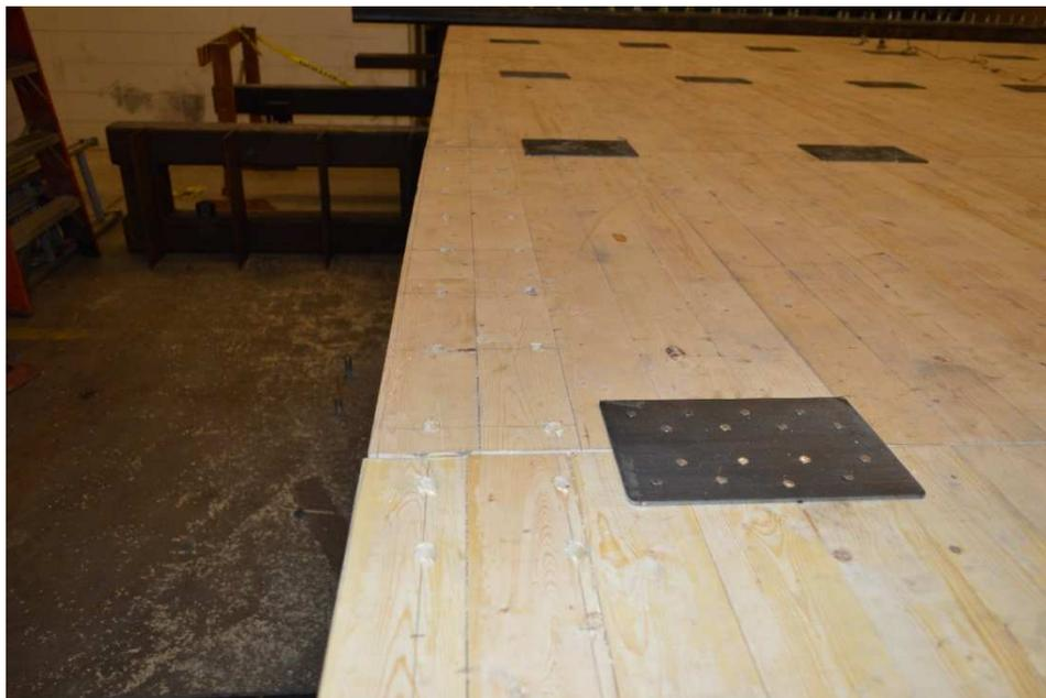
Figure 2.5 SDS Screws in a line connecting CLT to Chord Members
