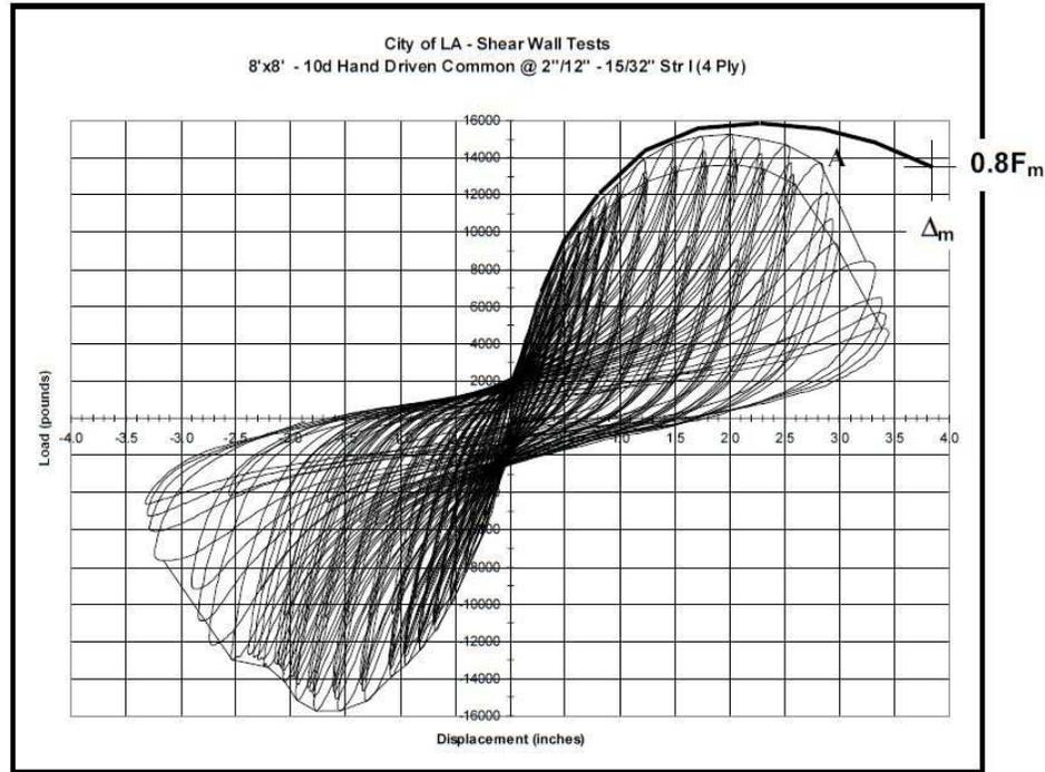
Figure 3.2  $\Delta_m$  (Monotonic Deformation Capacity) and its Relation to a Cyclic Test
