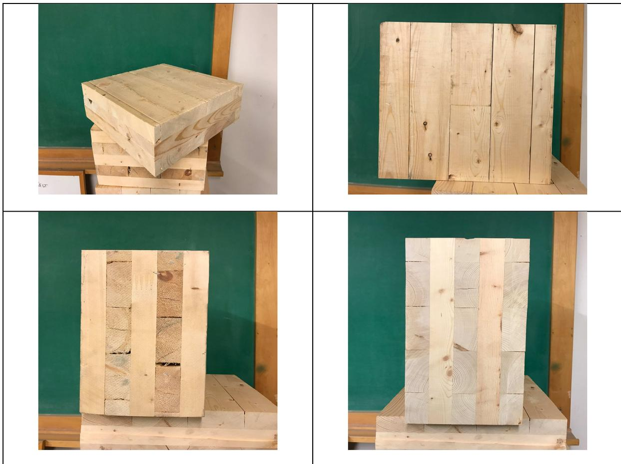
Figure 1.3 CLT Panels
