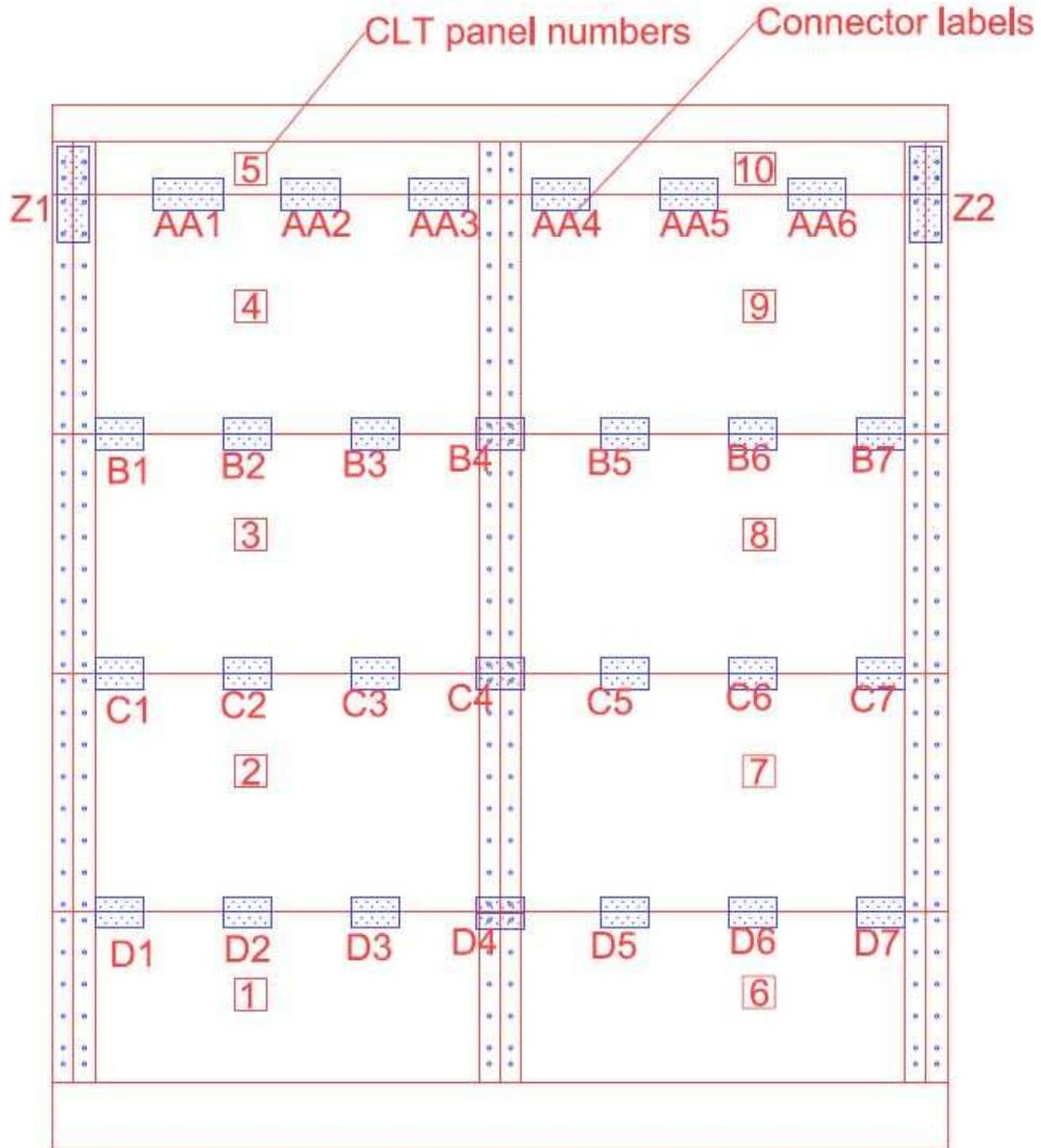
Figure 2.6 Connector Layout (Plan View)
