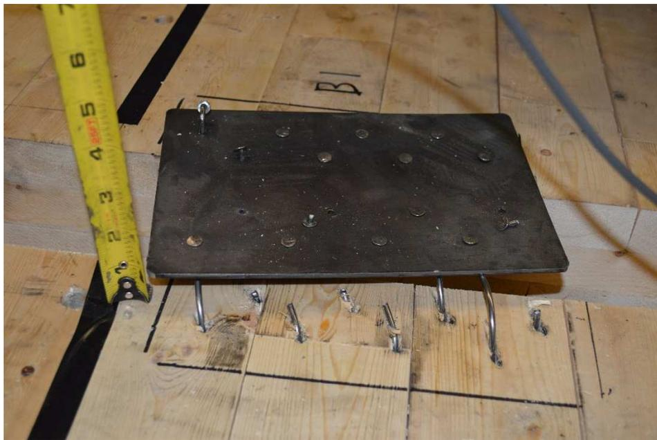
Figure 4.7 Connector B1 after the test (Side View)
