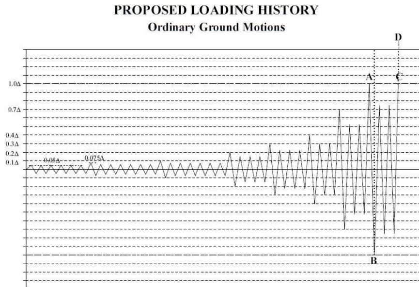
Figure 3.1 Loading History for Basic Cyclic Load Test
