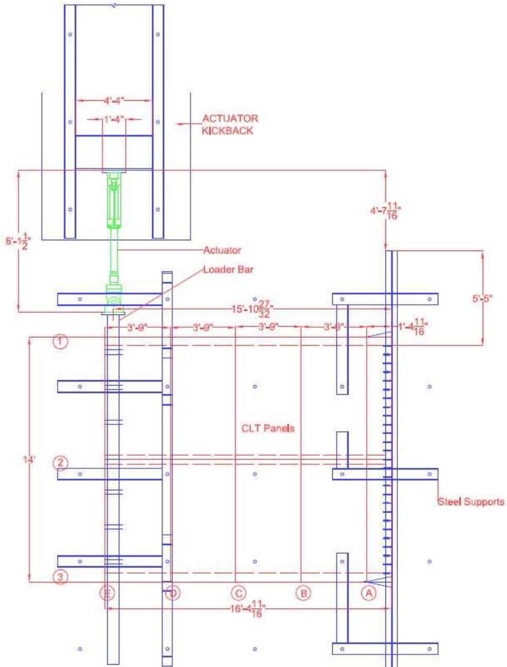
Figure 2.2 CLT Diaphragm Test Setup Plan View
