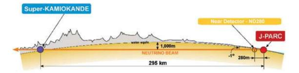
Figure 4: A schematic of the T2K experiment. The path of the neutrino beam is shown as it travels from the JPARC facility to Super-Kamiokande through ND280 and 295 km of rock.
