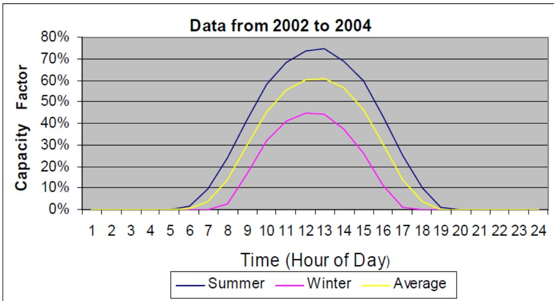
**Figure 14: MAB Solar Potential based on Time of Day [39]**
