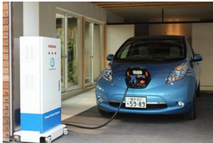
**Figure 11: Nissan Power Control System (6 kW through CHAdeMO compliant connector)**
