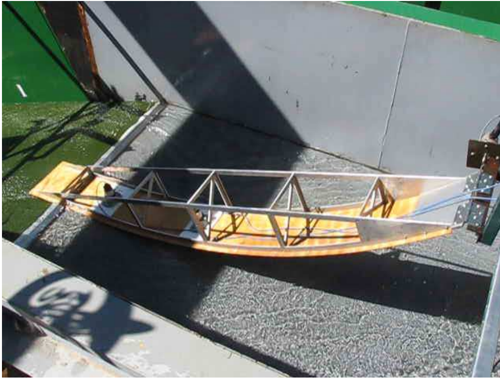
Figure 3-7. Surfboard for measuring flow thickness.
