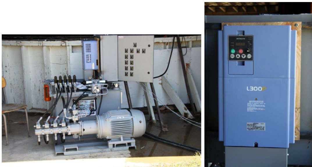
Figure 3-6. The hydraulic power unit (left) with variable speed drive (right).
