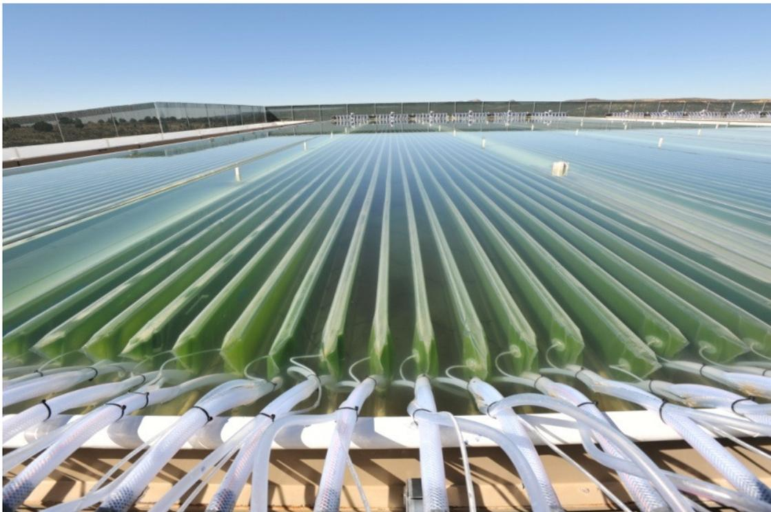
**Figure 22. Image of cultivation system modeled courtesy of Solix Biosystems. Photobioreactors are structurally and thermally supported in a water basin.**
